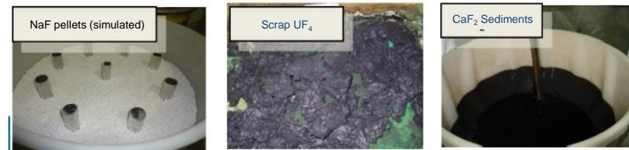
Figure Simulated diverse uranium waste used in the test using the FNDI method
