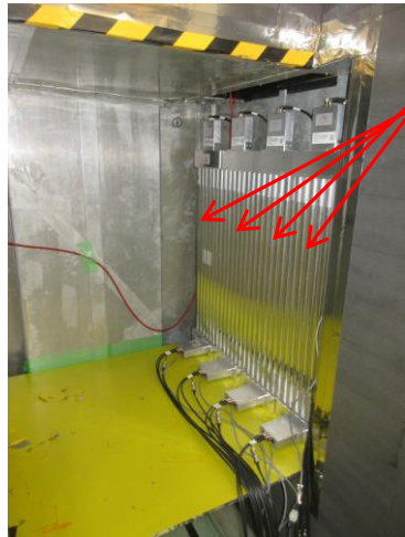
B-10 straw detector (Total 4 units: No.1, No.2, No.3, No.4 from the left 1 unit consists of 7 numbers of B-10 straw detectors lined up in a row)
