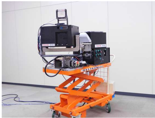
Contamination measurement by using \alpha camera
