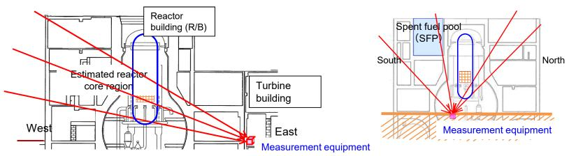
Illustration of measuring muons passing through the reactor building (horizontal cross section)
