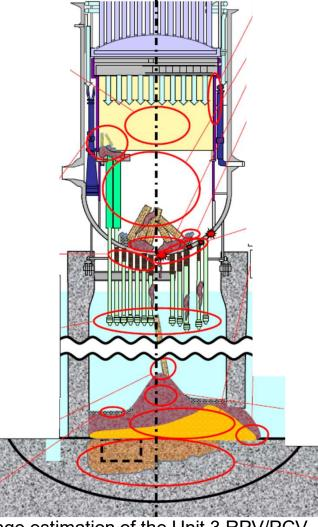
Damage estimation of the Unit 3 RPV/PCV (From TEPCO HP)
