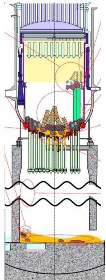
Damage estimation of the Unit 2 RPV/PCV (From TEPCO HP)
