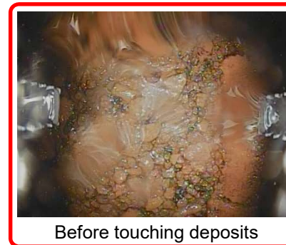
Photo: Touching pebble-like deposits by tool at the Unit 2 PCV bottom
