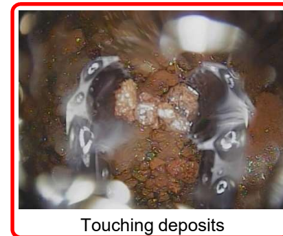
Photo: Touching pebble-like deposits by tool at the Unit 2 PCV bottom
