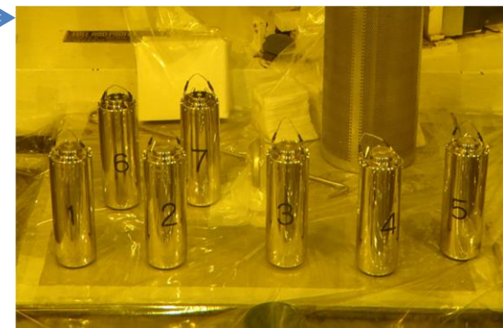
Removing the canister from the inner container for the transport cask (7 canisters)
