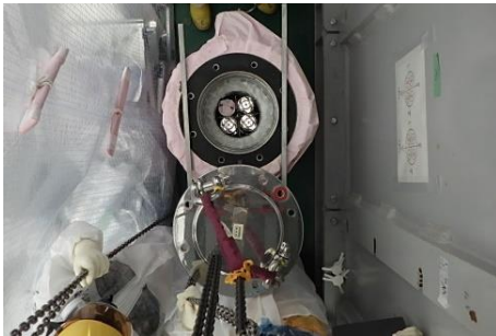
Storing the canister into the transport cask (Image captured facing down from the WS second floor)
