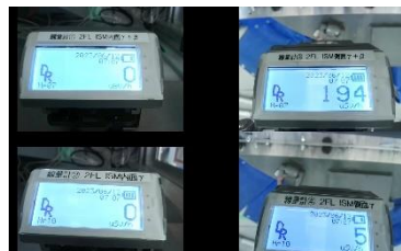
Figure 1 Illustration of dosimeter monitor displays (1 monitor displays data from 4 dosimeters simultaneously)
