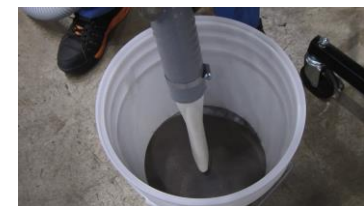
Figure 5 Lead particles suction recovery test
