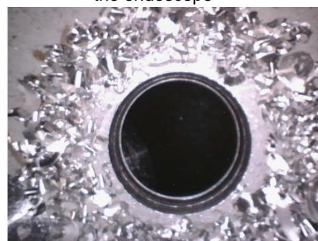
After performing the penetration for making the \Phi 50 opening
