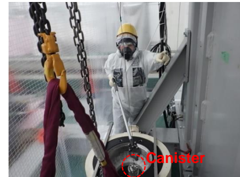
Minor adjustments with the grabber tool for storing the canister at the specified location in the inner container of the transport cask
