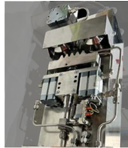
Dual arm type manipulator side terminal box being assembled
