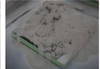
Figure 6 Use of liquid to solidified type of absorber on fuel debris with large unevenness
