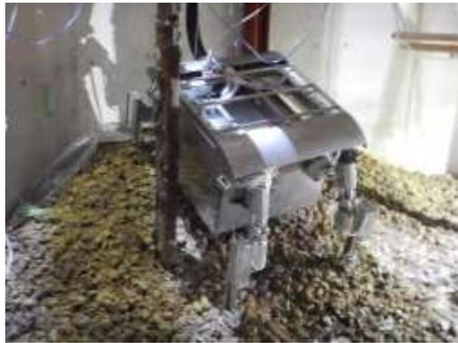
Loading and moving of neutron detector unit (simulated) with the heavy weight object transfer equipment (Side retrieval PLAN-B method)
