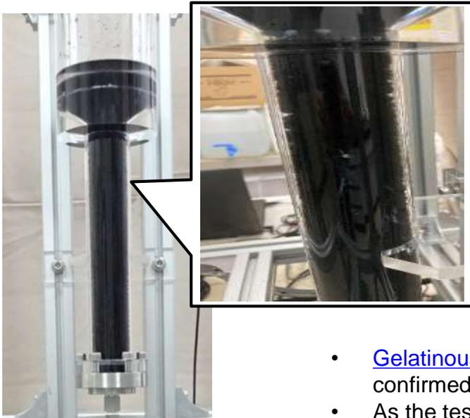
Since coagulant components were large, cakes with high viscosity and high moisture content were formed
