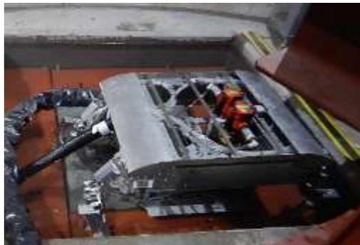
Loading and moving of crushing and suction equipment with the heavy weight object transfer equipment (Side retrieval PLAN-B method)
