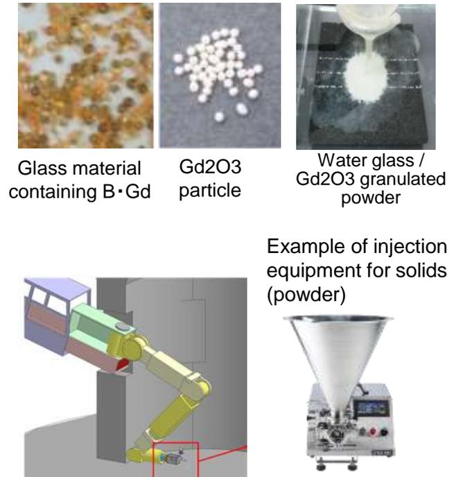
Figure 1 Drawing of injection of absorbers to fuel debris
