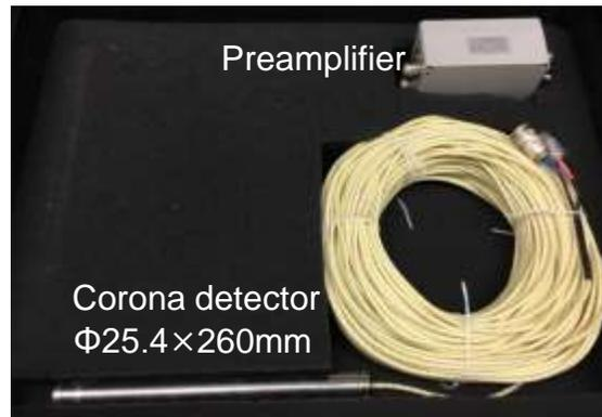
Figure 1 Appearance of B-10 corona discharge type detector
