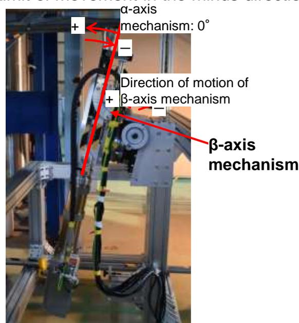
Direction of motion of  $\alpha$ -axis and  $\beta$ -axis
