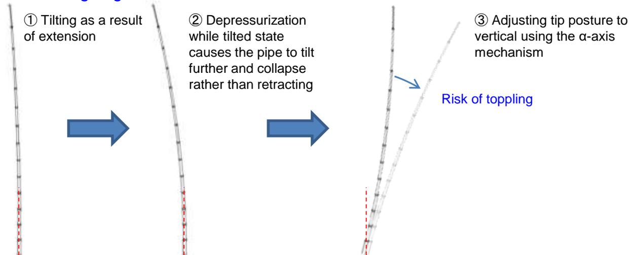
Diagram of telescopic pipe collapsing after depressurization
