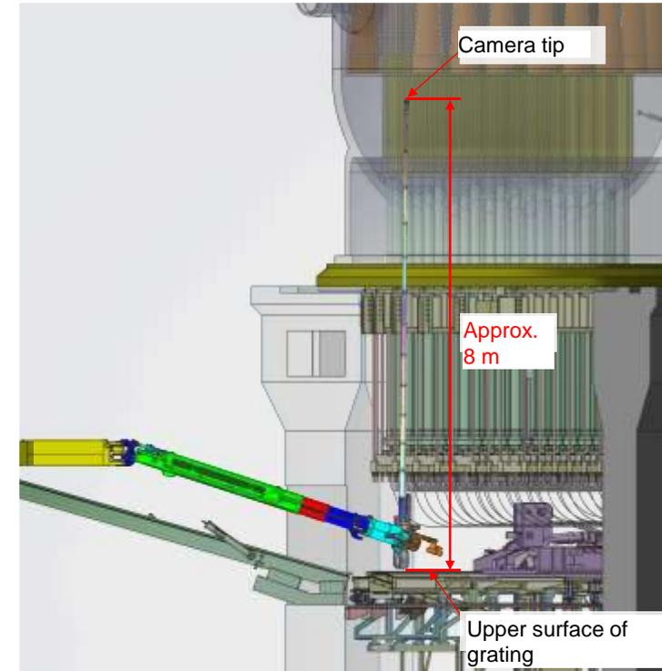
Picture of access using telescopic pipe
