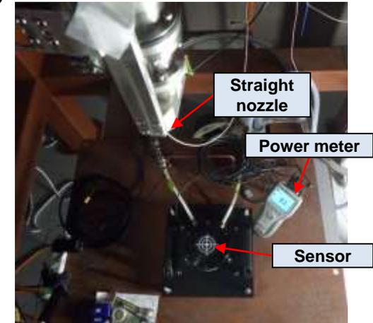
Laser output measurement setup
