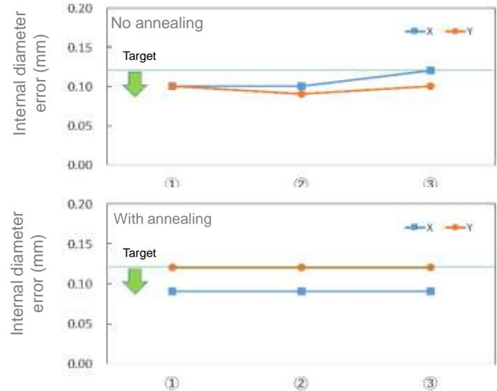
Machining results after annealing treatment
