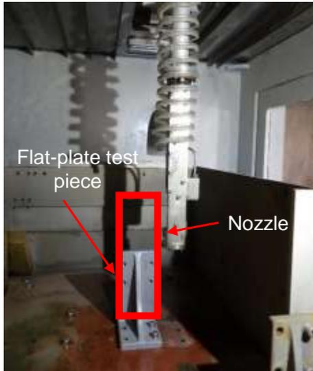
Setup for simple evaluation test of cutting performance
