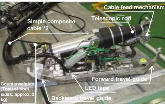
External view of FY2022 prototype (wired)
