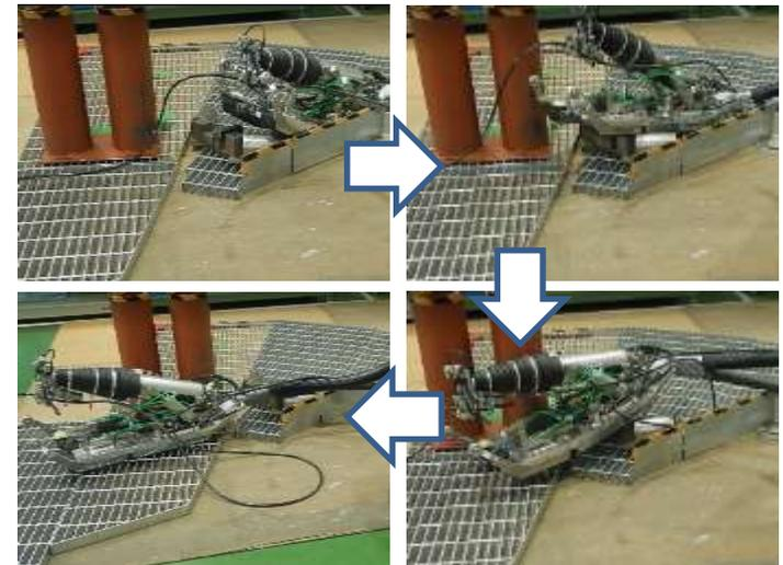
**Traversing mock left-behind B1 investigation equipment (wired specification)**
