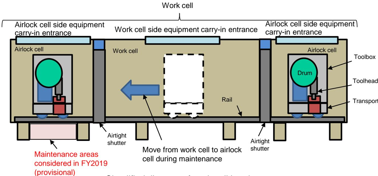
Simplified diagram of work cell interior
