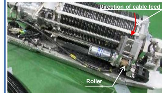
Improved cable feed mechanism (FY2022)
