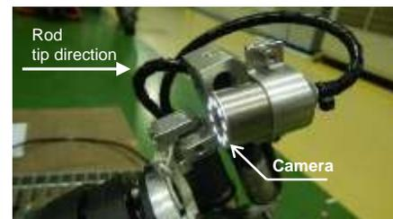
Revision of the pan tilt range for the camera on the tip of the wired drone rod \*3
