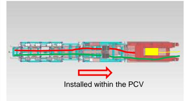
⑮ Installation of the cable drum transfer cart
