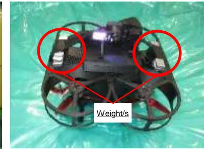
**Drones loaded with weights (left: wired, right: wireless)**
