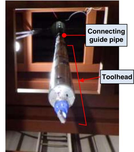
Connecting guide pipe and toolhead
