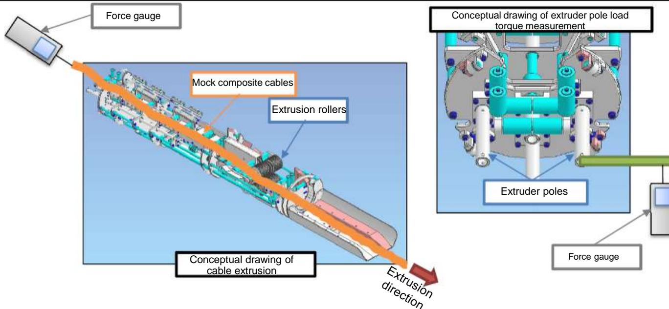
**Conceptual drawing of the test**
