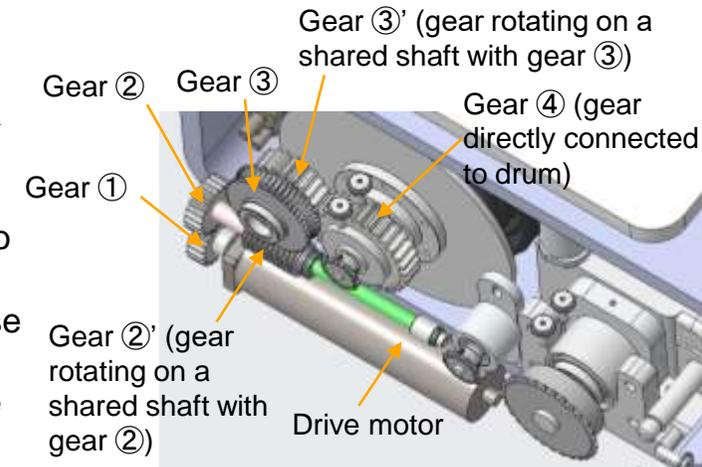
Mechanism for transmission of torque from motor to cable winding drum
