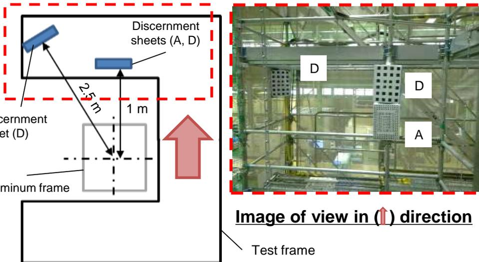
Test frame (ground plan)
