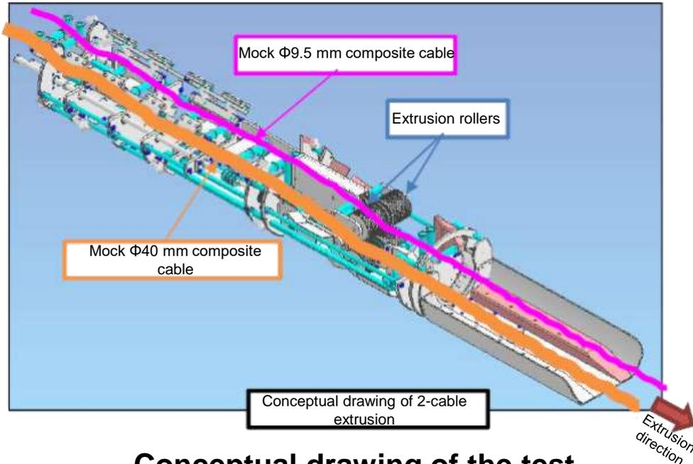
Conceptual drawing of the test
