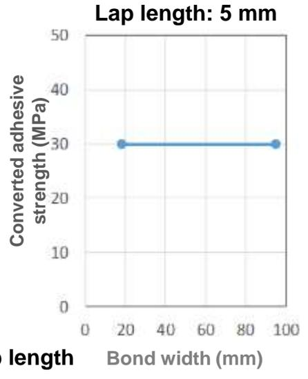
Test with constant lap length and varying bond width
