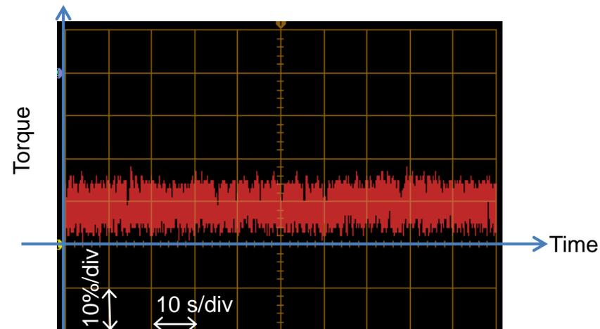
Variation in drum drive torque under no load conditions (After improvement)
