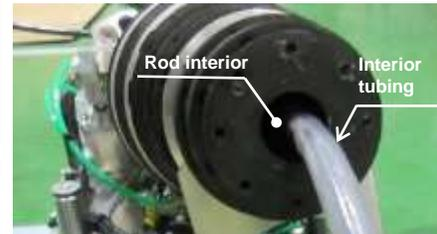
Interior tubing for power and signal cables (both wired and wireless drones)
