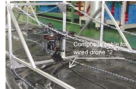
\*2 Dosimeter optical fiber (0.04 g/m) is not installed. PEEK tube for protection is installed.
