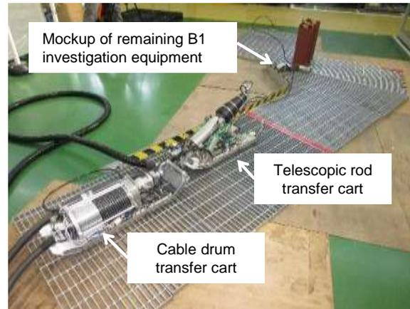
**Travelling ability verification test (wired specification)**
