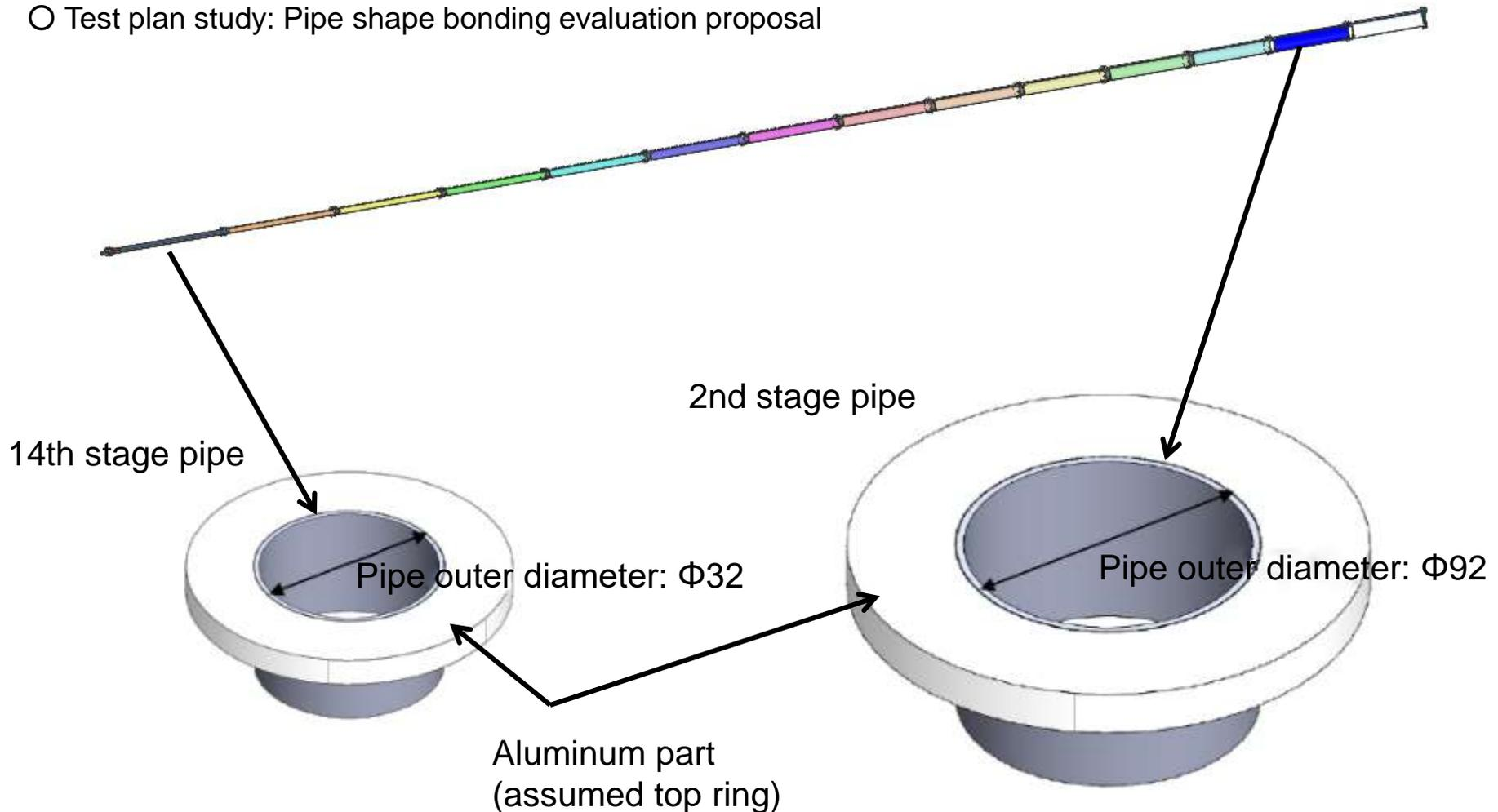
Note: 1st stage is aluminum pipe with no bonded section
