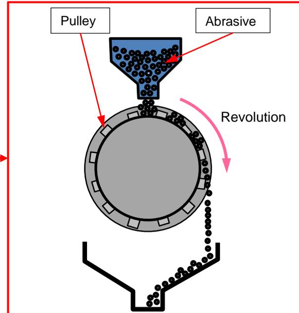
Illustration of pulley type feed mechanism
