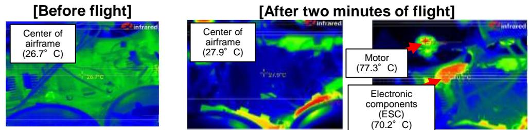
Measurement by thermal camera\* (wired drone)
