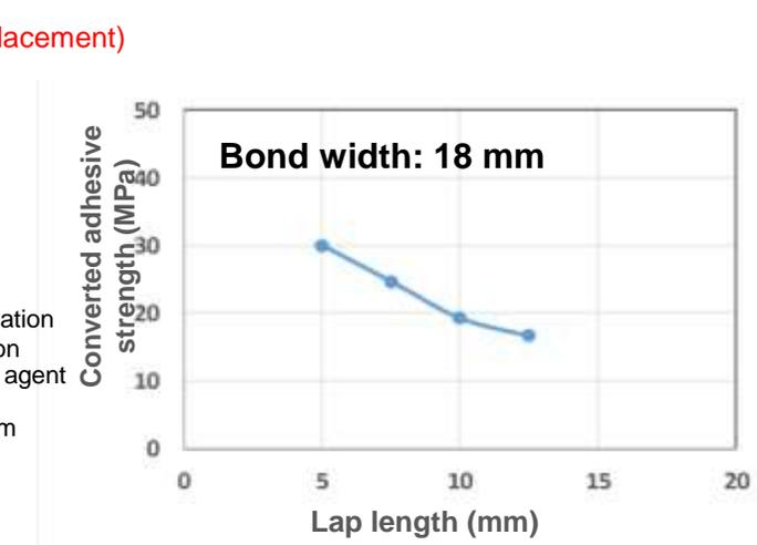
Test with constant bond width and varying lap length
