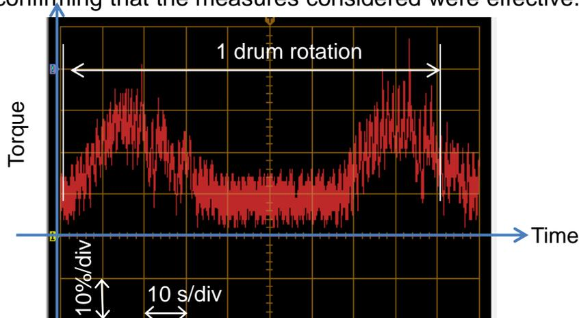
Variation in drum drive torque under no load conditions (Before improvement)
