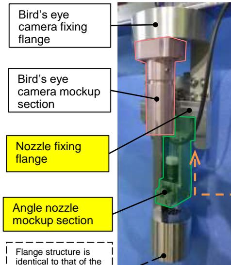
Toolhead tip (Partial element prototype)
