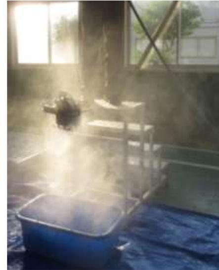
**Waterproof performance verification test (wireless specification)**
