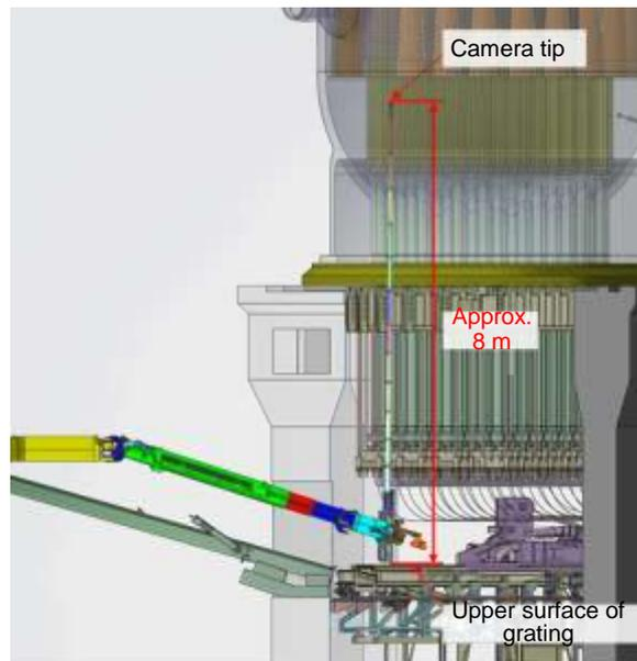
Drawing of access using telescopic pipe
