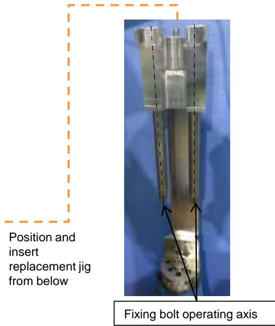
Nozzle replacement jig part prototype
