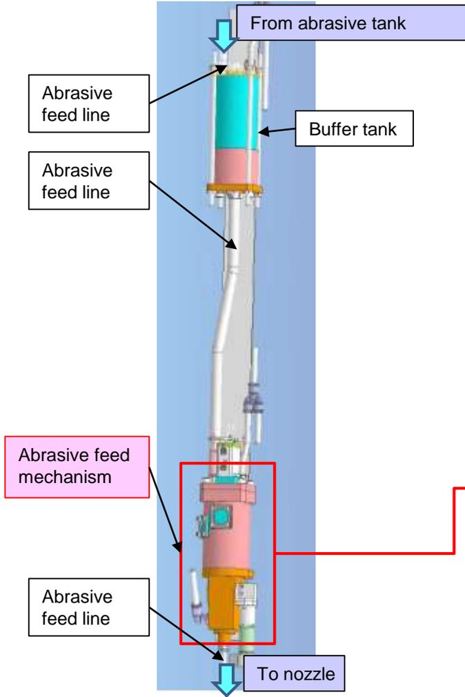
Abrasive feed mechanism external view
