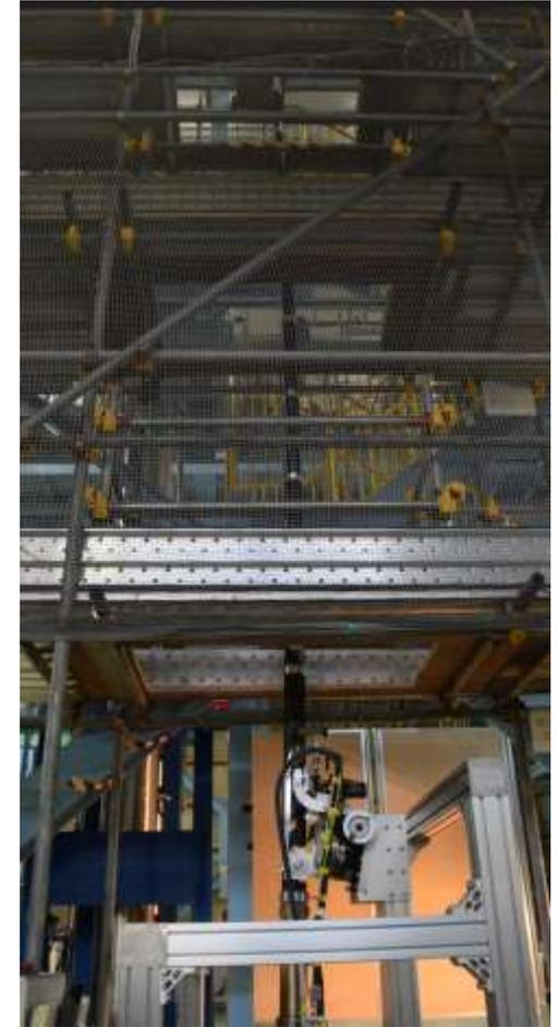
Tip is adjusted to a vertical position using the  $\alpha$ -axis and the pipe is swayed
