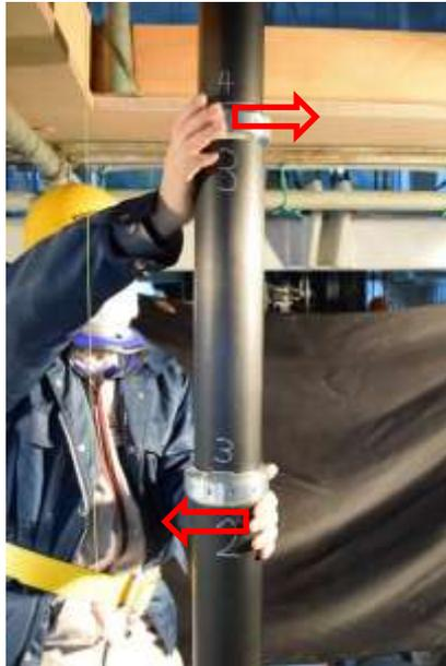
A bending force is applied to the pipe in order to tilt the 3rd stage
