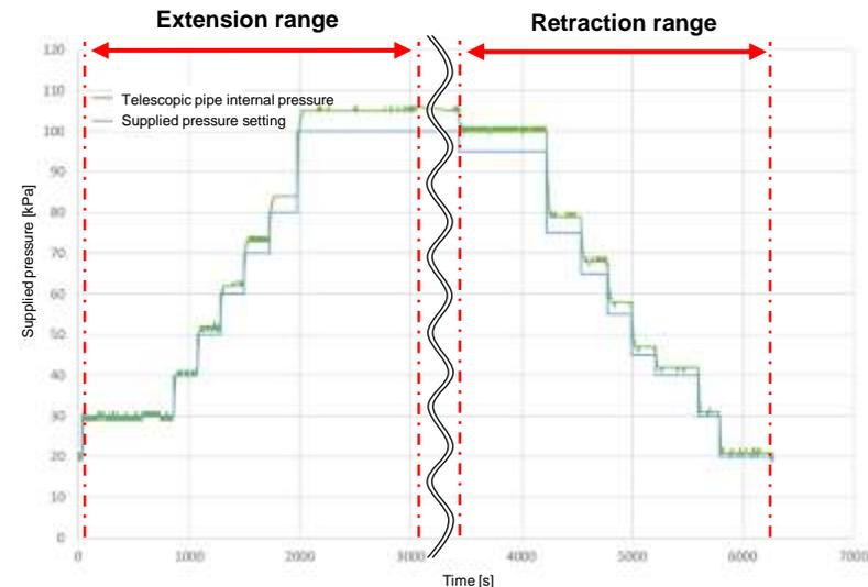
Changes in the extension length, cable tensile force, and internal pressure during telescopic pipe extension/retraction motion
