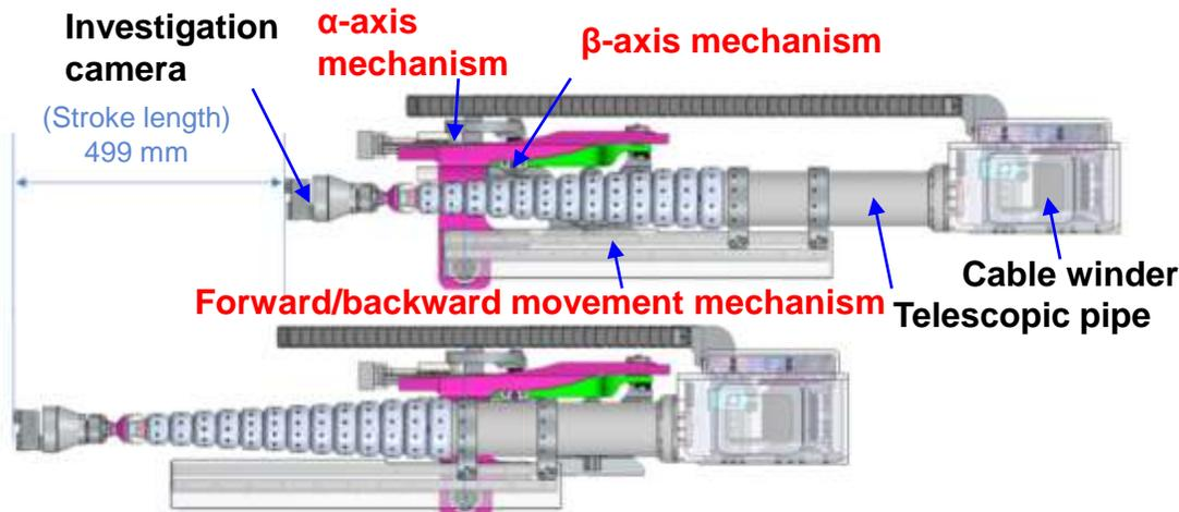
Movement by forward/backward movement mechanism
