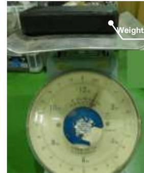
Adjustment of additional weight (Mock dosimeter (200 g) + weight (600 g))
