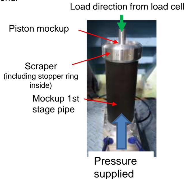
Measurements of force\* required to remove (average of 5 measurements each)
