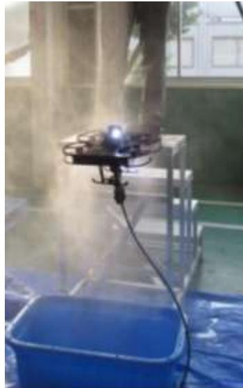
**Waterproof performance verification test (wired specification)**
