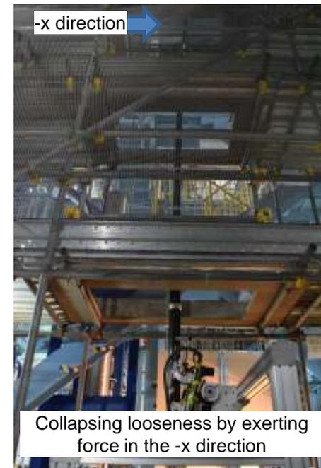
Telescopic pipe after the looseness is collapsed by applying a bending force
