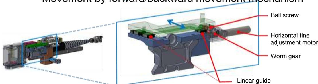
Movement by β-axis mechanism
