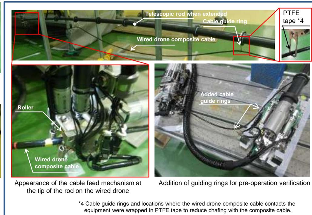
Appearance of the cable feed mechanism at the tip of the rod on the wired drone
