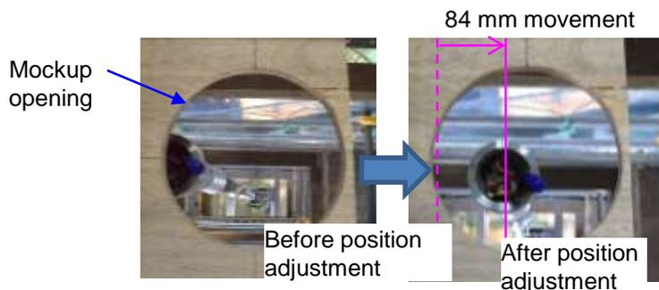
Position adjustment by  $\alpha$ -axis mechanism at the position just before the opening
