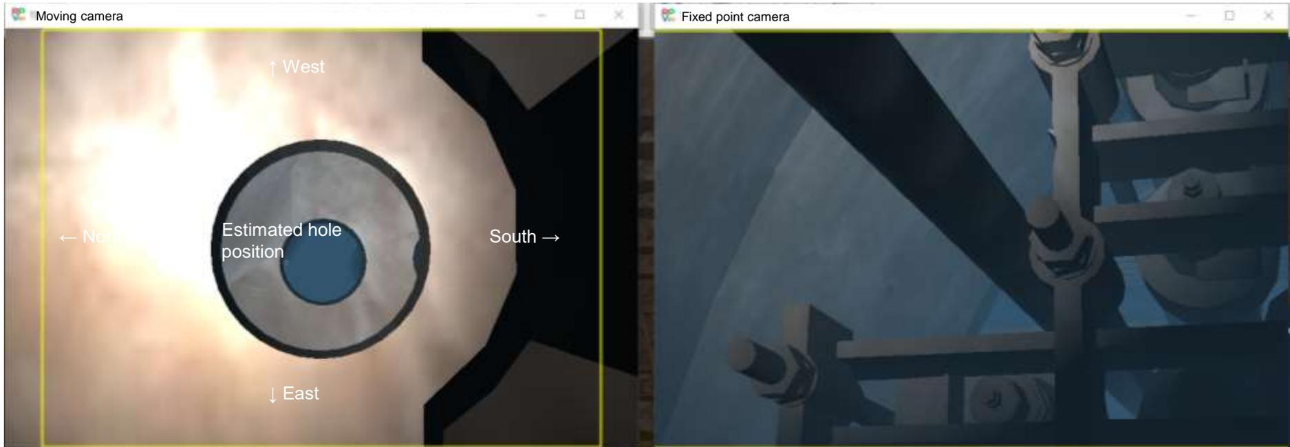
Unit 2: Camera image with telescopic pipe extended 3000 mm from retracted state (tilted 2° to the west)
