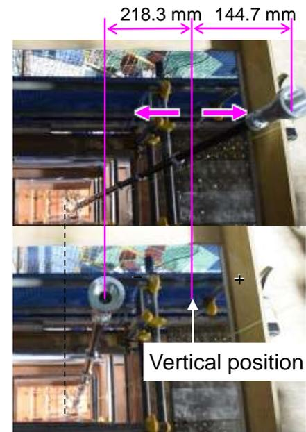
Amount of tip deviation caused by tilting due to looseness
