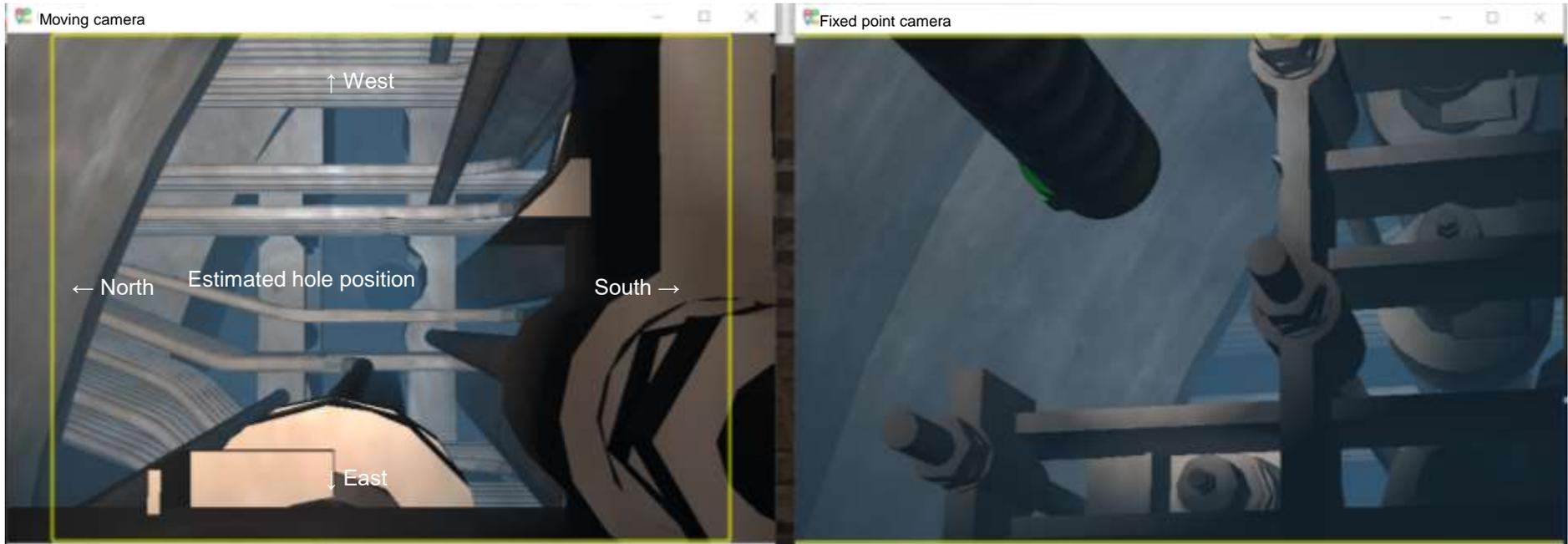
Unit 2: Camera image with telescopic pipe retracted (tilted 2° to the west)
