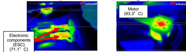
Measurement by thermal camera\* (wireless drone)
