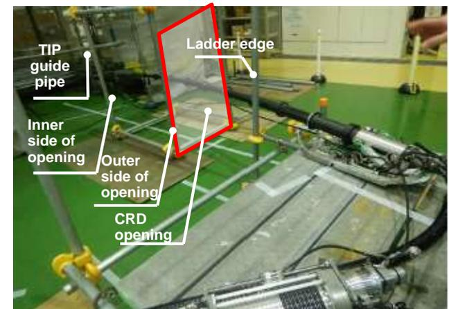
**Rod extension/retraction combined test (wired specification)**
