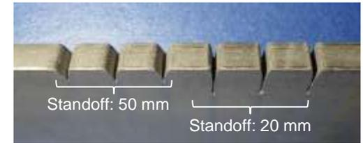
Cutting plate after cutting test (Standoff: 20, 50 mm) (top view)
