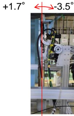
Operating range of  $\alpha$ -axis mechanism when fully extended
