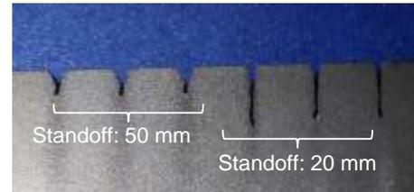
Cutting plate after cutting test (Standoff: 20, 50 mm) (front view)
