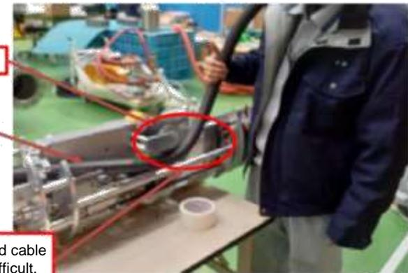
Installing  $\Phi 40$  cable
