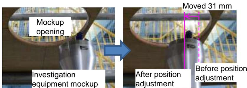
Position adjustment by  $\beta$ -axis mechanism
