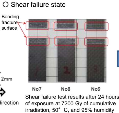
Testing system for FY2021
