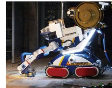
▲ Suction and blast decontamination equipment (Figure 1)
