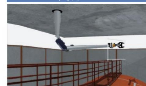
Inserting a held rod into the simulated hole placed in the top of the handrail
