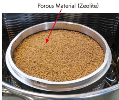
▲ Test piece in drying test (Figure 10)
