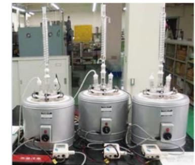
▲ Conducting the long-term corrosion test (Figure 5)
