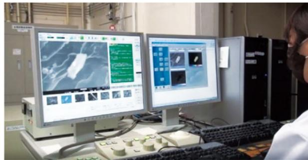
▲ Conducting a SEM\* analysis on the sample of accreted material collected inside the reactor (Figure 16)
