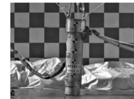
Structural test (dropped vertically)
