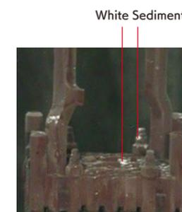
◀ Results of visual inspection of spent fuel from Unit 4 (upper tie plate of fuel mixed with rubbles) (Figure 2)
