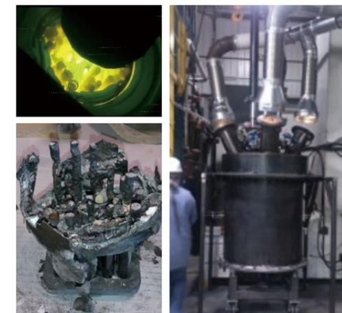
▲ Plasma-heating test on simulated fuel assembly (during heating and the test piece after)
