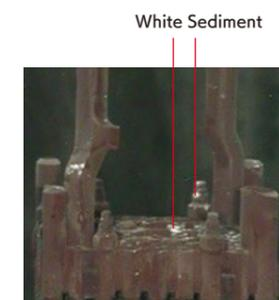
◀ Results of visual inspection of spent fuel from Unit 4 (upper tie plate of fuel mixed with rubbles) (Figure 2)
