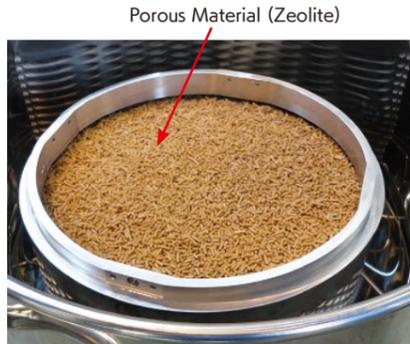
▲ Test piece in drying test (Figure 10)
