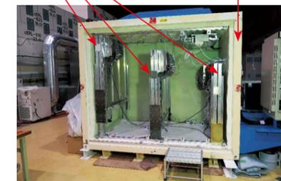
▲ Muon-transmission measuring device (Photo 1)
