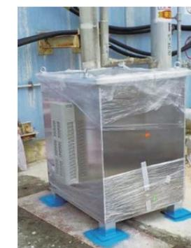
▲ Small muon-transmission measuring equipment (Photo 2)
