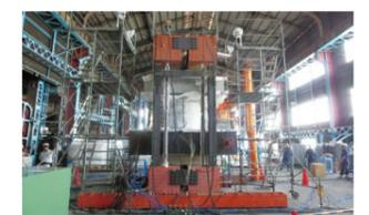
Testing the durability of the RPV pedestal
