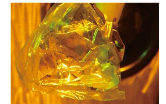
▲ The protective sheet, an analysis target obtained from the fifth floor of the reactor building of Unit 2
