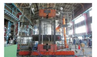
Testing the durability of the RPV pedestal
