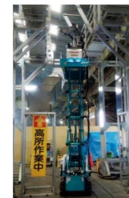
▲ Dry-ice blast decontamination equipment for high places (Figure 6)
