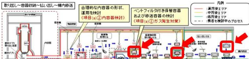
Fig.1: Dismantled waste treatment process\*1
