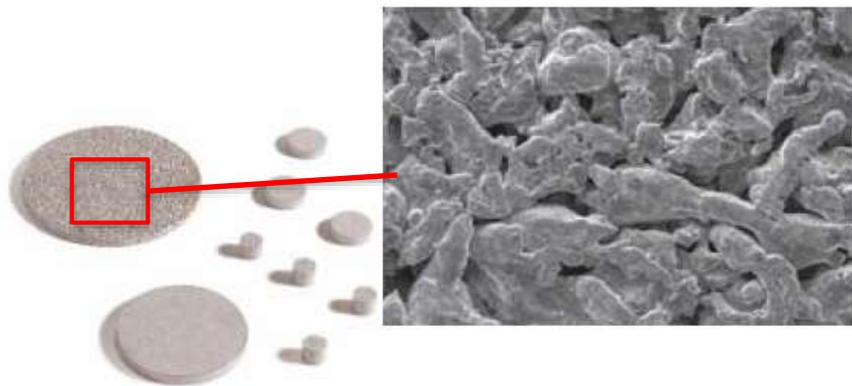
Fig. 1 Sintered metallic filter manufactured by Poral\*1
