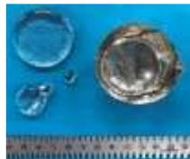
The mixed reagent is heated at 1200°C and melted to test manufacture the top off frit material
