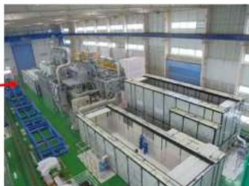
External appearance of large component decontamination equipment
