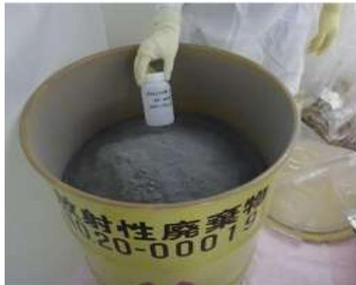
Sampling location (Temporary storage chamber) The incinerated ash drum and the collected samples
