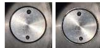
Fig. 3 Expansion of ring spring
