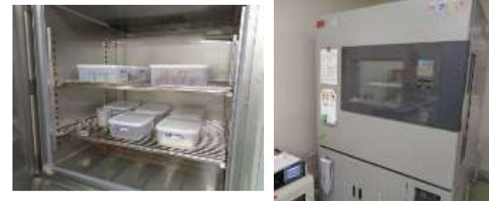
Fig. 1 Freezing-thawing test equipment and test status
