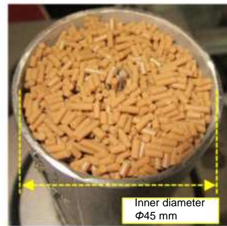
Figure: External appearance of a test container filled with water containing piece samples
