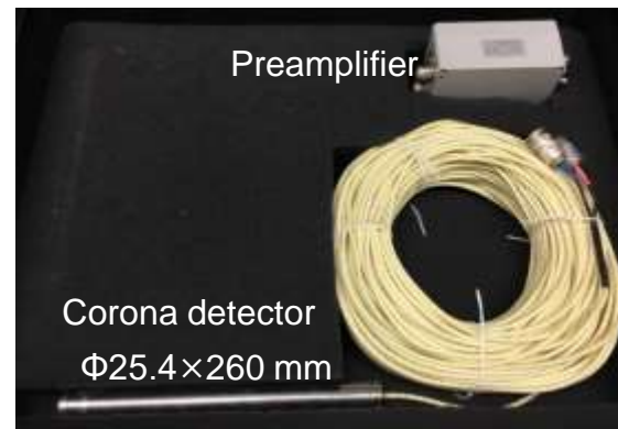
Figure 1 Appearance of Corona-based detector ( ^{10}\text{B} )
