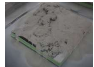
Figure 6 Using a liquid → solidification type absorber for fuel debris with large unevenness
