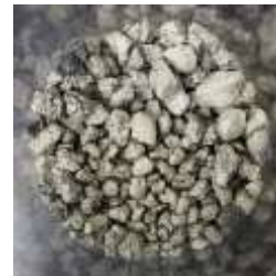
Figure 3 Using a liquid → solidification type absorber for pebble-like fuel debris
