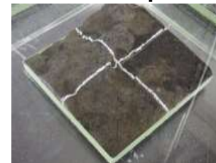
Figure 6 Using a liquid → solidification type absorber for fuel debris with large unevenness
