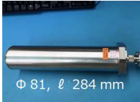
Multicell-based He-3 proportional counter
