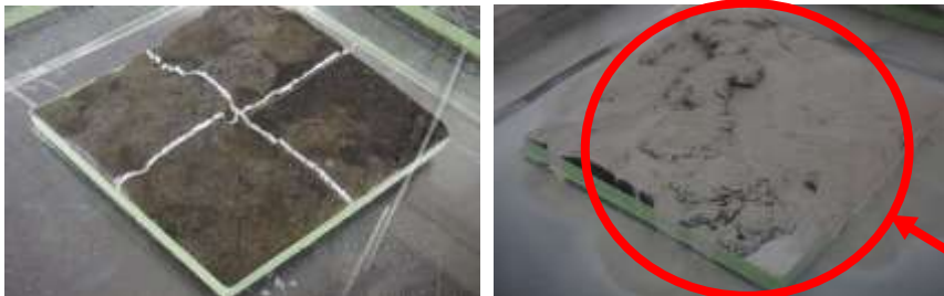
Figure An example of covering uneven surface with water glass absorber
