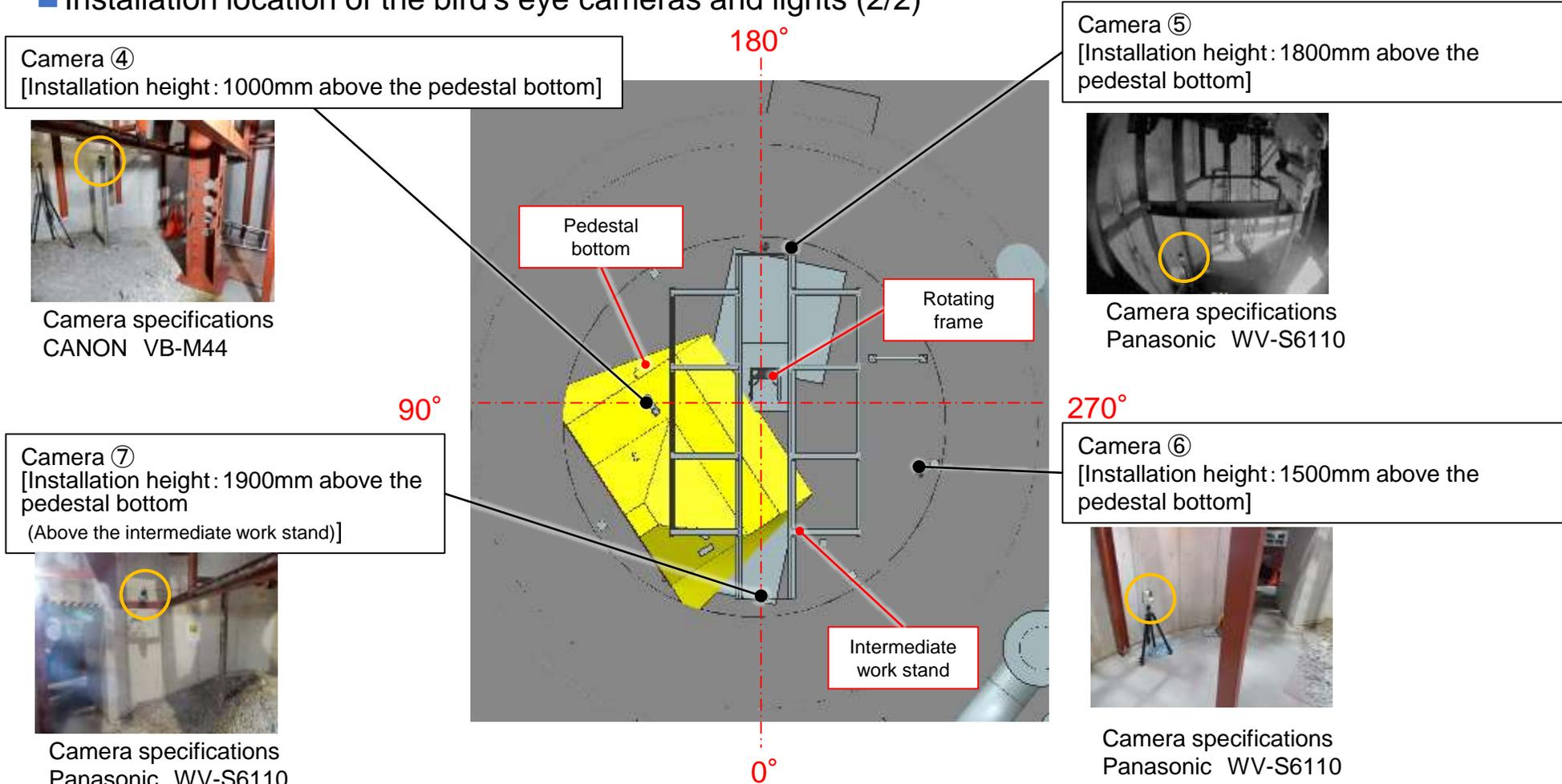
Camera installation location (Floor plan from the intermediate work stand to the pedestal bottom)
