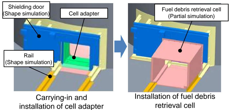
Illustration of element tests
