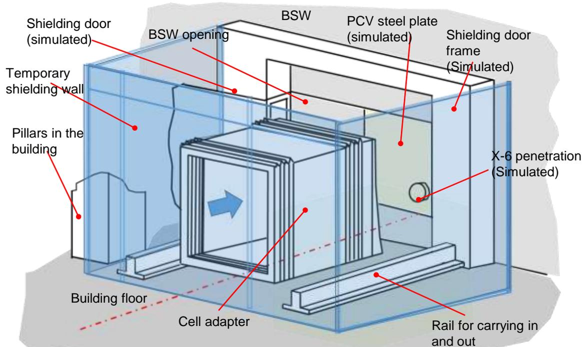
\* The cell adapter is transferred using a generic crane and verified.
