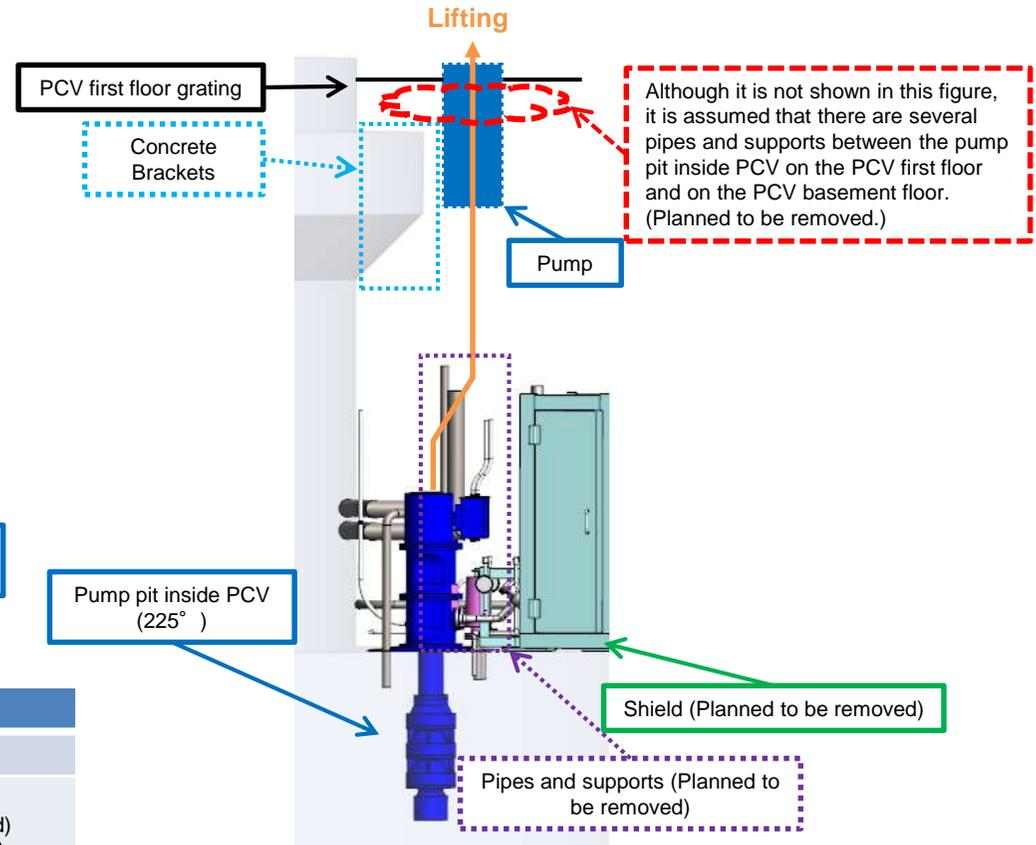
Layout drawing of Unit 1 PCV basement floor
