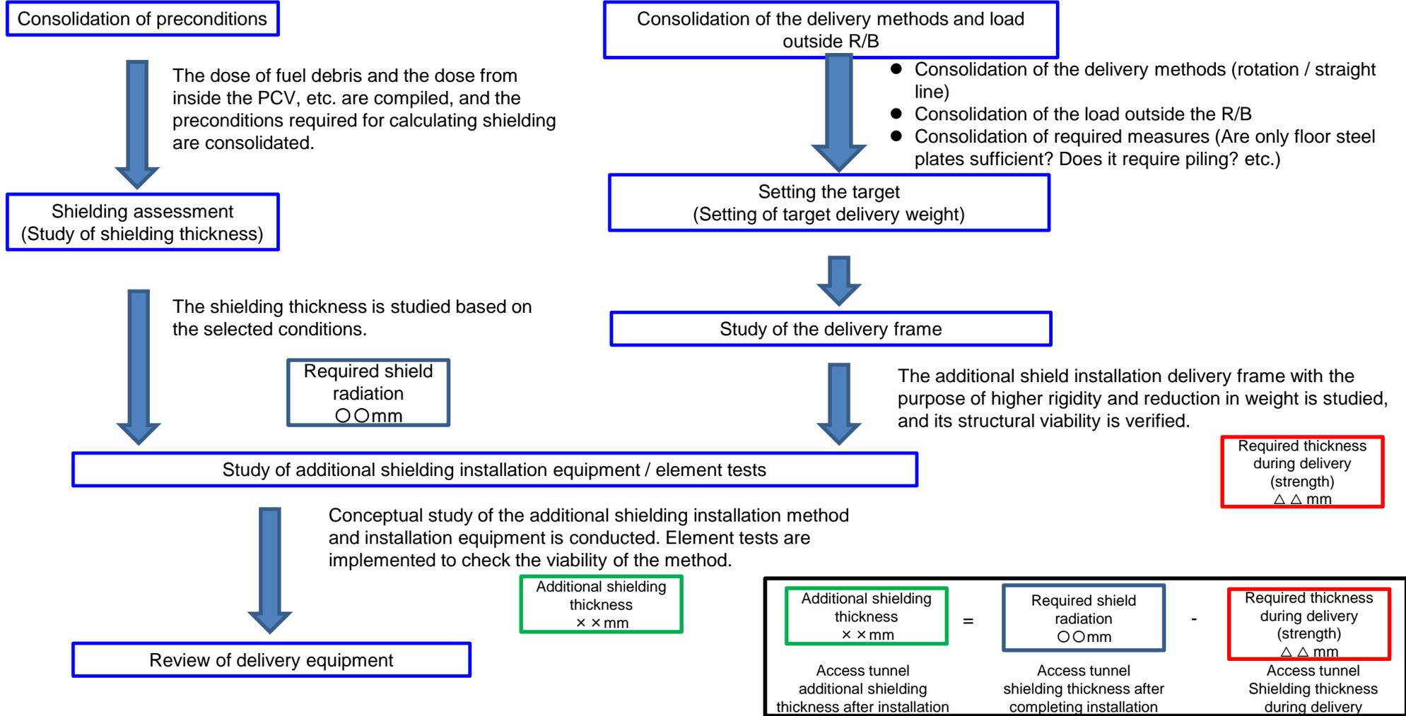
Small access tunnel delivery weight ⇒ Downsizing the ancillary facilities such as temporary building, etc. ⇒ Shortening of schedule and reduction in cost
