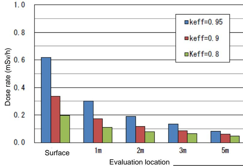
1mSv/h or less is satisfied even when the shielding thickness is 250mm.
