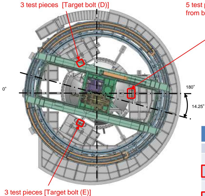
5 test pieces [Target bolt (A, B, C from below)]
