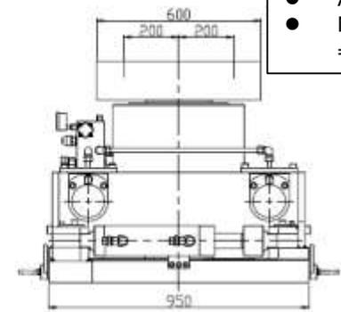
Ground pressure of the lower surface of the floor steel plates:  $P_{max}' = 2,077.2 \text{ [kN/m}^2\text{]}$
