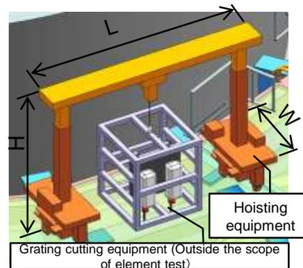
Example image showing the use of the hoisting equipment on the site
