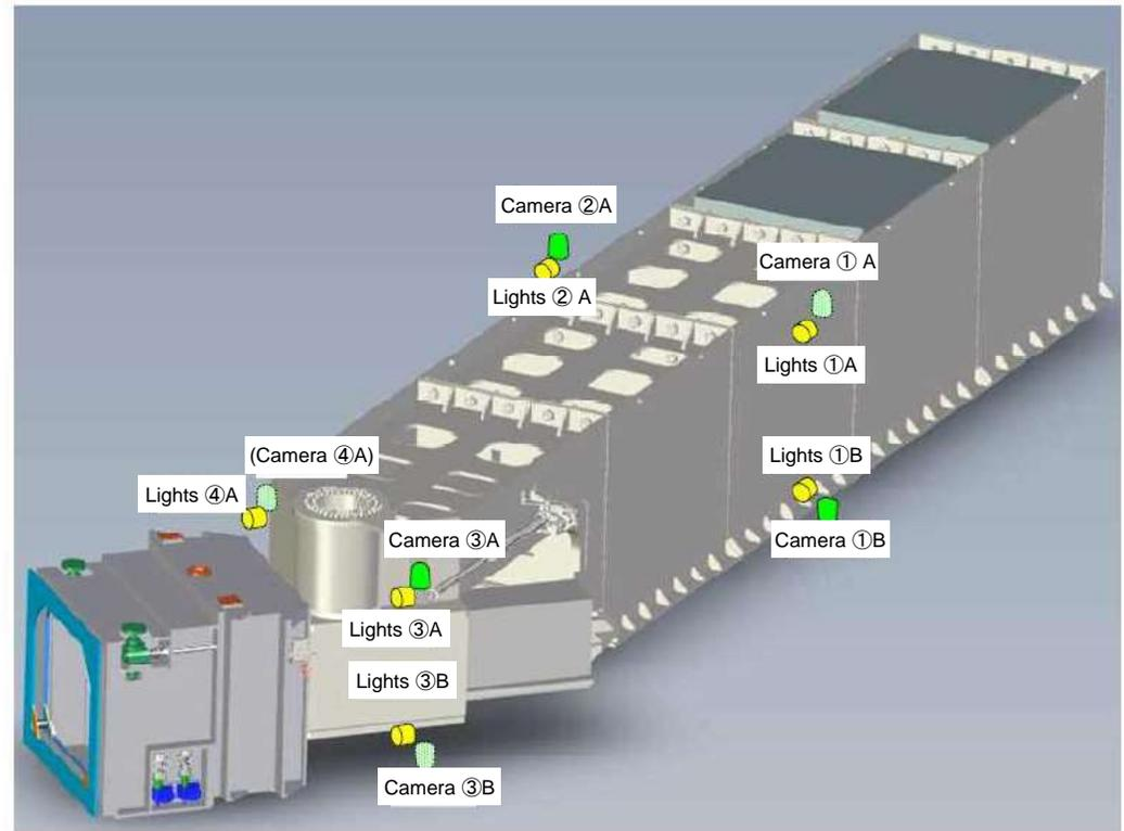
② PCV connection sleeve installation and welding by remote operation: (a) Remote installation [Arrangement of cameras]
