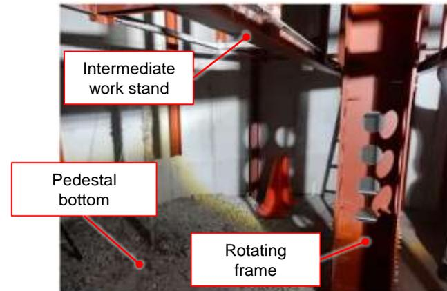
Simulated CRD exchanger (lower part)
