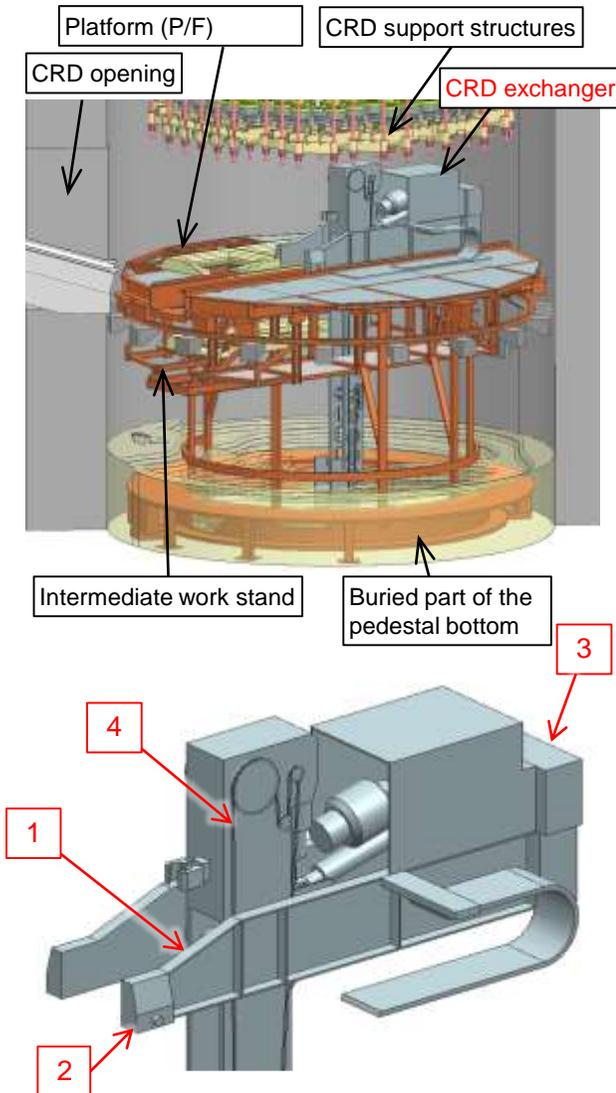
② Disassembly of CRD exchanger
