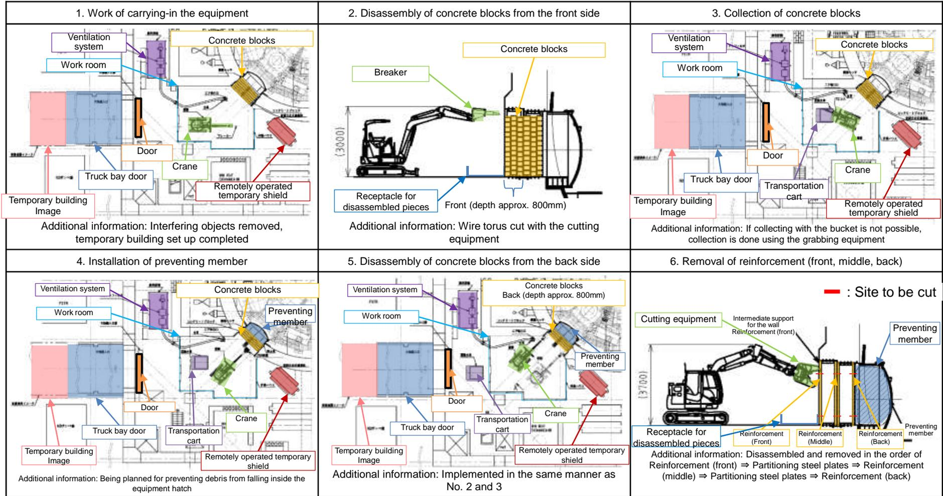
Preventing member: Planned to be installed by opening a through hole into the block by means of core boring, etc. The purpose of installing it is to prevent disassembled pieces from falling in between the PCV and BSW and preventing the equipment hatch from getting damaged, but its necessity needs to be discussed further.
