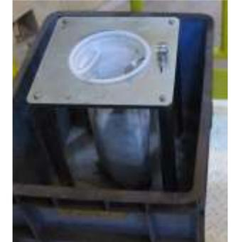
Collection of abrasive after cutting 1 stud bolt
