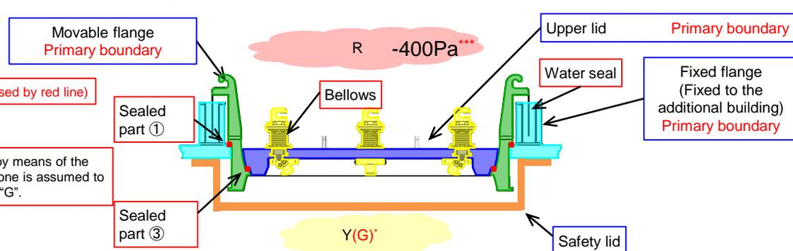
(1) Preparing for carrying-in the container: Removing the safety lid
