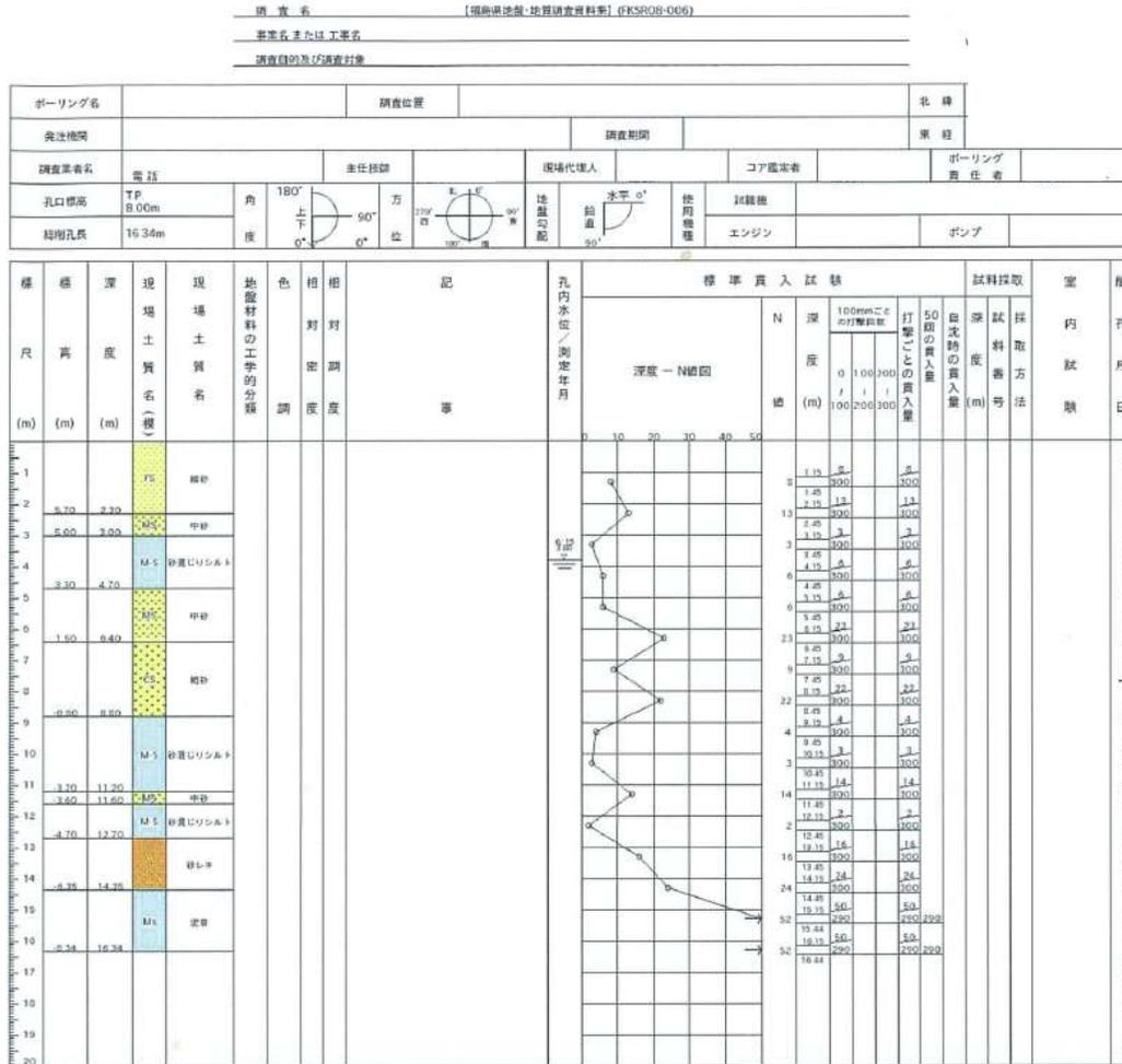
(Note) Subsurface exploration of the area where equipment will be installed needs to be conducted when actual equipment is studied.
