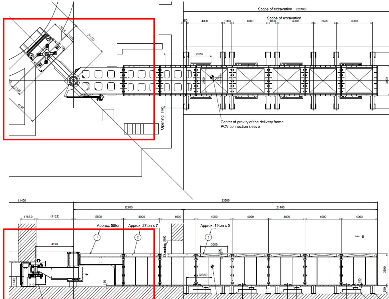
The test equipment is made up of the mechanical equipment within the red frame, BSW opening and equipment hatch.
