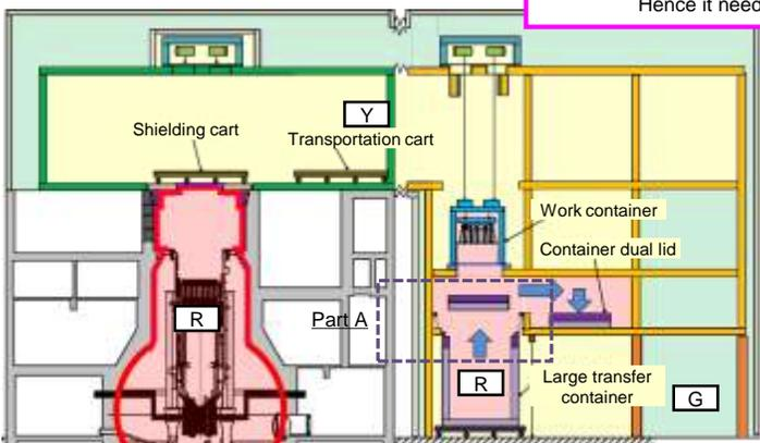
If the space between the upper lid and lower lid is not completely air-tight, the upper surface of the lower lid gets contaminated. Hence it needs to be air-tight to some extent.
