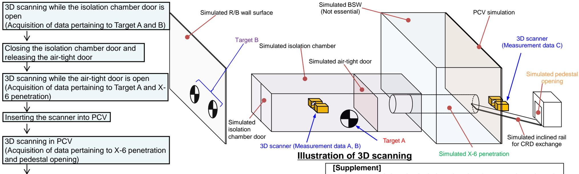
The relation between R/B wall surface, X-6 penetration and pedestal opening is ascertained in terms of coordinates based on the measurement data A, B and C, and the installation reference line is marked on the R/B floor after the isolation chamber is removed (for verifying accuracy).
