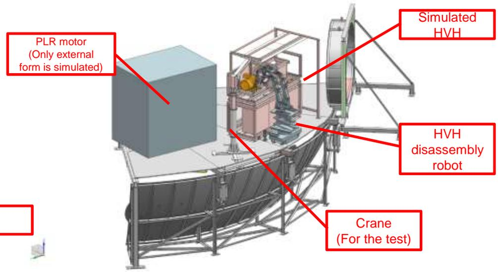
Illustration of the simulation for the element test
