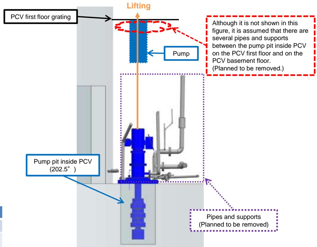
Layout drawing of Units 2, 3 PCV basement floor
