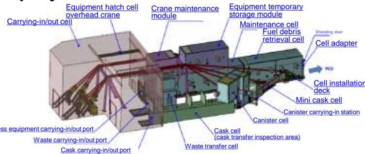
Composition of the fuel debris retrieval equipment (suspension bridge type cell)
