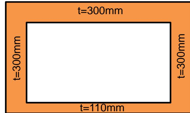
(Current state) Cross-section of access tunnel
