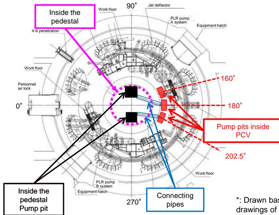
Layout drawing of PCV basement first floor in Units 2, 3\*
