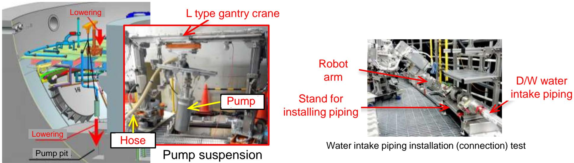
Submersible pump suspension test
