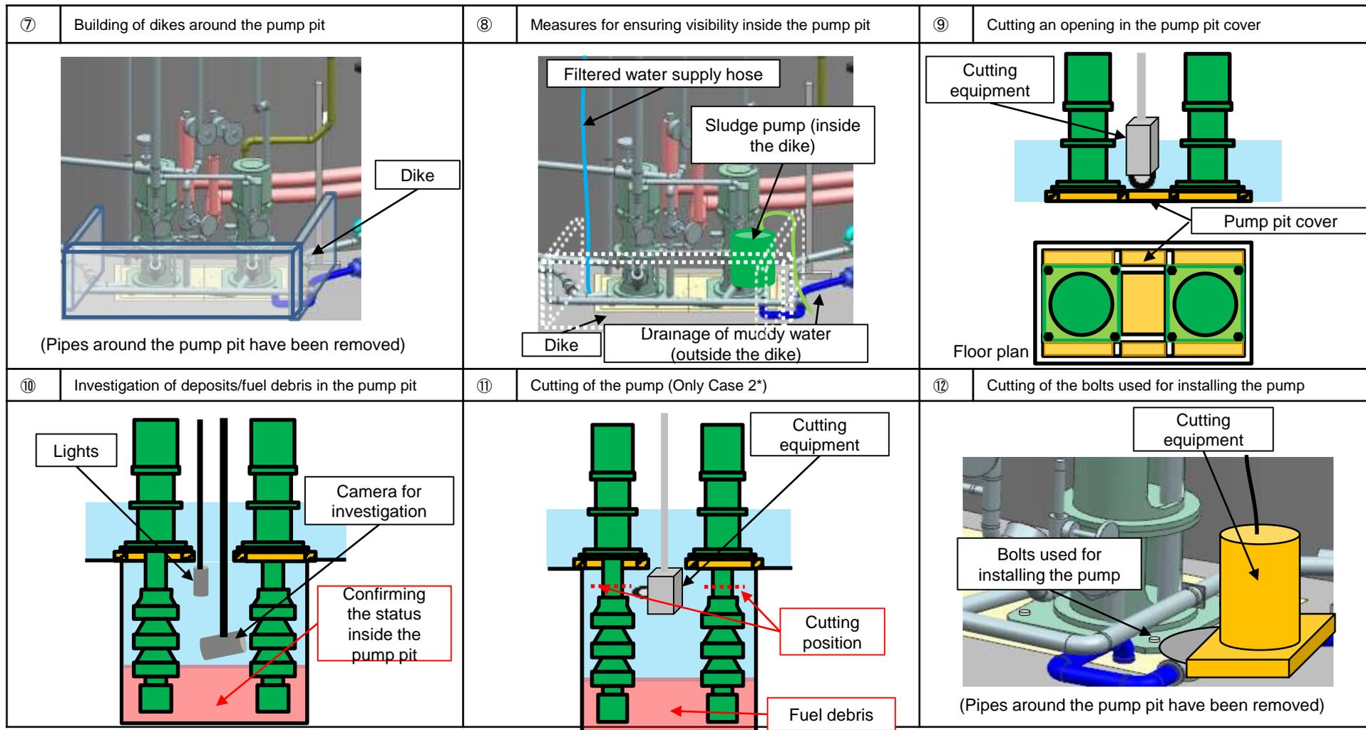
③ Interference removal from pump pit
