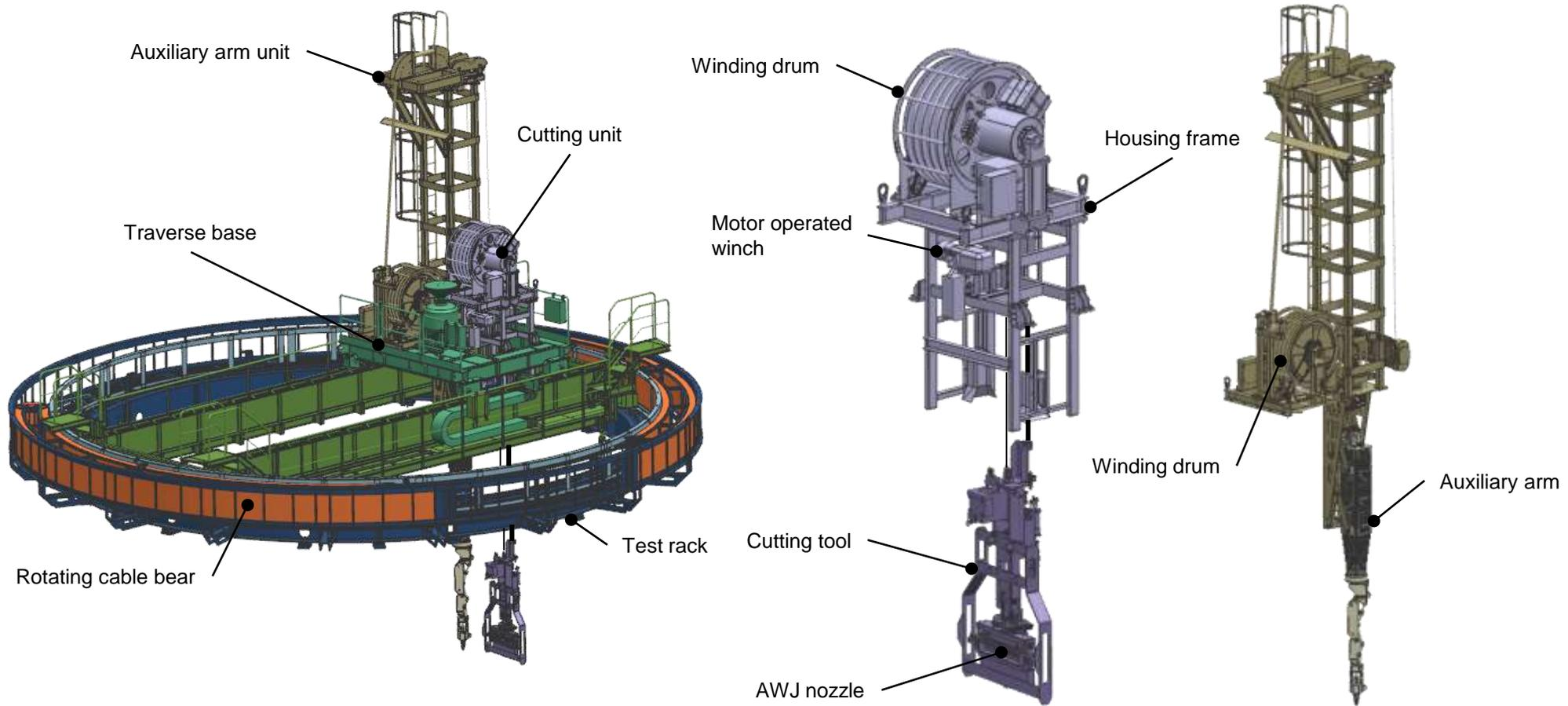
Big-picture view of the RPV disassembly equipment (Polar crane) Detailed drawing of the cutting unit Detailed drawing of auxiliary arm unit
