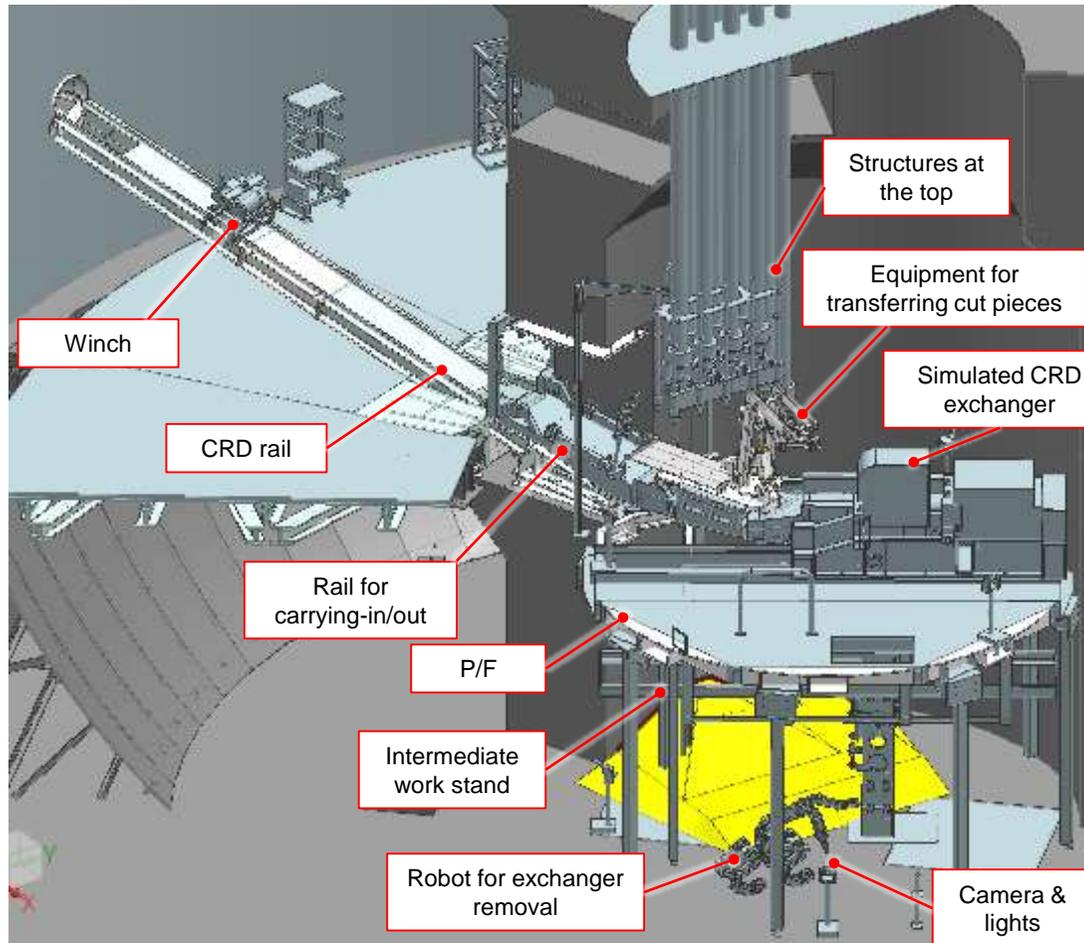
Facility for mock-up test of the inside of the Unit 2 pedestal (Illustration of overall view)
