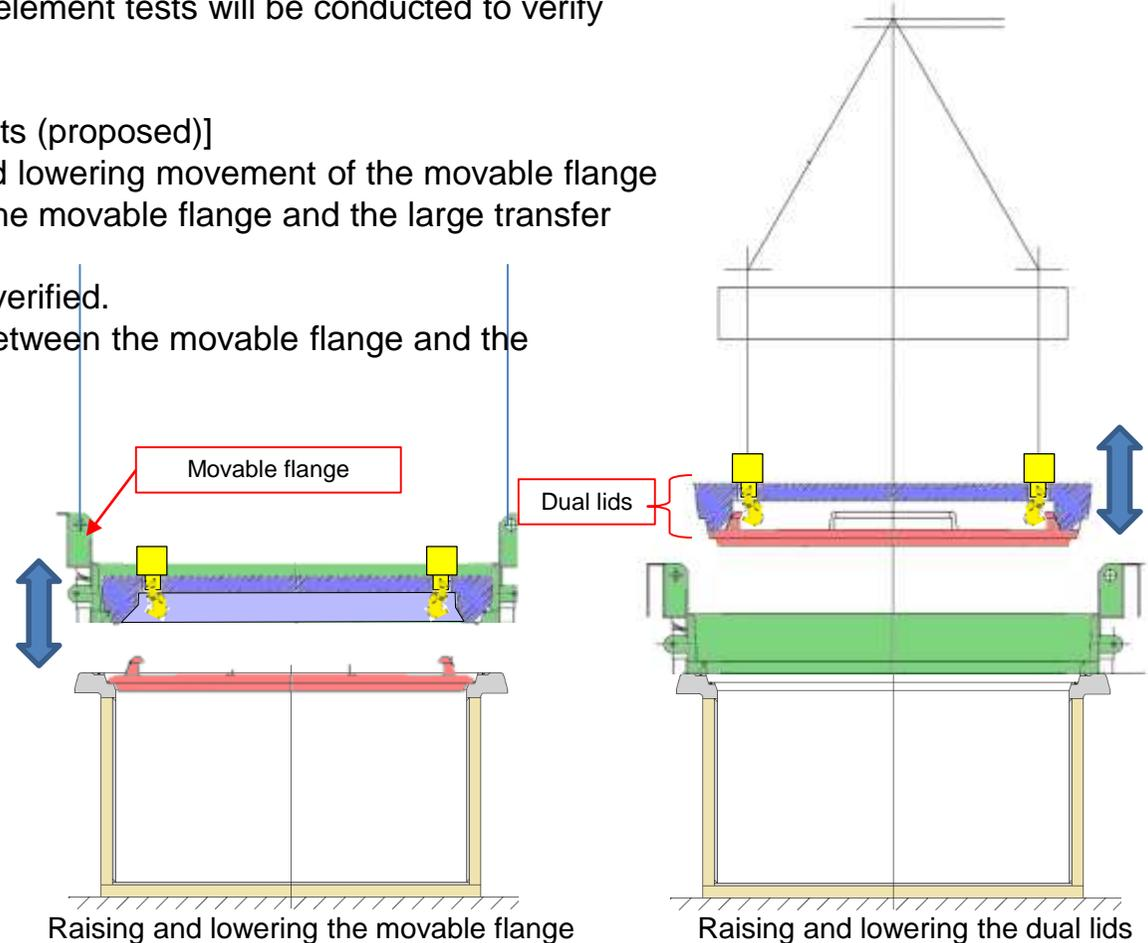
Illustration of the large transfer container element test
