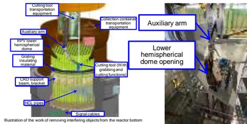
Illustration of the work of removing interfering objects from the reactor bottom
