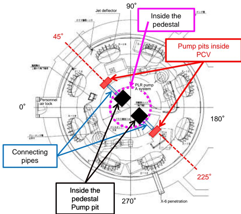
Layout drawing of PCV basement first floor in Unit 1
