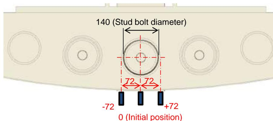
Illustration indicating the scope of operation of AWJ nozzle during cutting
