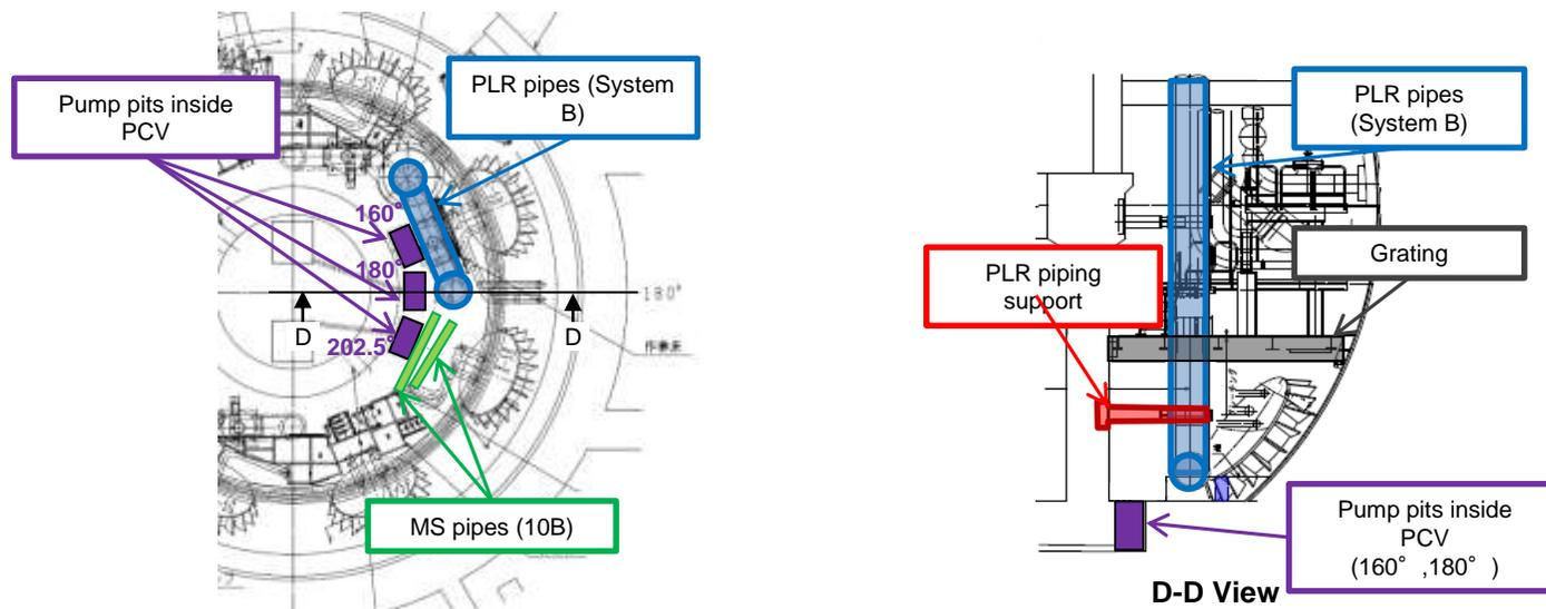
Floor plan of first floor in Unit 2\* (180°: D-D)
