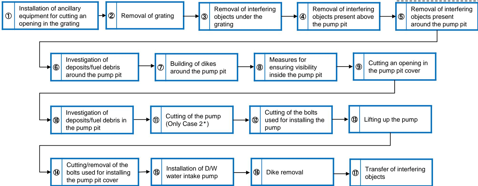
③ Interference removal from pump pit
