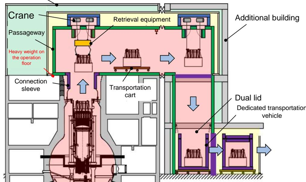
Illustration of the method of transferring unitized structures
