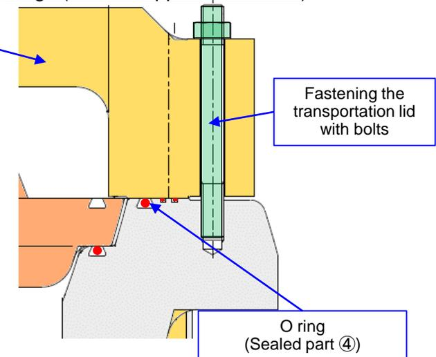
Detailed drawing of container flange (with the transportation lid installed)
