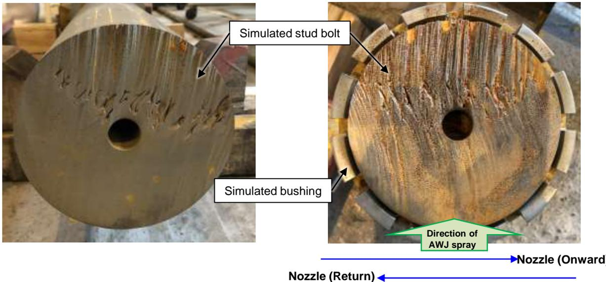
State of surface to be cut during element tests (Bolt D)
