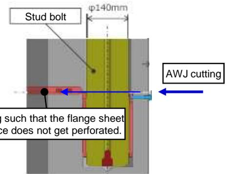
● Even if the cutting is performed where the nut is positioned, pulling it up would be difficult as it is a stud bolt.
