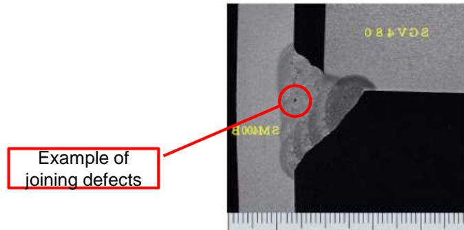
Welding position: Vertical upward
