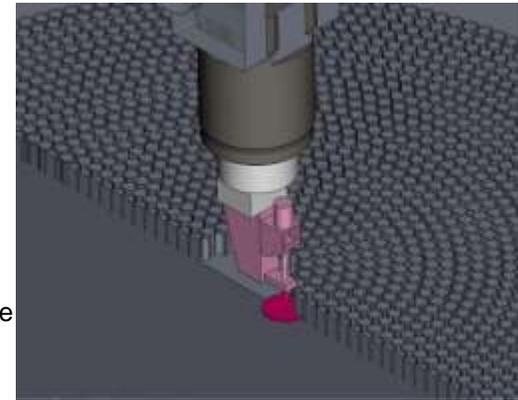
Making a hole at the center for inserting the circular cutter ⇒ cutting the reactor core
