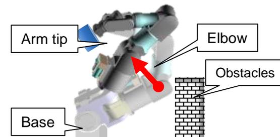
Figure 2 Evasive maneuvering of the manipulator with redundant degree of freedom
