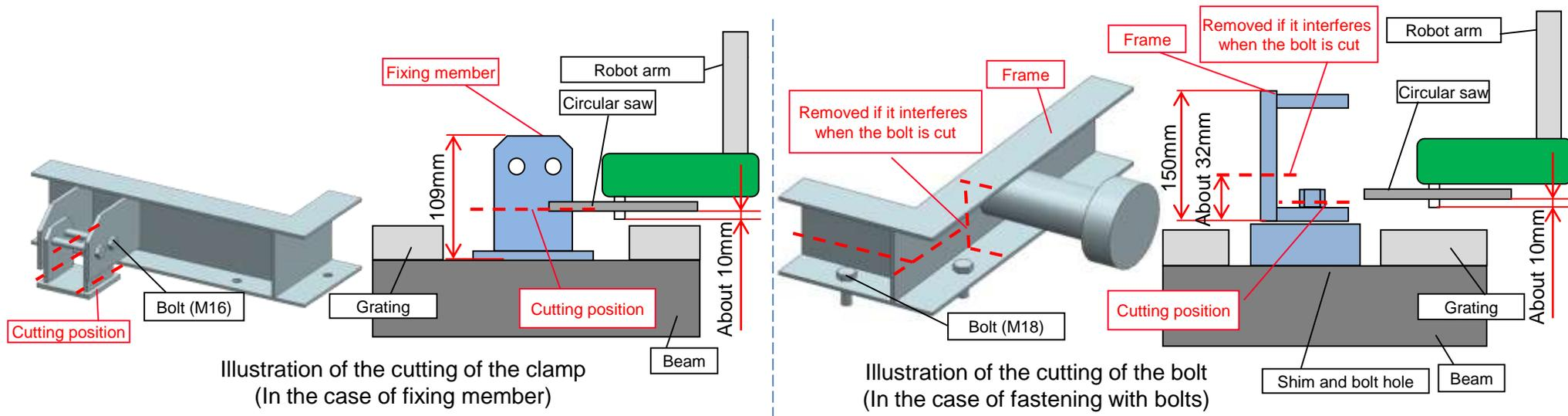
After disassembling and removing HVH, there will be remnants of about 10mm on the grating.
