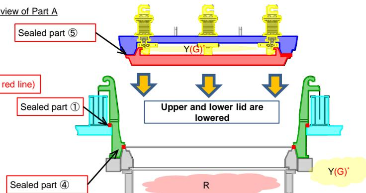
(7)-1: Inspection and cleaning the sealed surface (removing trash, etc.)
