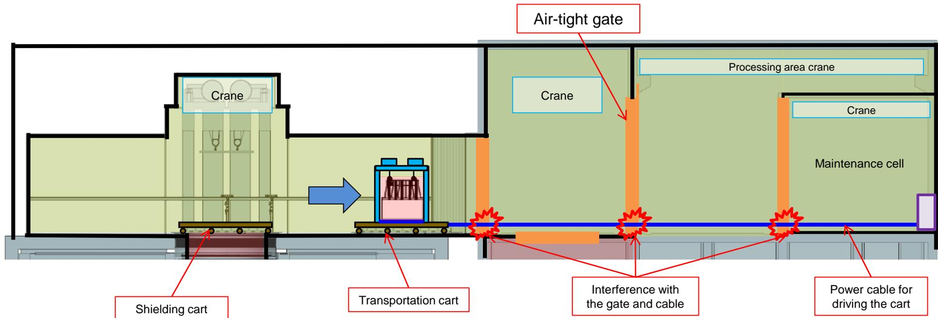
Illustration of the large transportation equipment (The layout of the additional building is being examined. This drawing is based on FY2020 results.)
