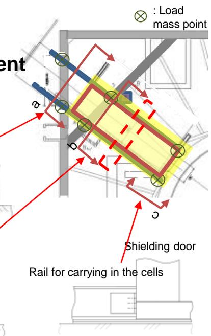
Connecting part of the rail for carrying-in the shielding door and cell (Enlarged view) Cross section c
