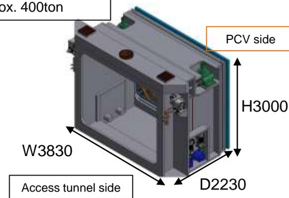
Bird's eye view of the PCV connection diagram (Unit 1)
