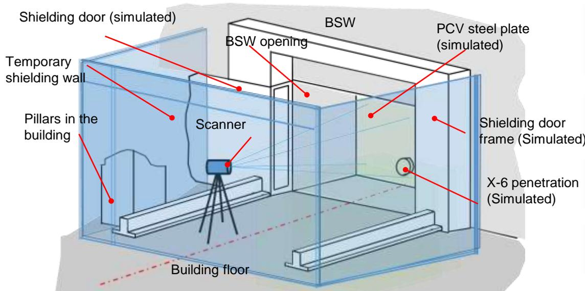
\* The 3D scanning was performed at a prescribed location and the flange was manufactured based on those results.
