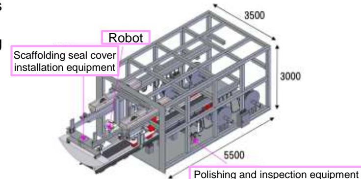
Illustration of PCV connection sleeve welding equipment
