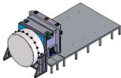
Illustration of PCV connection sleeve remote welding test (Before equipment installation)
