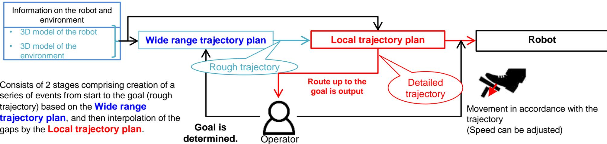
Consists of 2 stages comprising creation of a series of events from start to the goal (rough trajectory) based on the **Wide range trajectory plan**, and then interpolation of the gaps by the **Local trajectory plan**.
