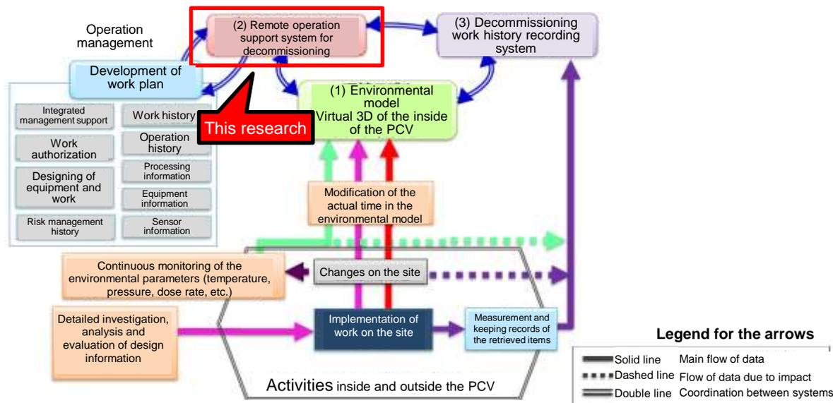
Data utilization proposal by the Fuel debris retrieval monitoring/support/integrated management WG
