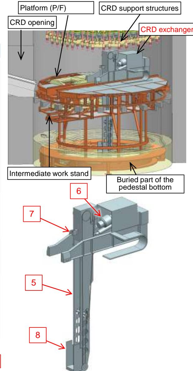
② Disassembly of CRD exchanger
