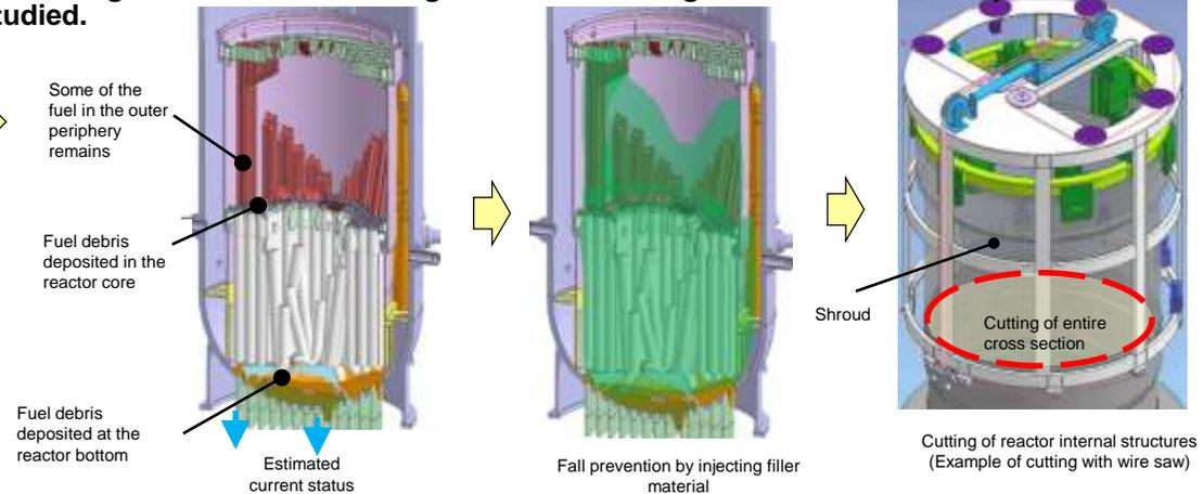
Studies will be conducted on the method of cutting structures and the concept of the equipment, and element tests will be conducted related to the filling and solidification material for the reactor core.
