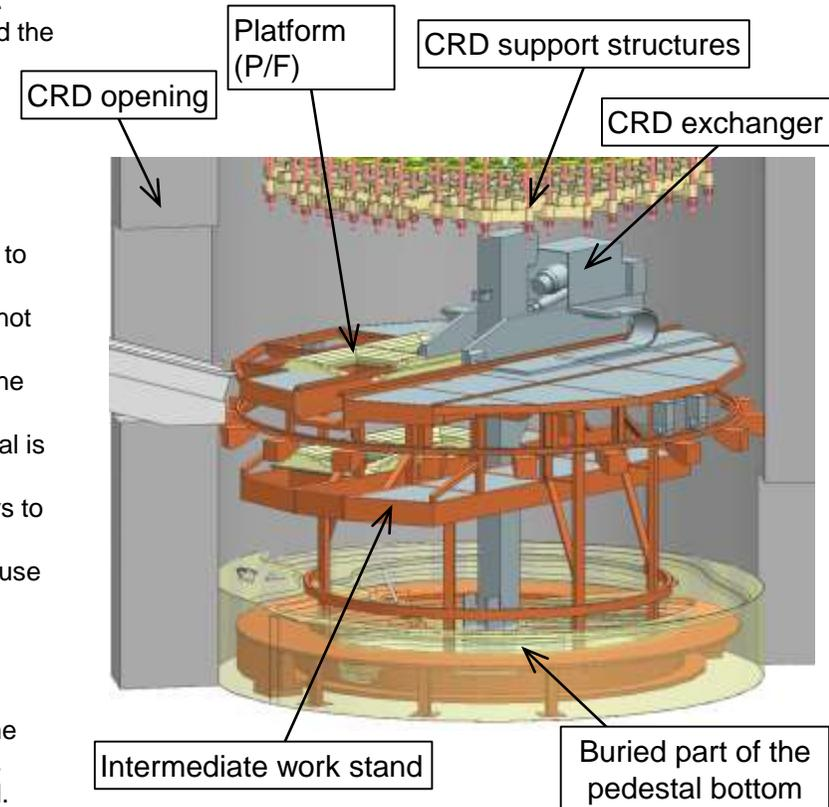
Illustration showing an overview of the inside of the pedestal (Example of Unit 2)
