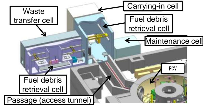
Illustration showing how the PCV and additional building are connected
