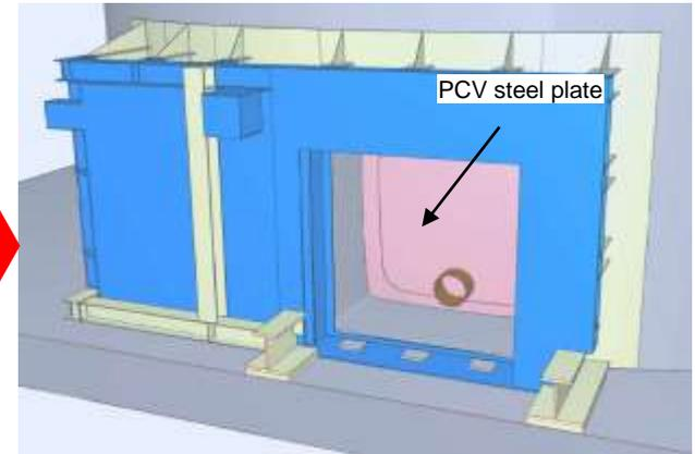
③ BSW drilling (Temporary closure and reduction in length of X-6 penetration)
