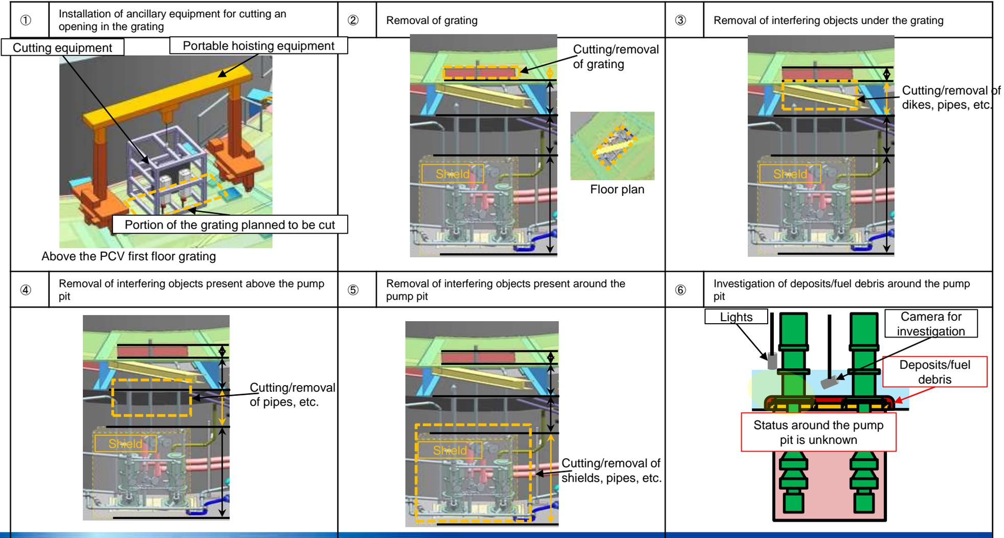
③ Interference removal from pump pit
