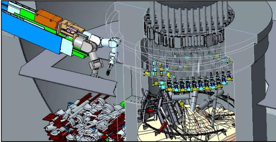
The work of removing interferences from outside the pedestal will be simulated. (Interfering objects will be left behind at the PCV bottom)
