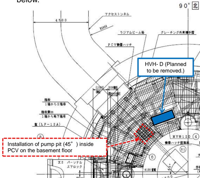
Layout drawing of Unit 1 PCV first floor
