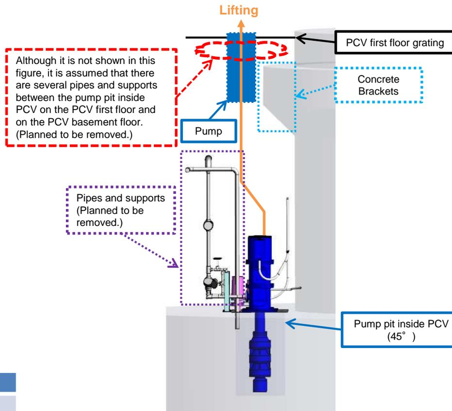
Layout drawing of Unit 1 PCV basement floor
