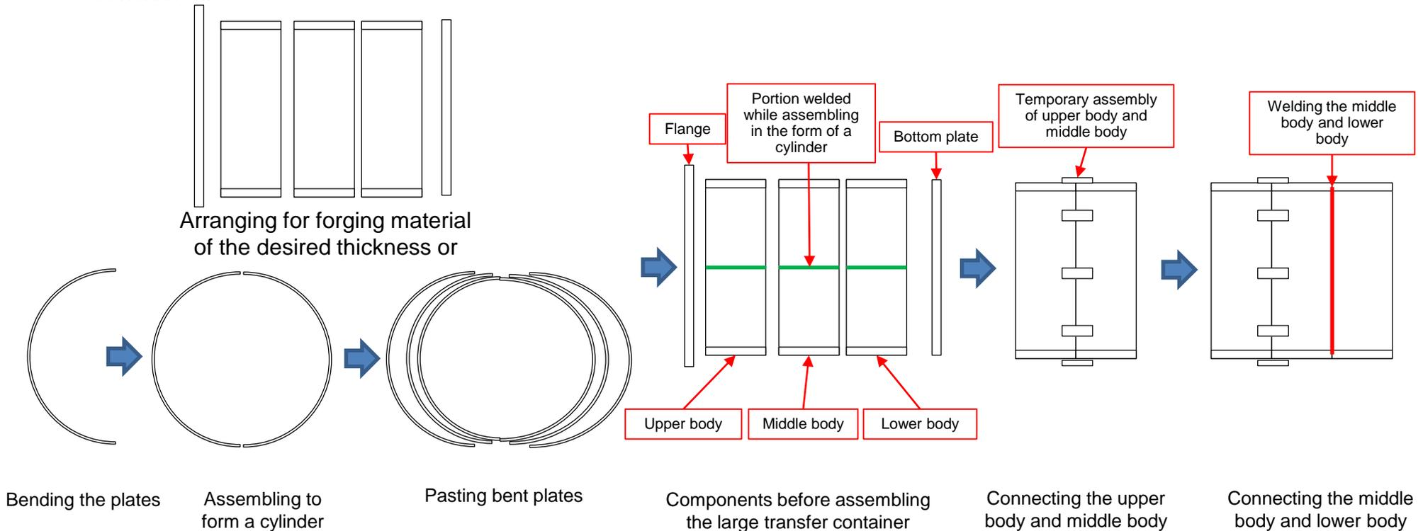
Study of the procedures for fabricating large transfer containers
