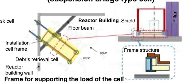
Frame for supporting the load of the cell
