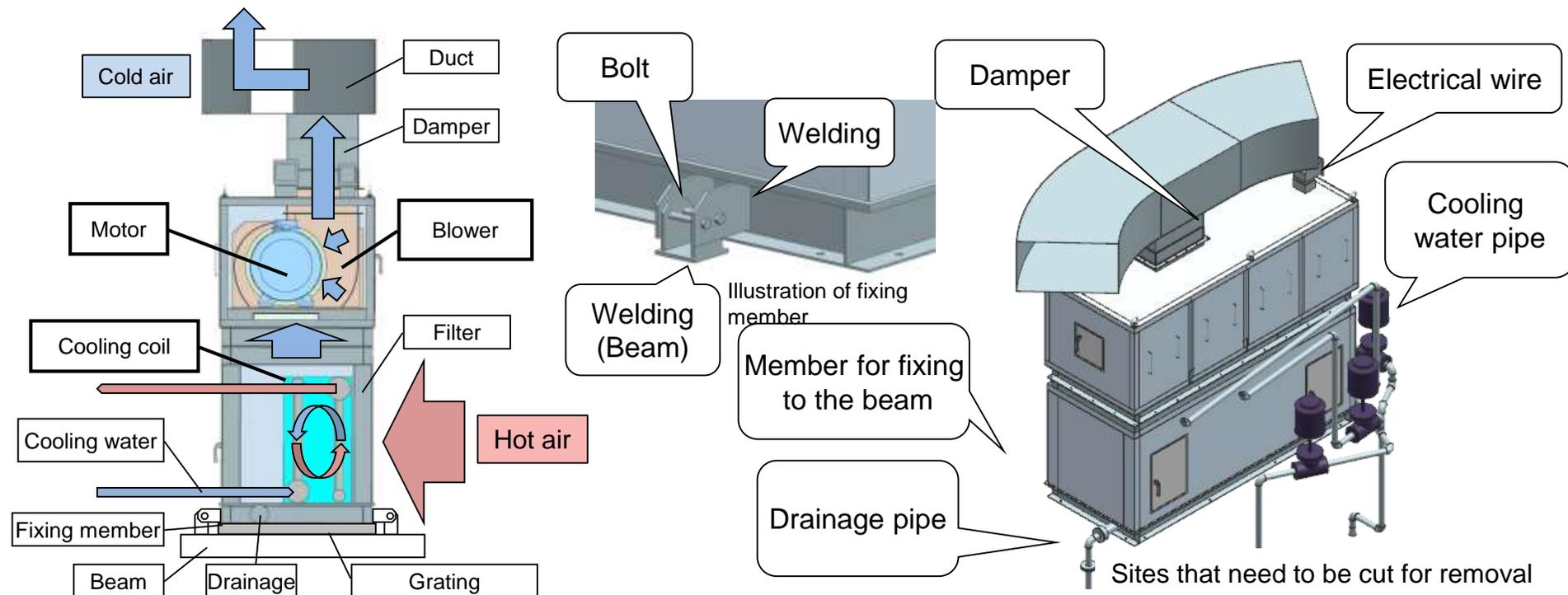
(Structures such as fixing members, etc. that are not shown in the outline drawing are assumed based on Unit 1.)
