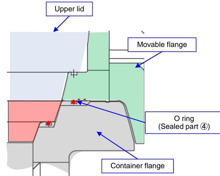
Detailed drawing of container flange (with the upper lid installed)
