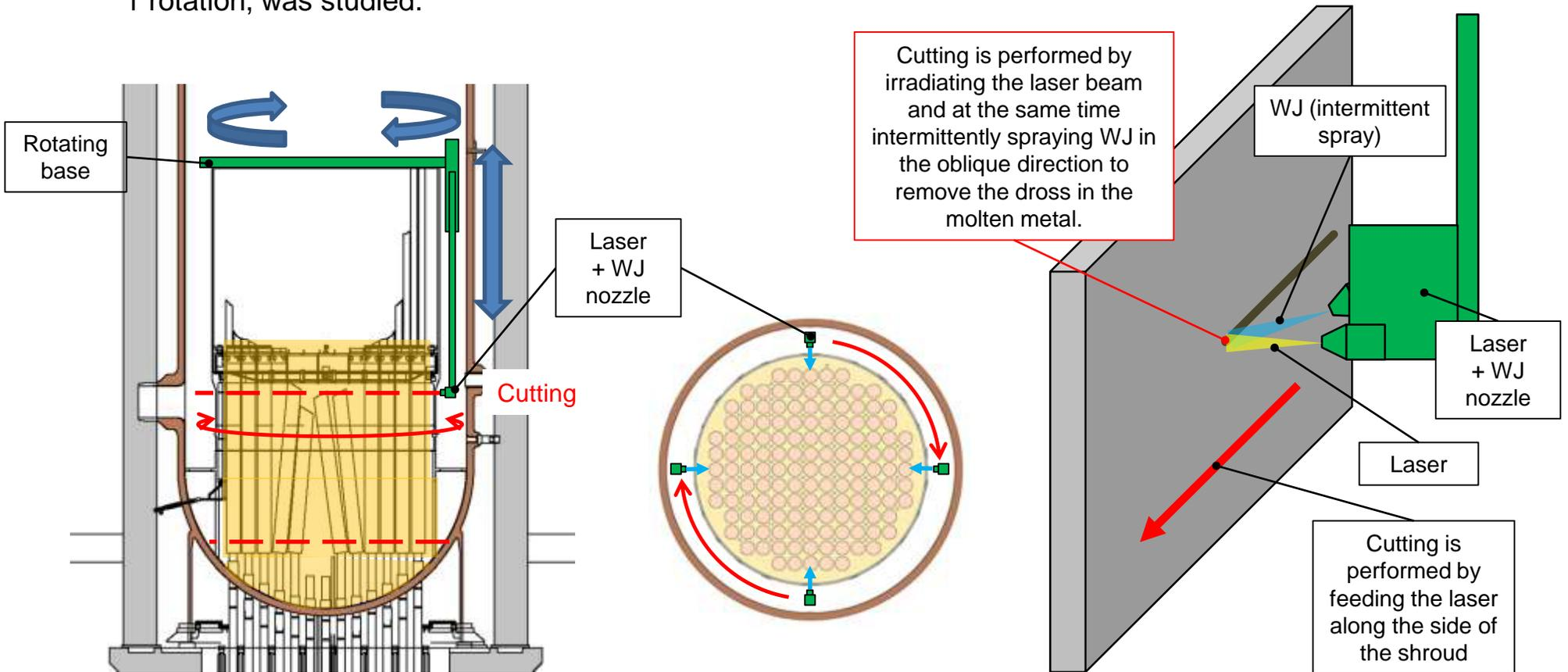
Illustration of the cutting equipment for reactor internal structures (shroud)
