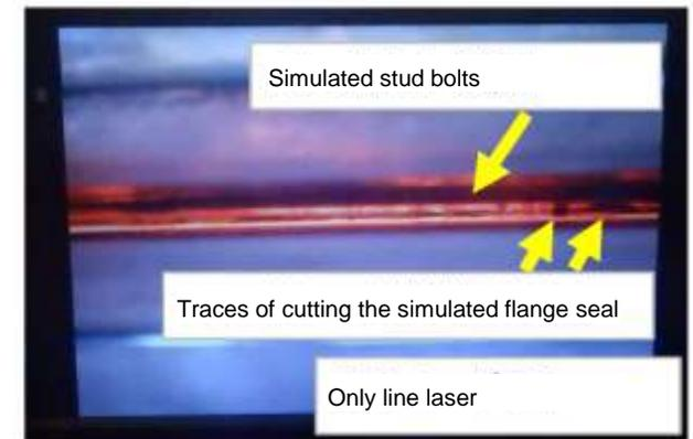
State of irradiating the line laser on the simulated bolts (after they are cut) during the preliminary tests
