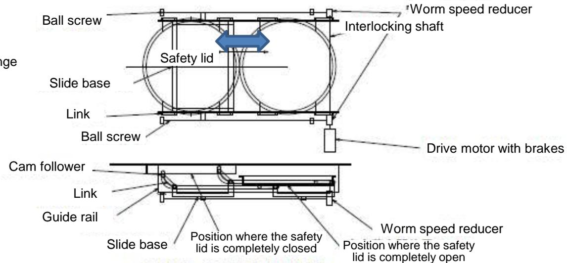
Part C (Safety lid opening/closing mechanism)
