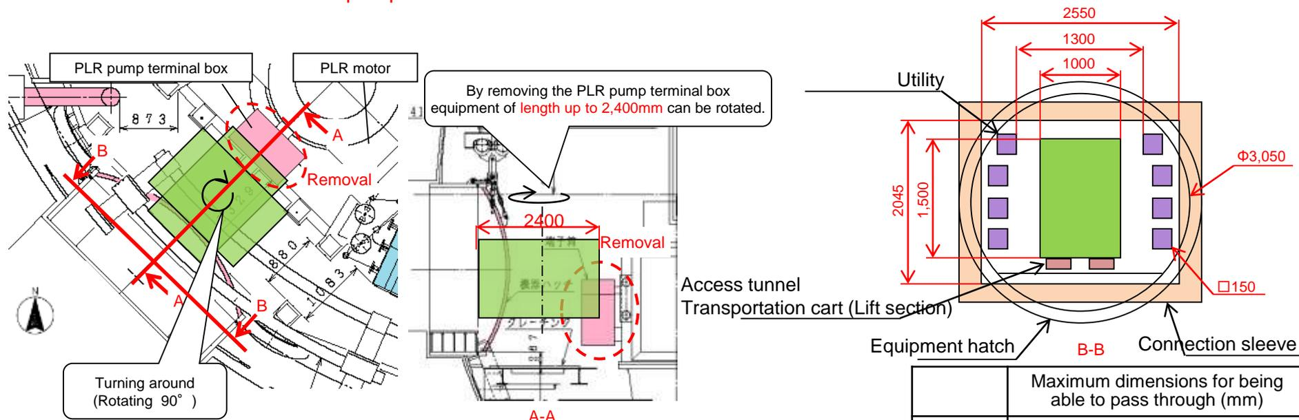
Results of the study on dimensions related to inserting the equipment inside the PCV
