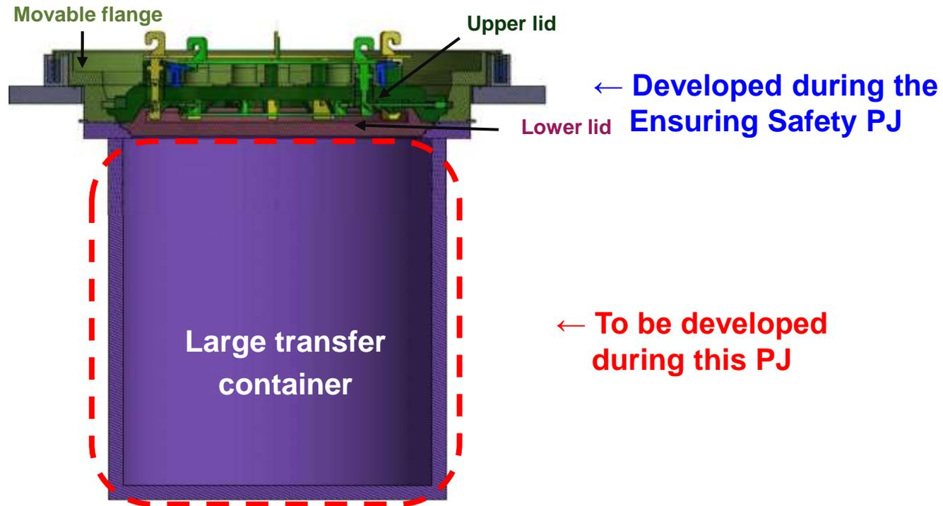
⇒ The structure of the main body of the large transfer container will be substantiated and the viability of the structure including the manufacturing capability will be studied. Air-tightness of the container body will be verified by test manufacturing the container.
