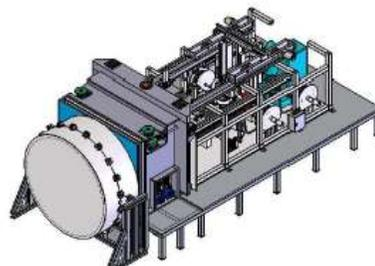
Illustration of PCV connection sleeve remote welding test (After equipment installation)
