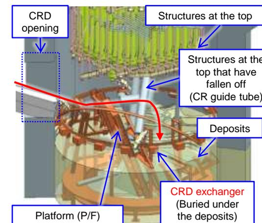
Figure illustrating the estimated conditions inside the pedestal (Units 1/3)
