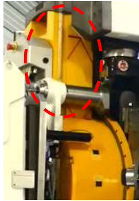
Photo 5 Connection test (opening/closing of shielding door)
