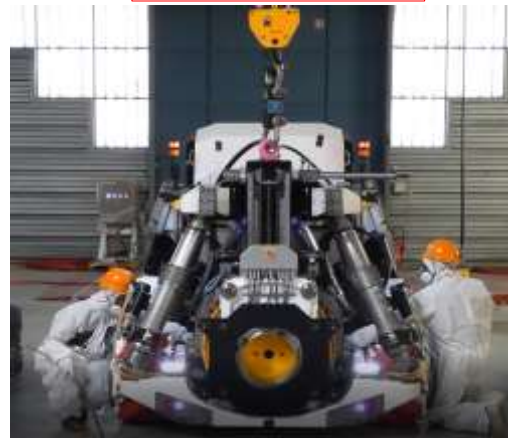
Setting the TPS + PADIRAC on to the cart
