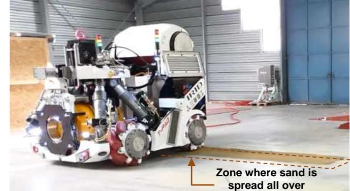
Photo 4 Traveling test (traveling over sand)
