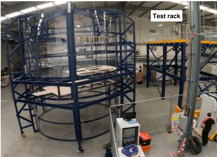
Simulated pedestal and test rack used in the in-factory verification test
