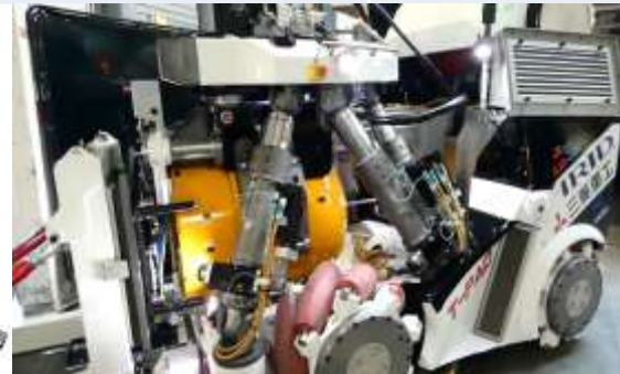
Photo 1 Hexapod positioning performance test
