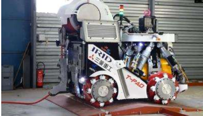
Photo 2 Traveling test (traveling over a slope)
