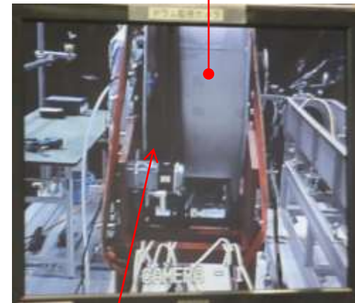
Number of windings of the remaining composite cable on the cable drum
