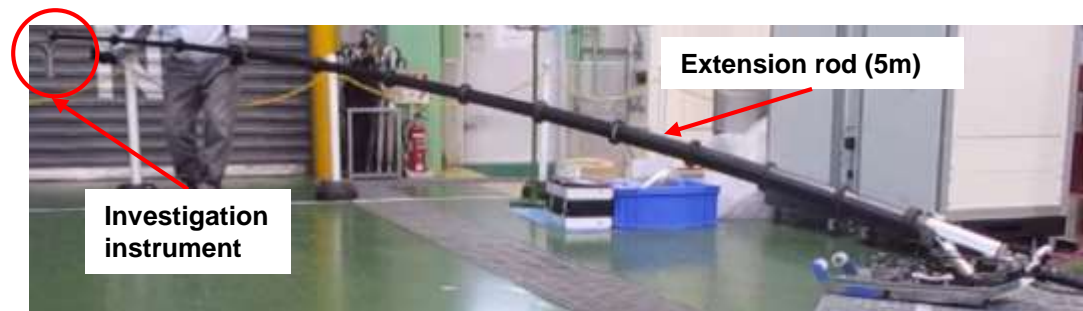
Figure 17: Equipment for investigating inside the pedestal
