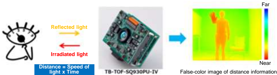
Figure 34: Measurement principle of the TOF depth camera
