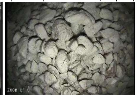
Photo [4] Zeolite (Endoscope: direct vision, near point)
