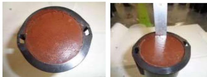
Fig. 3 Status on surface of solidified substance during segregation (example) (Water/solid ratio = 41 mass%, Waste filling rate = 35 mass%)
