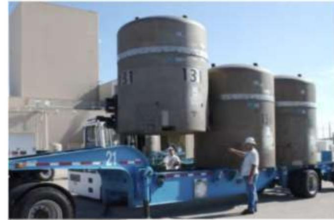
Figure 1. Example of a typical transport cask used for high-level radioactive wastes (TRUPACT-II)
