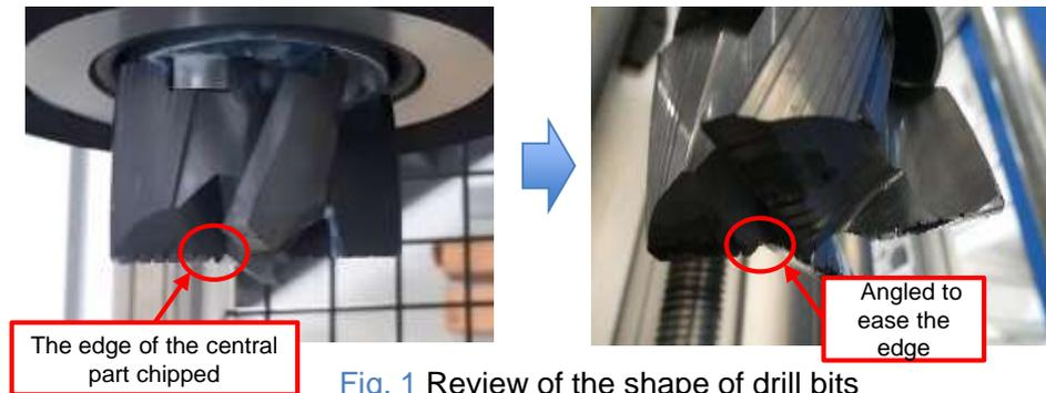
Fig. 1 Review of the shape of drill bits
