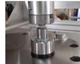
Closing plug being installed
