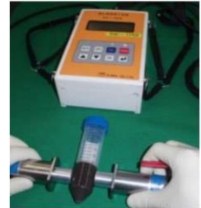
Fig. 3 State of ultrasonic measurement using a centrifuge tube
