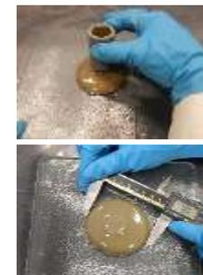
Fig. 4 Small flow test
