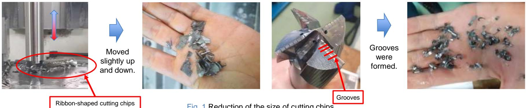
Fig. 1 Reduction of the size of cutting chips
