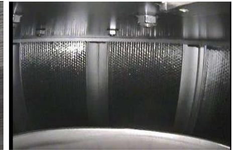
Photo [2] The sides of the simulated adsorption tower (Endoscope: lateral vision, far point)
