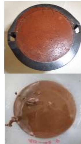
Fig. 2 Segregation state in  $\phi 5 \times 10$  cm container (top) and  $\phi 5.8 \times 8.5$  cm container (bottom)
