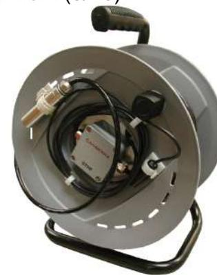
Fig. 1 Semiconductor detector (with Si diode)
