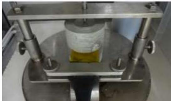
Fig. 1 Measurement using the Hot Disk method
