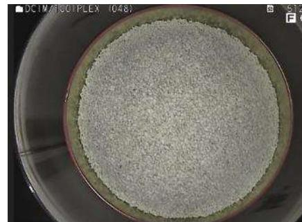
Photo [3] Zeolite (Endoscope: direct vision, far point)
