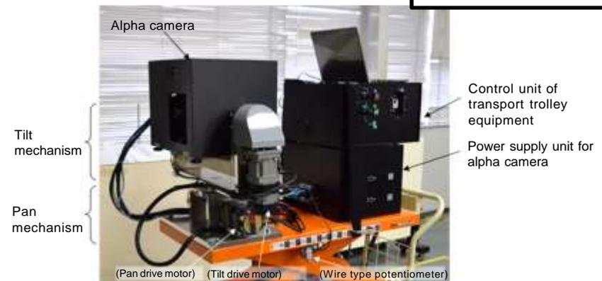
Fig. 2 Image of  $\alpha$  ray contamination measuring system
