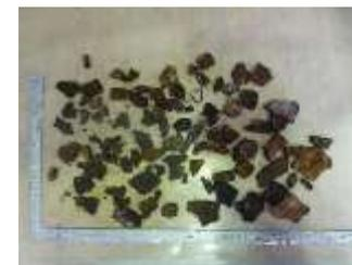
Fig. 2 Appearance of iron coprecipitation slurry dehydration product
