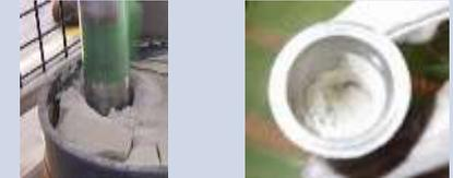
By drilling the solidified sample and taking in the sample from the collection port at the bottom, a target amount of the sample can be collected.
