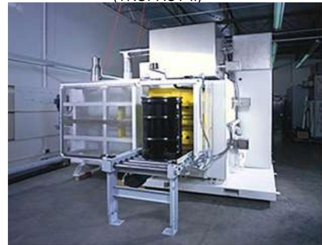
Figure 2. External appearance of a remote control filter vent attachment system (DVS: drum venting system)
