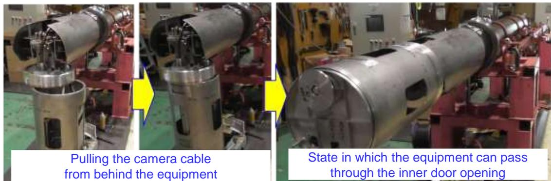
Verifying the transformation to a state in which the equipment can pass through the inner door opening when the gear is idling
