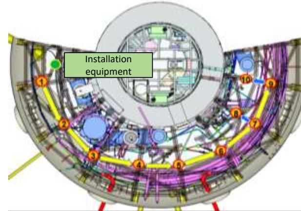
Figure Route for measurement of deposit thickness
