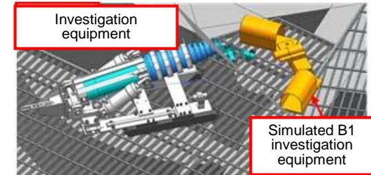
Figure 21 Crossing over the B1 equipment left behind
