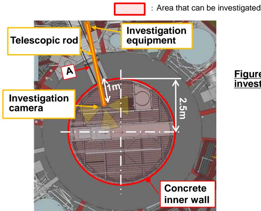
**Figure 11** Area that can be visually confirmed by the equipment for investigating inside the pedestal (horizontal)
