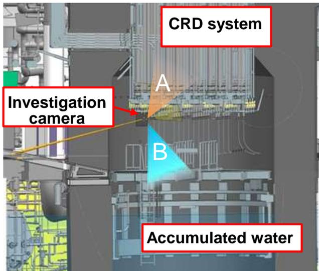
Figure 14 Capturing the image of the inside of the pedestal
