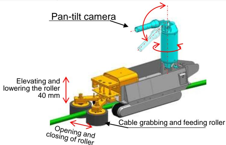
Figure 29 Cable feeding equipment
