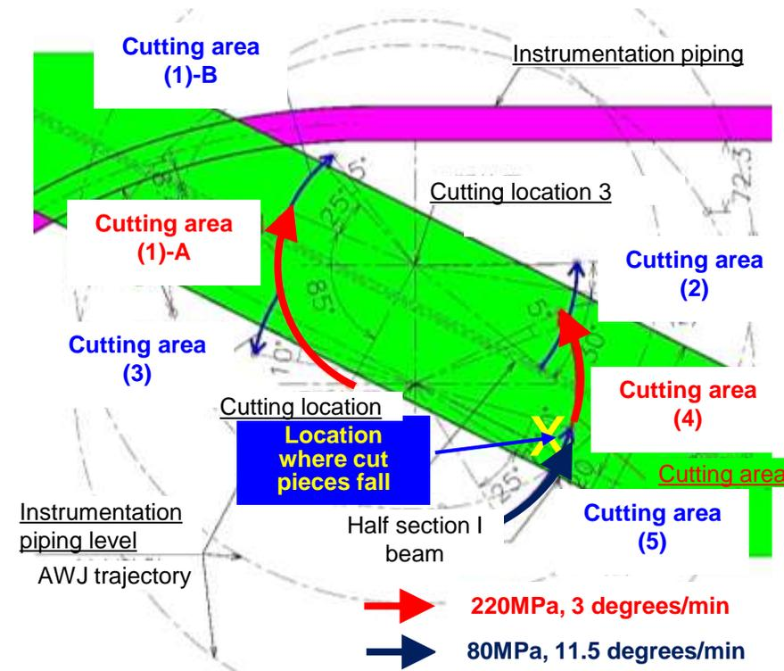
Location of cutting area and instrumentation piping (estimated)
