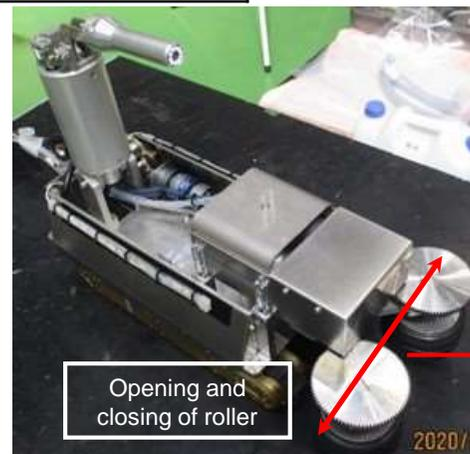
Figure 30 Cable feeding equipment: Prototype
