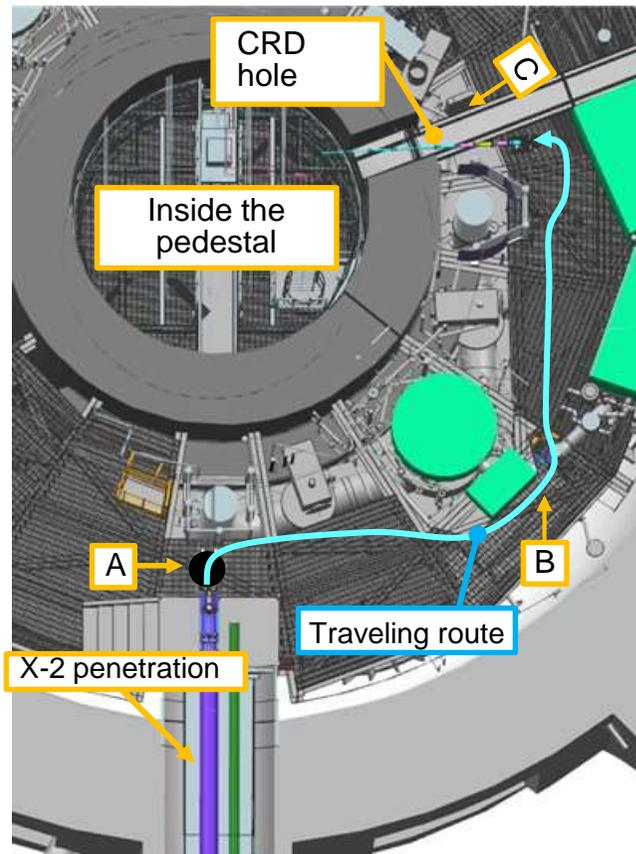
Figure 17 Assumed traveling route of the investigation equipment inside PCV
