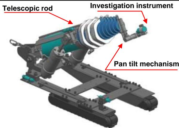
Figure 23 Equipment for investigating inside the pedestal
