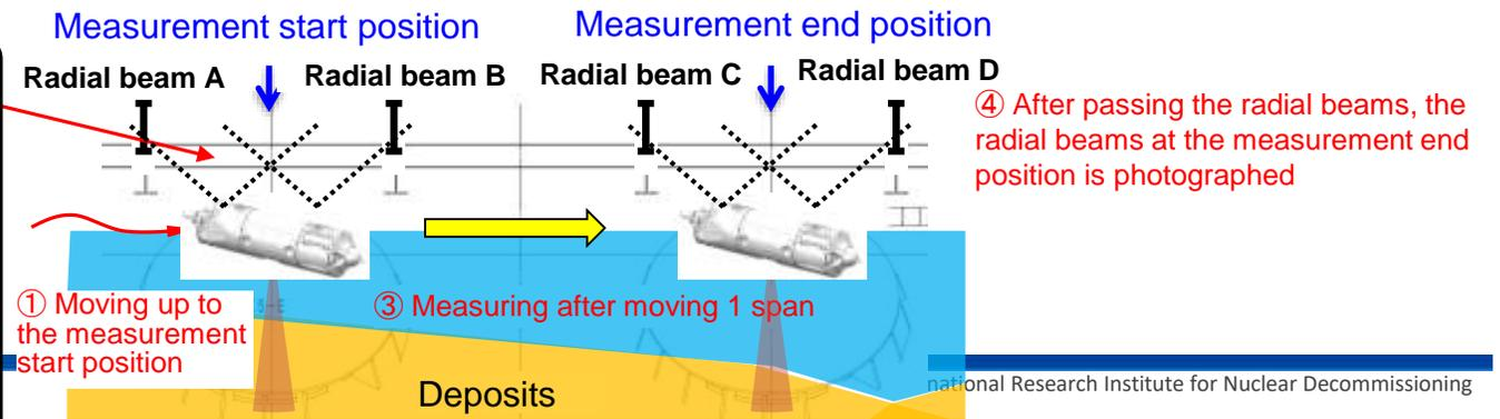
Figure Flow of measurement of deposit thickness
