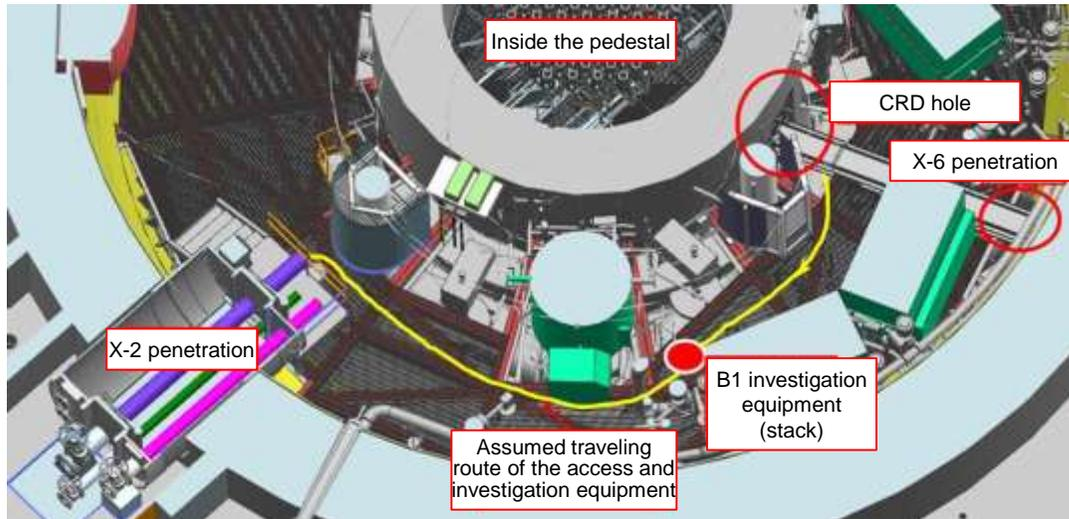
**Figure 1: Assumed traveling route of the access and investigation equipment inside PCV**
