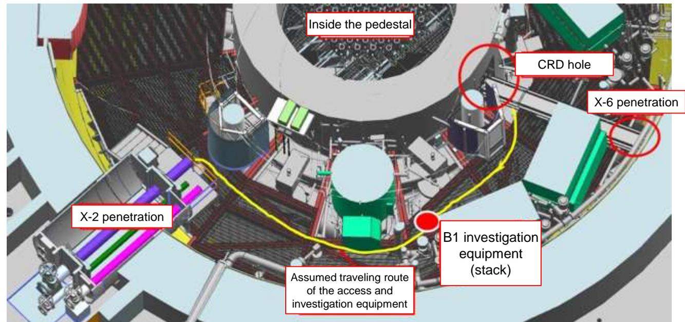
**Figure 4: Assumed traveling route of the access and investigation equipment inside PCV**
