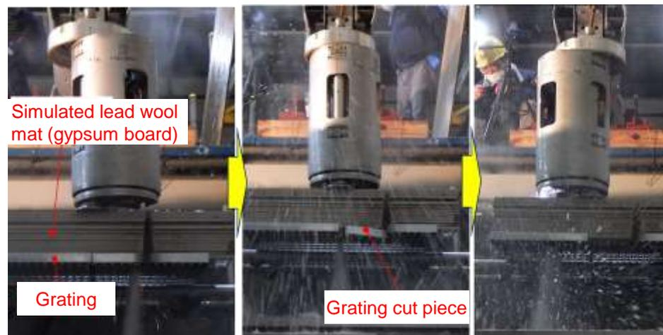
Verifying the ability to cut the grating underneath the lead wool mat
