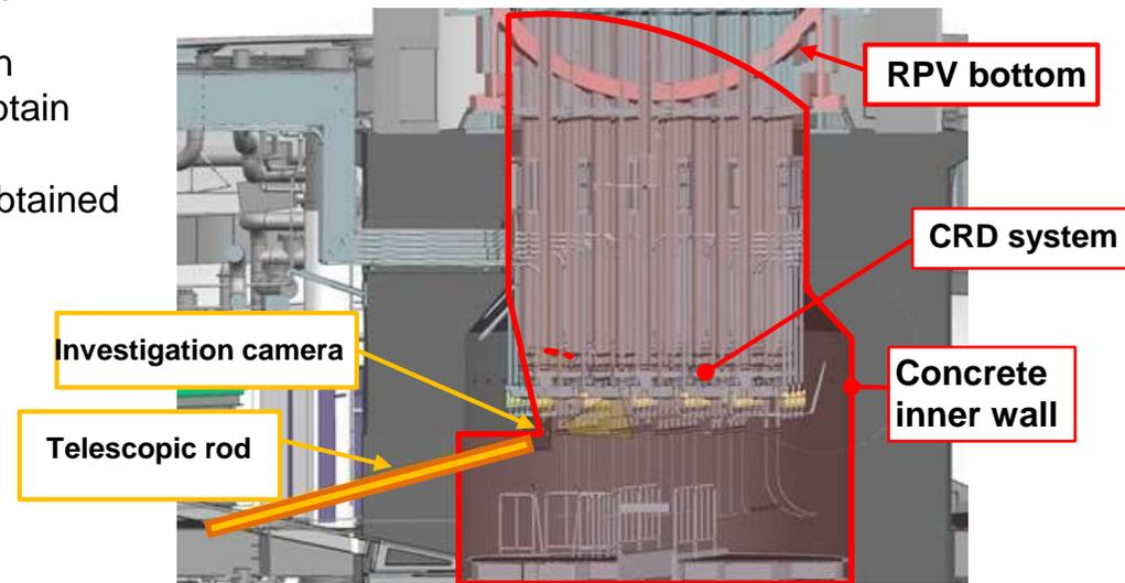
**Figure 12** Area that can be visually confirmed by the equipment for investigating inside the pedestal (A view / Upper part of the pedestal)
