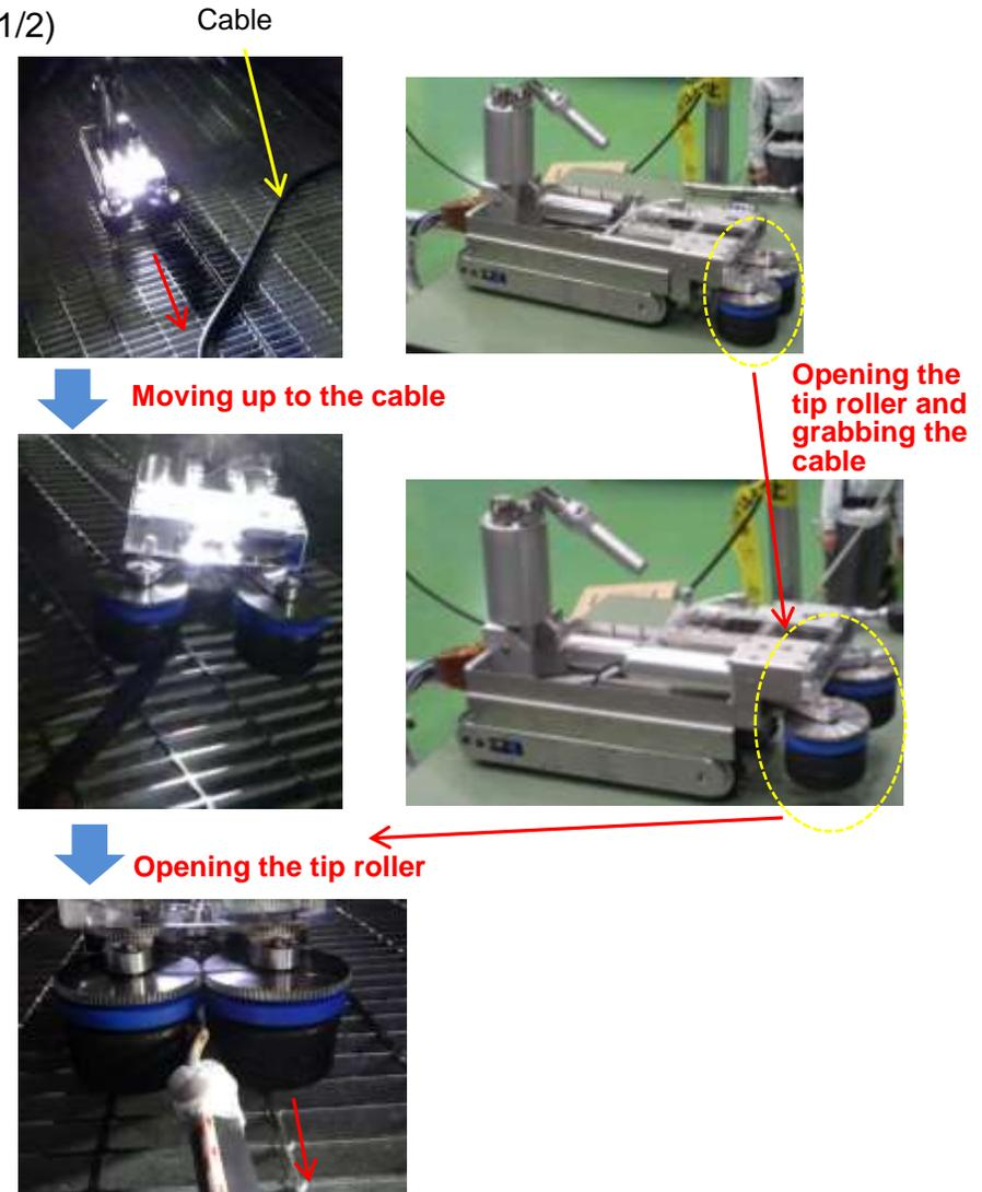
**Figure 37** Overview of the movement during cable feeding
