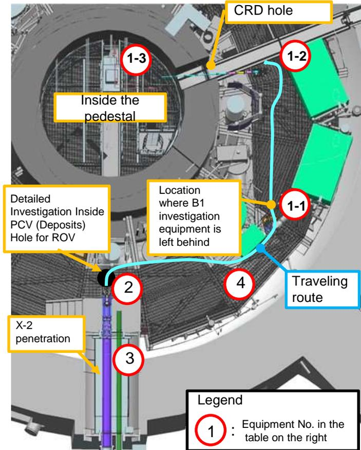
Figure 18 Assumed traveling route of the investigation equipment inside PCV
