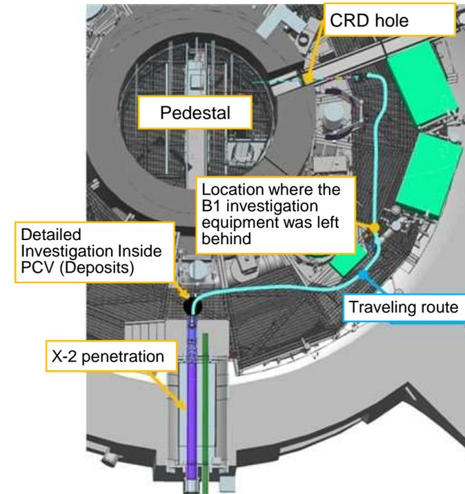
The investigation equipment was moved from the X-2 penetration to the CRD hole by means of remote automatic operation and the conditions inside the pedestal were investigated by means of the investigation instrument (camera) at the tip of the telescopic rod.
