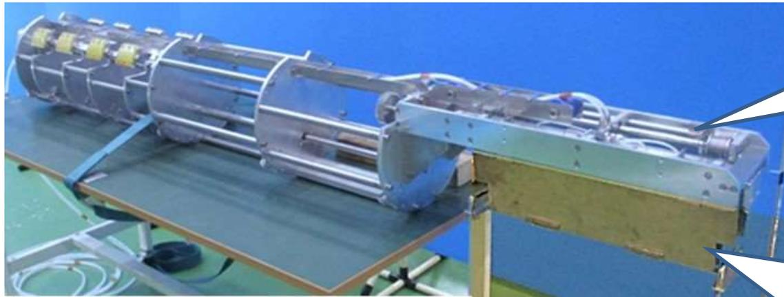
Figure 27 Hole cover installation equipment prototype
