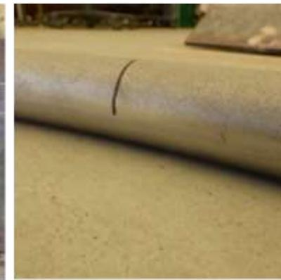
External appearance of the simulated PLR instrumentation piping after the test
