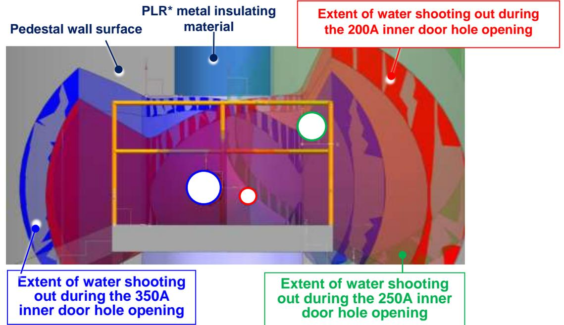
Schematic diagram of the extent of water shooting out from the AWJ during the inner door hole opening
