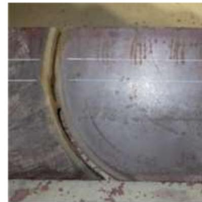
Half section I beam test piece (after cutting area (1))
