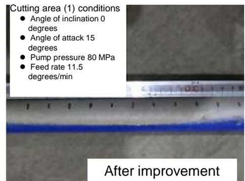
Example of verification of wall thinning of the simulated PLP instrumentation piping at the time of cutting the half section I beam flange surface
