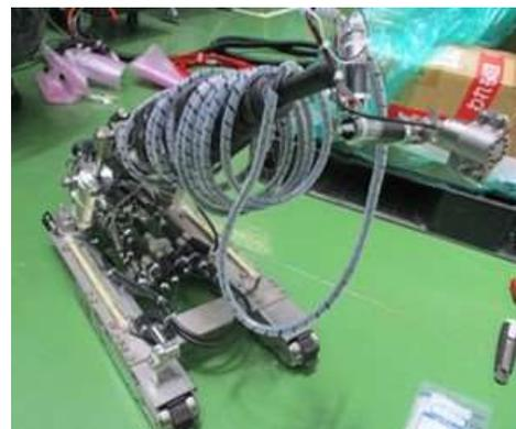
Figure 24 Equipment for investigating inside the pedestal (Prototype)
