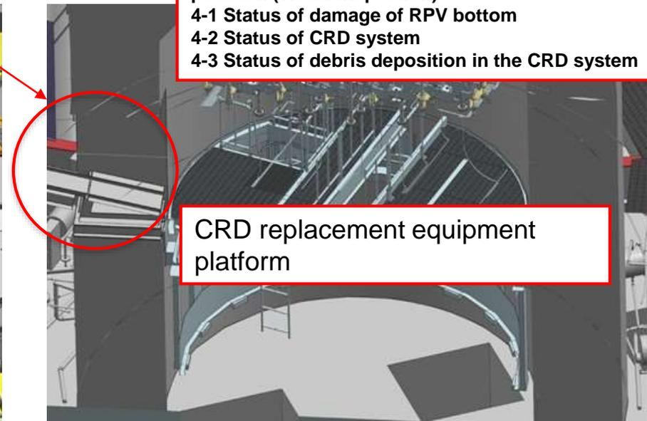
Figure 10 Structures inside the pedestal (Example) (2/2)
