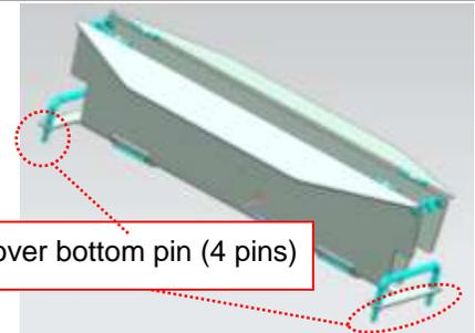
It was confirmed that the cover does not slip even if equipment travel on it since the hole cover bottom pins (4 pins) are inserted in the groove of the grating.
