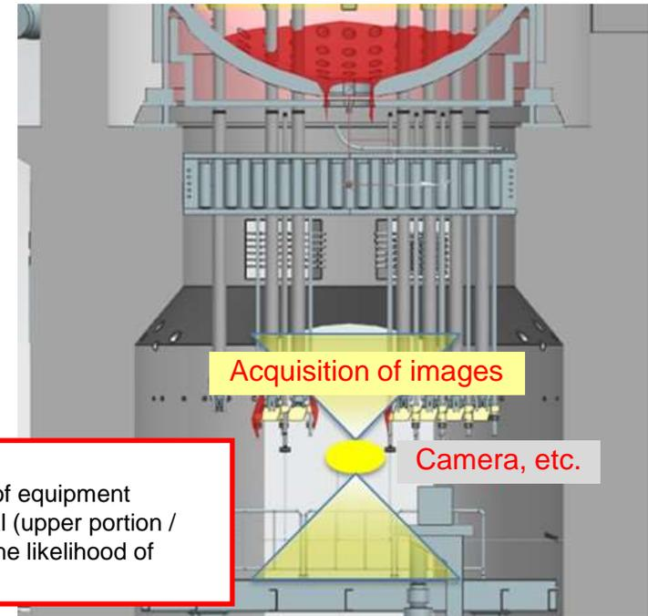
Figure 6 Secondary investigation (Inside the pedestal)
