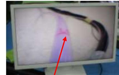
The tube is fed while checking the scale on the tube at any position by means of the image from the camera for checking the extension of the rod
