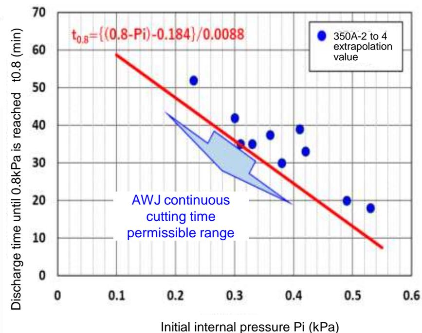
Figure-1 Method of setting the following timing for starting of cutting depending on the increase in dust level
