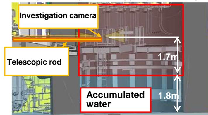
**Figure 13** Area that can be visually confirmed by the equipment for investigating inside the pedestal (A view / Lower part of the pedestal)
