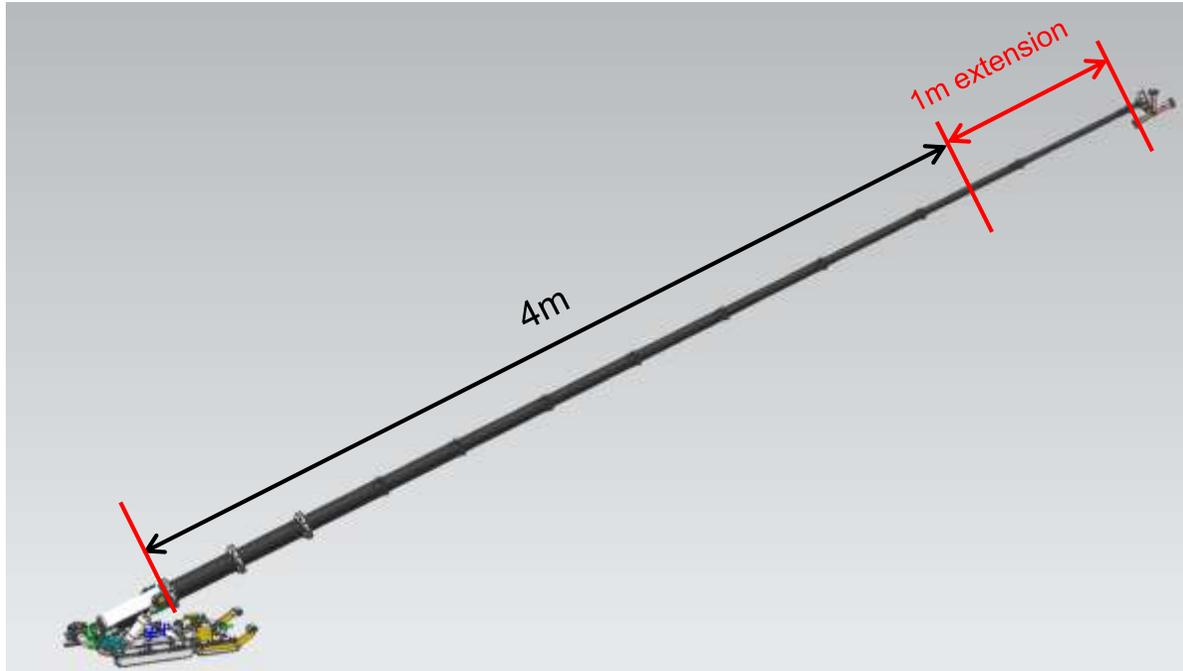
**Figure 31** Extension of the telescopic rod
