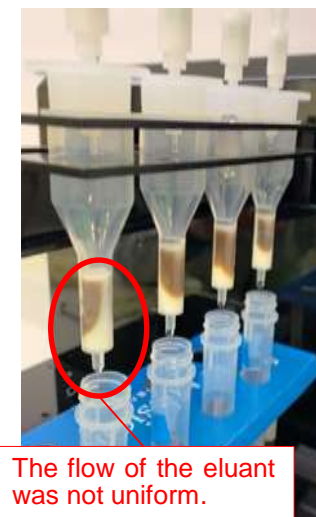
Fig.2 State of the column after the Mo elution operation
