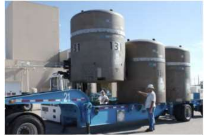
Fig. 1 Example of transport cask used for high-level radioactive waste (B type transport cask, USA: TRUPACT- II)
