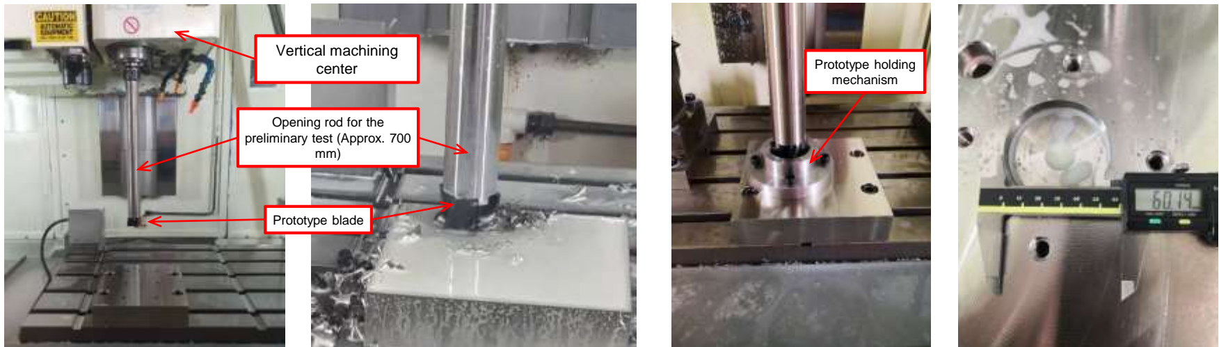
Preliminary test equipment for making openings
