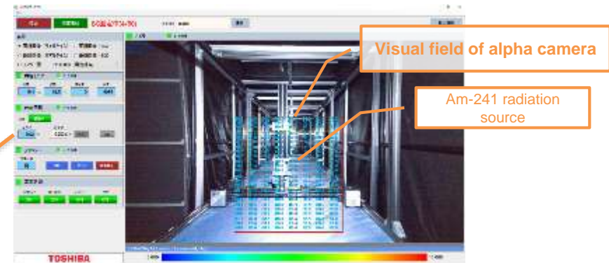
Fig. 2 Alpha camera software screen (During BG measurement)
