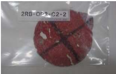
Fig. 2 External appearance of analytical sample (outer wall waterproofing material)
