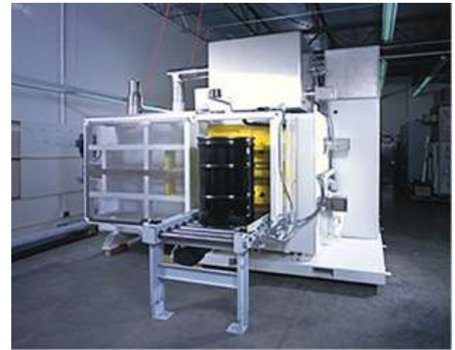
Fig. 2 Remote controlled type filter vent attachment device (DVS: Drum Venting System) External appearance (Used at the Waste Isolation Pilot Plant (WIPP) in Carlsbad)
