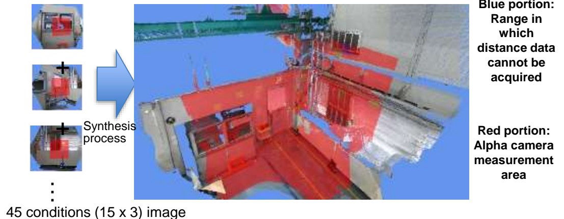
Fig. 2 Example of 3D synthesis of the photographic data of multiple locations
