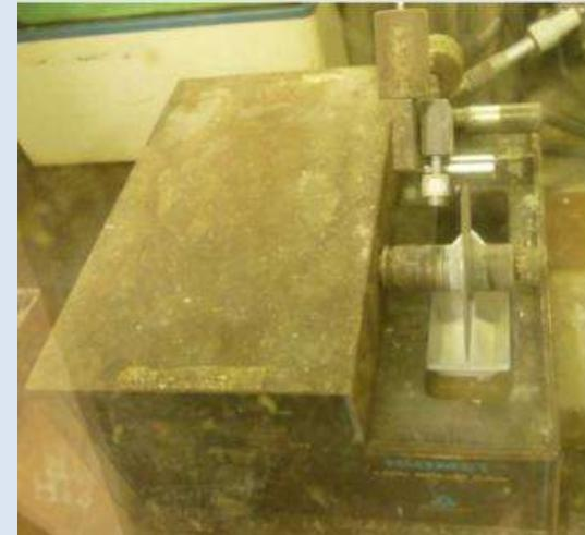
Low-speed cutting machine set up inside the glove box (Mechanical processing test)
