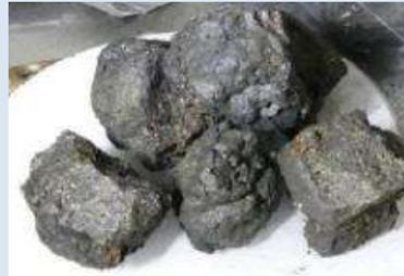
External appearance of the UO<sub>2</sub>\_In-vessel sample (No. 6)
