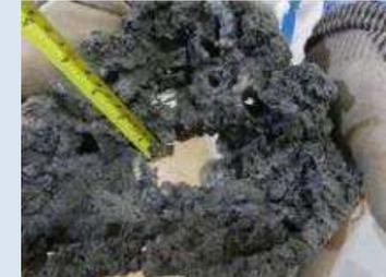
External appearance of the UO<sub>2</sub>\_In-vessel sample (No. 8)
