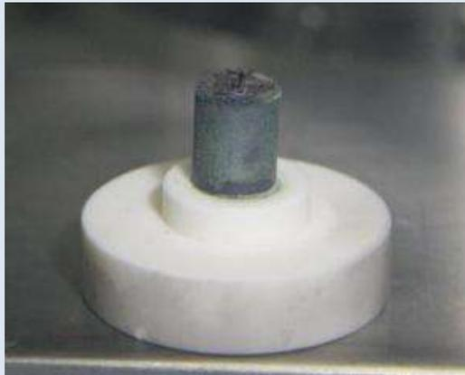
Produced (Pu, Zr) O<sub>2-x</sub> simulated debris
