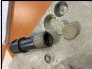
Performance test result of the above-mentioned cutting device (Test of cutting a  $ZrO_2$  block by a diamond-coated bit)
