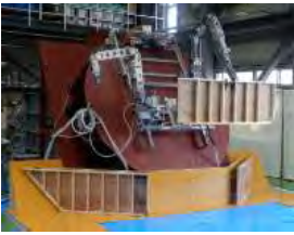
Equipment for preventing the spread of contamination into S/C
