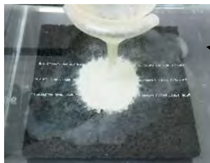
Figure 2 Water glass type absorber (viscous solidified)
