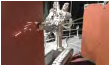
Flexible work arm (crawler, dual arm type)
