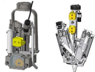
Collection device for chip powder and core (rock-like) debris
