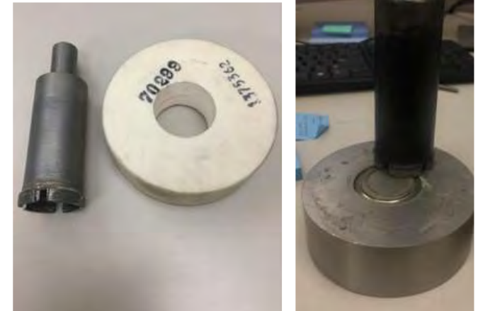
Ceramic (aluminum oxide) on left and metal (stainless steel) on right, both cut by diamond coating bits.
