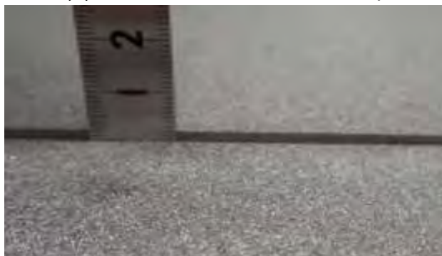
(d) Center level difference of joint of BSW mold (2 mm)
