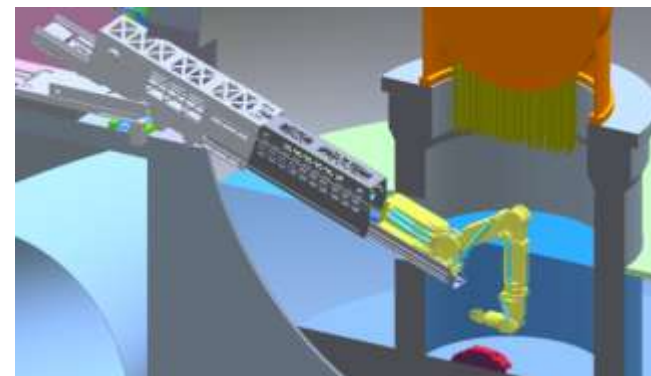
Fuel debris removal by a hydraulic robot arm
