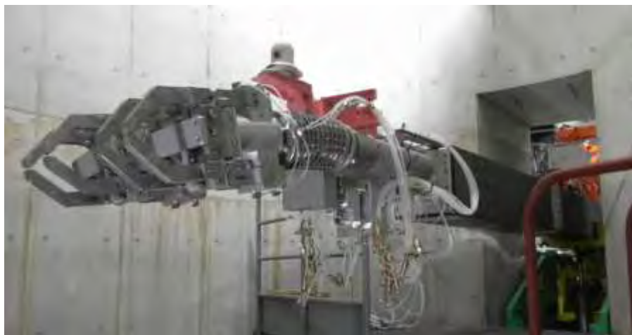
External appearance of the arm section of the interfering object removal device
