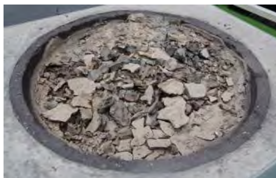
MCCI simulant after processing
