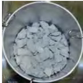
(a) Simulant size: 20 to 40 mm
