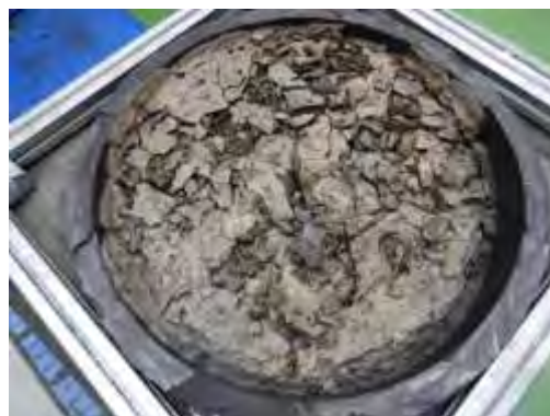
MCCI simulant after processing
