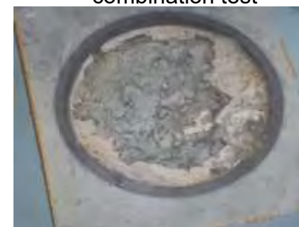
MCCI simulant after processing
