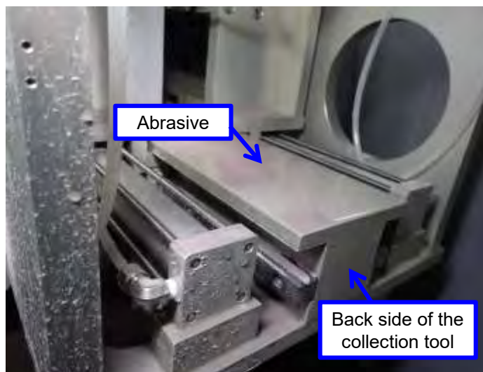
Deposit in the collection tool driving mechanism
