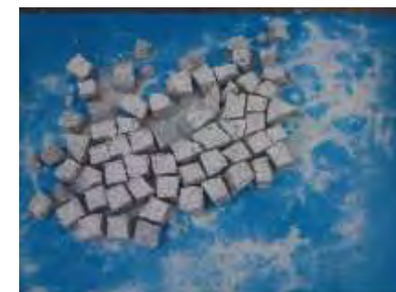
Granite after crushed (cubes of 50 mm or smaller)
