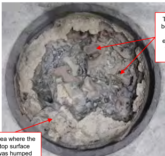
MCCI simulant after broken pieces were removed
