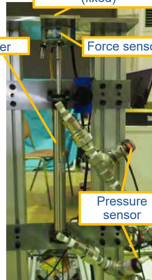
Single axis hydraulic cylinder test equipment
