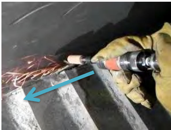
Step 1. Tilt the tool and run it across the edge three times
