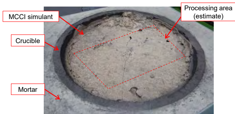
MCCI simulant before processing
