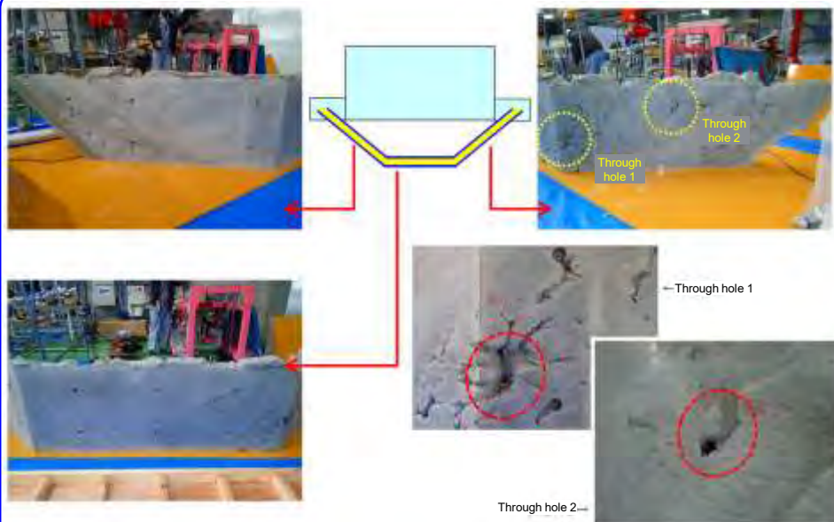
Dike after mold was removed (outside)
