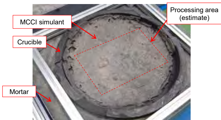
MCCI simulant before processing
