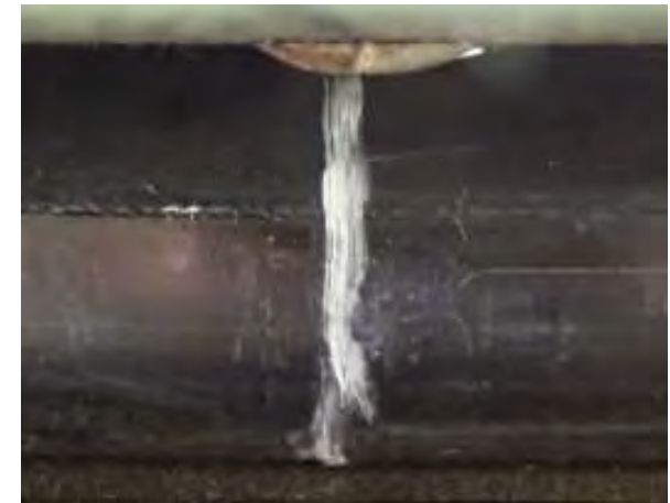
(c) Internal pressure of seal 0.08 MPa
