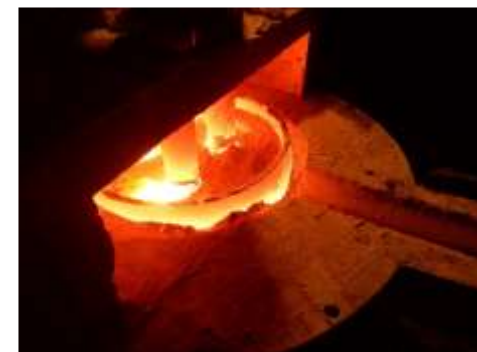
Molten pool when final samples are put inside
