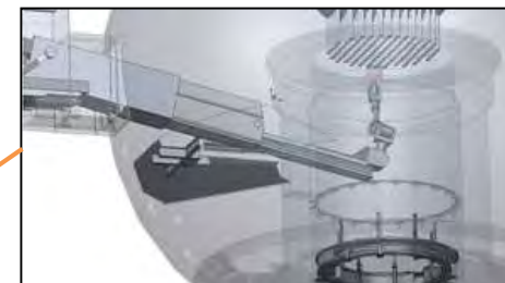
Verification of the maneuverability of a combination of a robot arm and access rail
