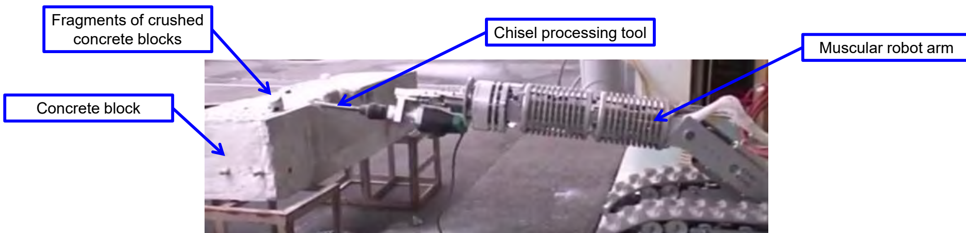
Crushing a concrete block using the chisel processing method
