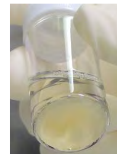
Figure 2. Non-dissolved residues of cerium oxide adsorbent
