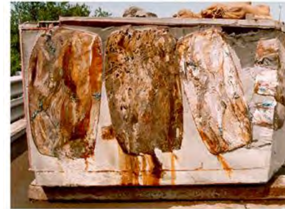
Cut cross-section of a container containing a compressed drum
