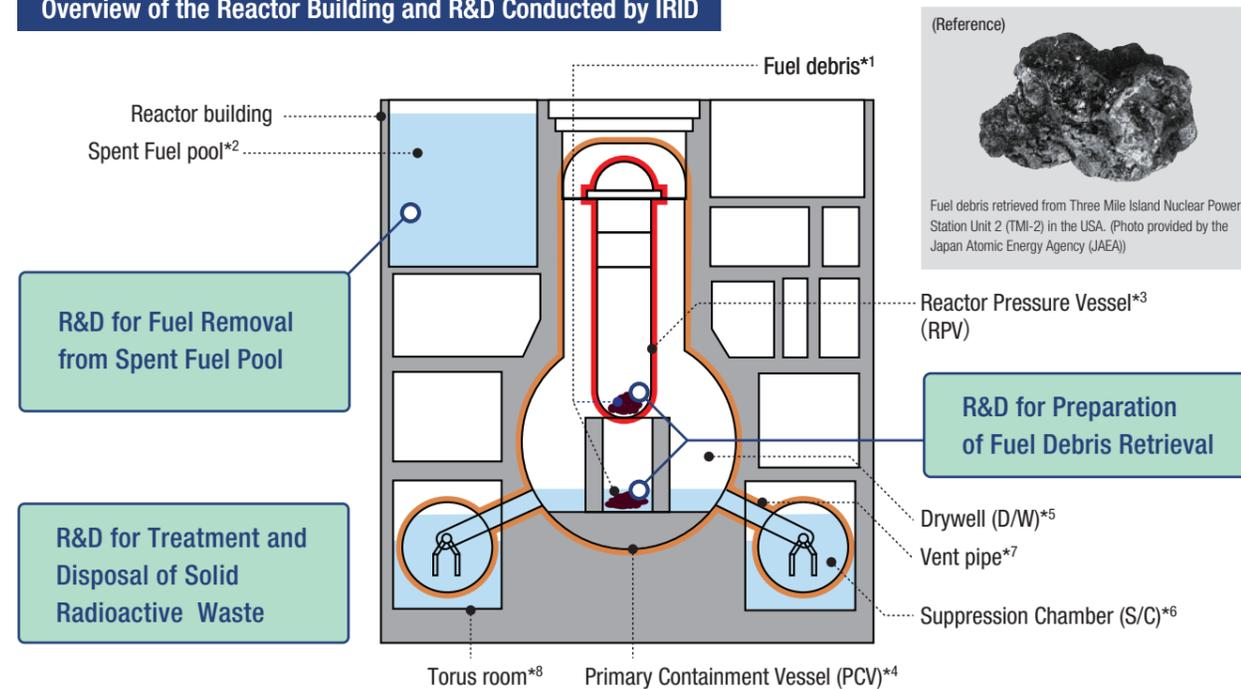
\*1 **Fuel debris:** Lava-like fuel containing material that is produced under high temperatures through melting with control rods and structures inside the RPV, after which it cools and re-solidifies.
