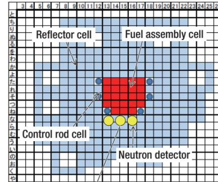
Example of test reactor core
