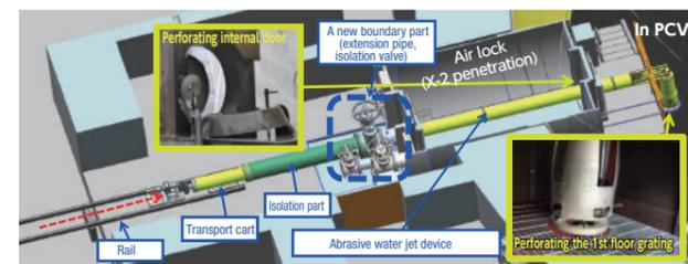
A new boundary part of X-2 penetration and perforating the grating
