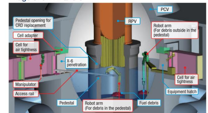
Note) Those in the red frames are new equipment. \*Position of X-6 penetration of unit 1 is different from those of unit 2&3.
