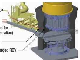
Penetration hole of PCV used for the investigation (X-53 penetration)
