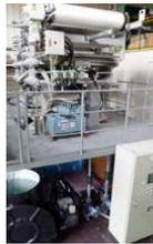
Pressure filtering test device to examine dehydration treatment of ALPS slurry
