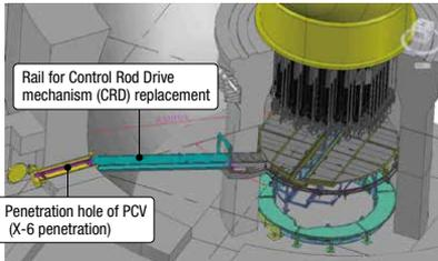
Rail for Control Rod Drive mechanism (CRD) replacement
