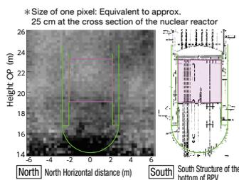
An image of high density substance thought to be fuel debris is confirmed on the bottom of the RPV. \*The measurement at unit 2 was conducted by TEPCO Holdings as a part of the IRID activities.
