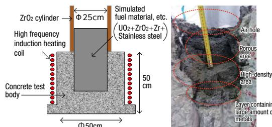
Large MCCI test apparatus in cooperation with CEA and its test product generated in MCCI test
