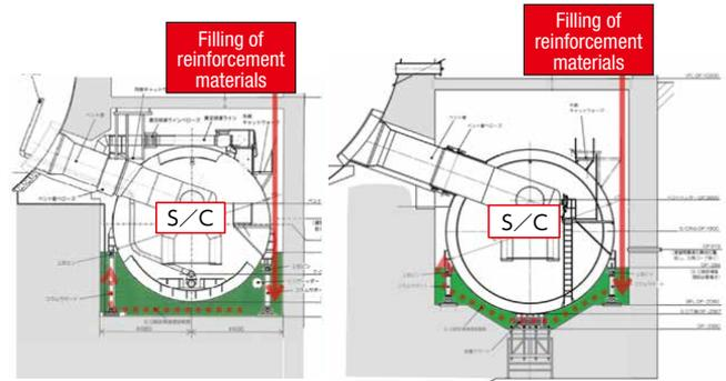
[Candidate material] Underwater inseparable mortar
