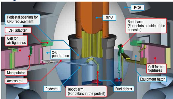
Note) Those in the red frames are new equipment. \*Position of X-6 penetration of unit 1 is different from those of unit 2&3.
