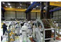
Implementation of reinforcing workability verification test for S/C support columns
