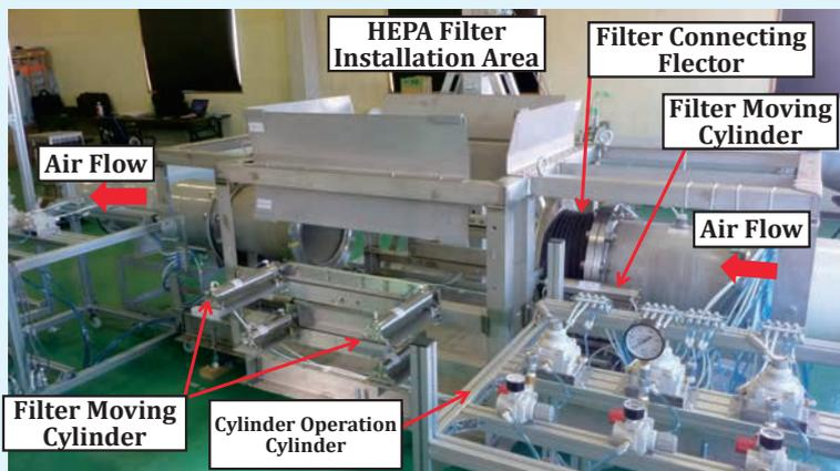
Fig. 5: Example of Collection and Removal Test Testing Device for Remote replacement HEPA
