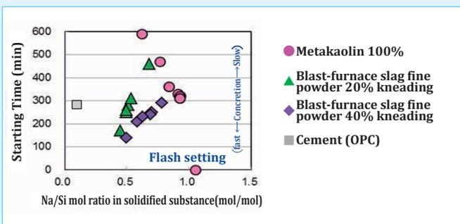
**Fig. 2: Relationship between Composition and Concretion Time**
