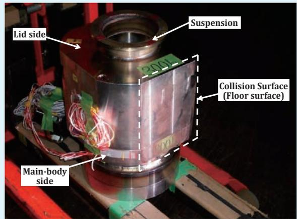
**Fig. 2: Example of Simulated Lid after Test**
