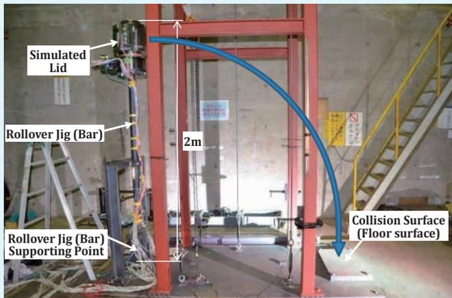
**Fig. 1: Appearance of Test Device**
