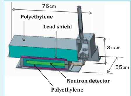
**Fig. 2: Design Concept of Neutron Detection Unit**
