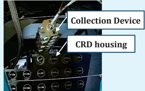
Fig. 3: Partial Submersion Side Access Method: Element Test of Interfering Object Removal
