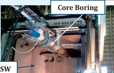
Fig. 2: Partial Submersion Side Access Method: Element Test of Biological Shielding Wall (BSW) Removal
