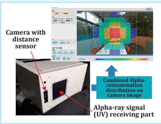
**Fig. 4: Surface Alpha Contamination Measurement Device (Alpha Camera)**
