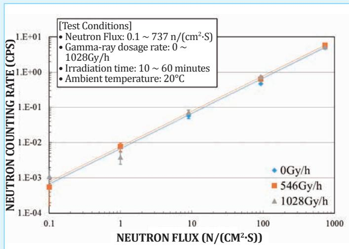
Fig. 4: Neutron Flux Detection Performance (under radiation environment)
