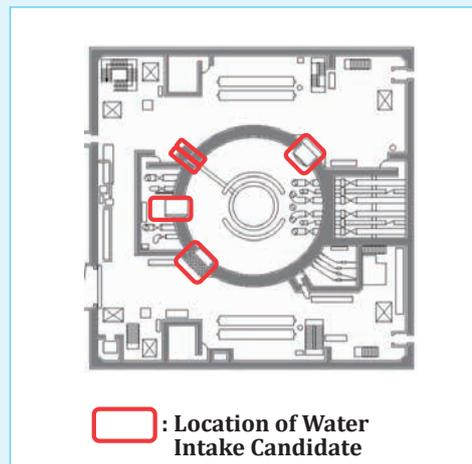
Fig. 2: Selection Result of the D/W Intake Candidate Penetration (Example: Unit 3)
