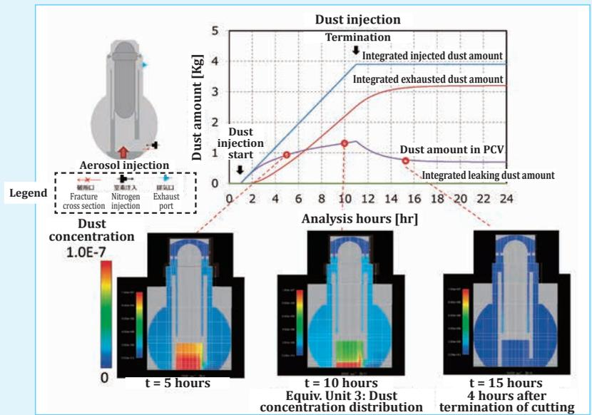
Fig. 1: Example of Technology Development of Confinement Functions (Dust spreading prediction)
