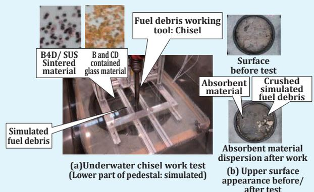
**Fig. 6: Insoluble Absorbing Material Injection and Crushing Test for Fuel Debris**
