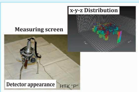
**Fig. 5: Example of Investigation Results of Penetration Alpha Contamination Measurement Technology: Detector appearance and image of measured results**
