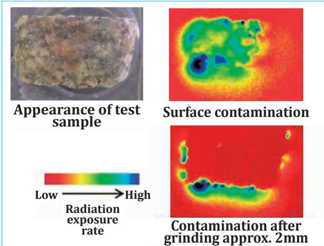
Fig. 1: Appearance of Locally Inhomogeneous Contaminated Rubbles (by imaging plate measurement)
