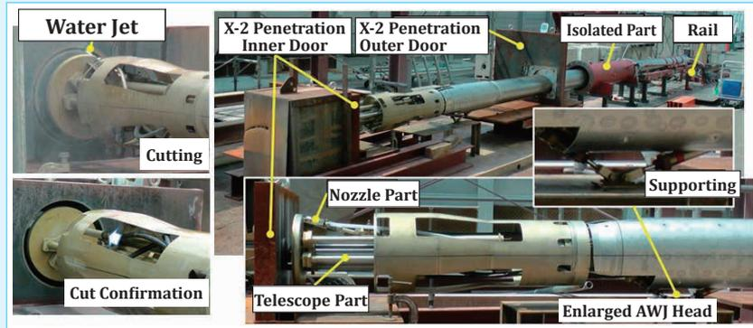
Fig. 2: In-plant Validation Status of Opening Hole in X-2 Penetration Inner Door
