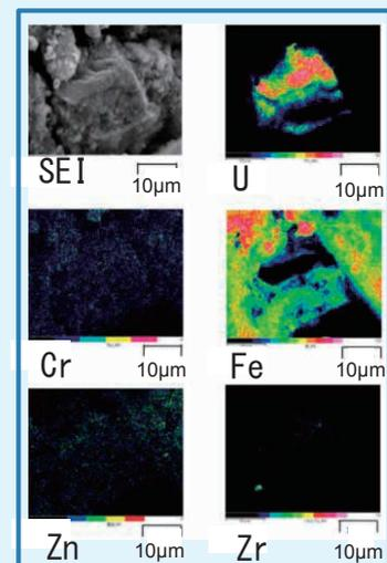
**Fig. 2: Wiping Deposits (photo in the center) and Analysis Result by Field Emission Type Electron Scanning Microscope (Figure in right)**
