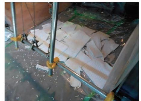
**Photo 1: Appearance of Crushing Test by Simulated Dehydration Products**
