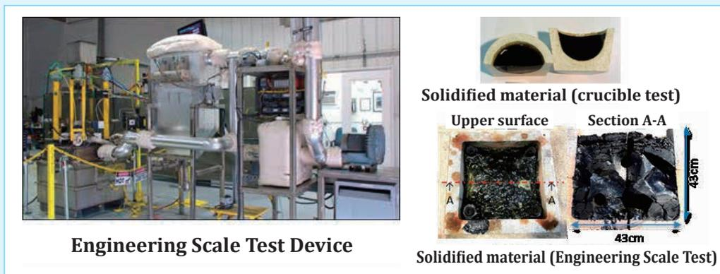
Fig. 4: Test Facility of In-Drum Type Glass Solidification Technology and Solidified Materials
