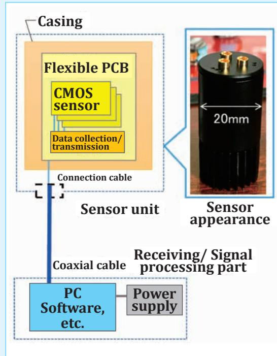
Fig. 2: Overview of CMOS Type Neutron Detection System
