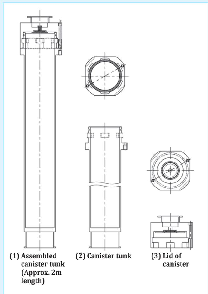
**Fig. 5: Basic Plan of Canister Shape**
