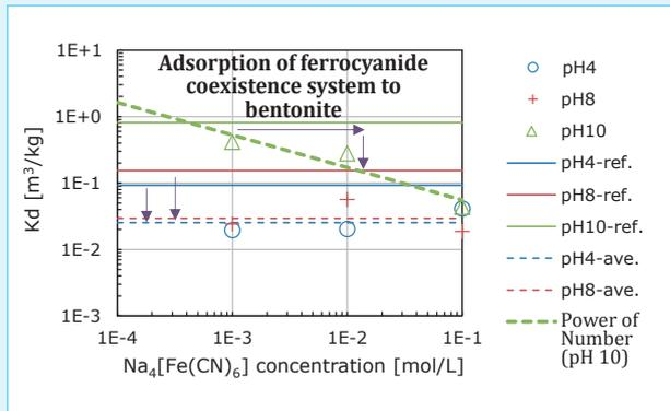
**Fig. 3: Evaluation Example of Adsorption Decreasing Factor for Artificial Barriers**
