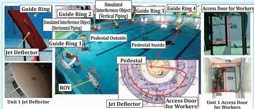
Fig. 3: In-plant Validation Status of Submersible Type Access Device
