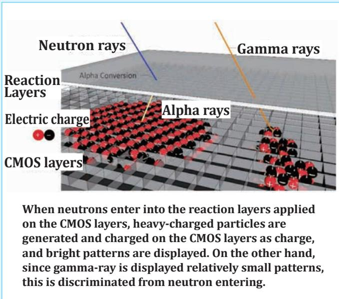
Fig. 1: Principle of CMOS Type Neutron Detector
