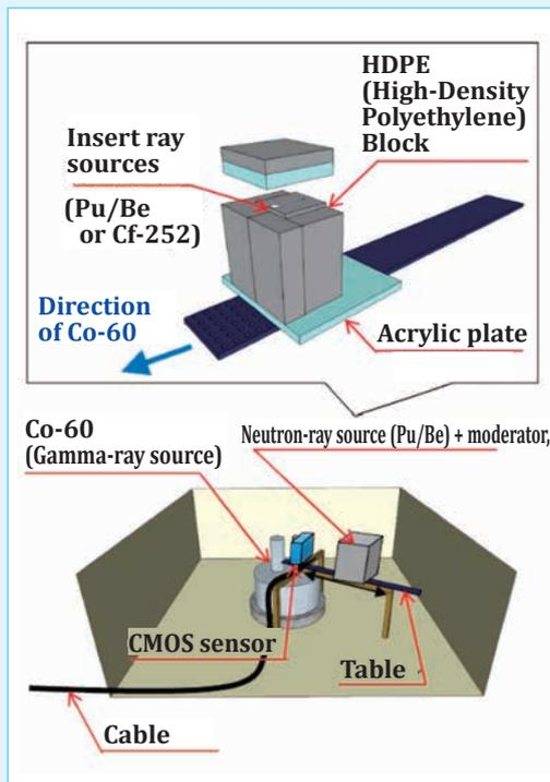
Fig. 3: Mockup System of Element Test
