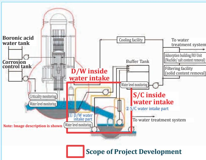
Fig. 1: Water Circulation System during Fuel Debris Retrieval
