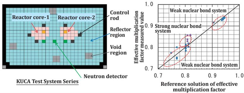
**Fig. 1: Subcriticality Measurement Test and Measured Results of Kyoto University Critical Assembly (KUCA)**
