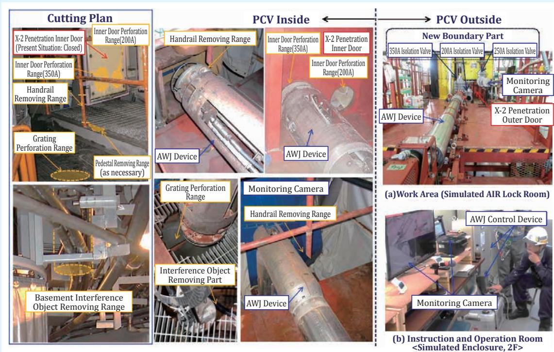
**Fig. 1: Status of AWJ Mockup Test for 350A**
