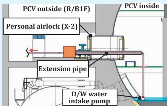
A used penetration part will be selected as the D/W water intake port depending on requirements of the water circulation system layout. This figure shows the example of the airlock for staffs (X-2) as a water intake port.
