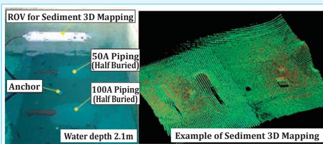
Fig. 5: Status of Compatibility Validation for measurement of Deposits 3D Shape
