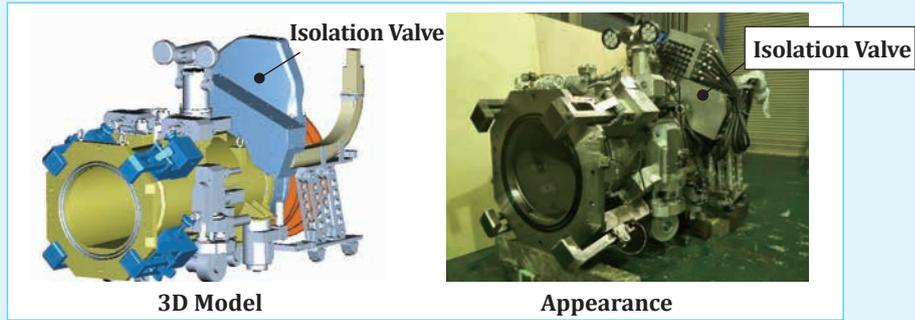
Fig. 1: X-6 Penetration Connection Structure
