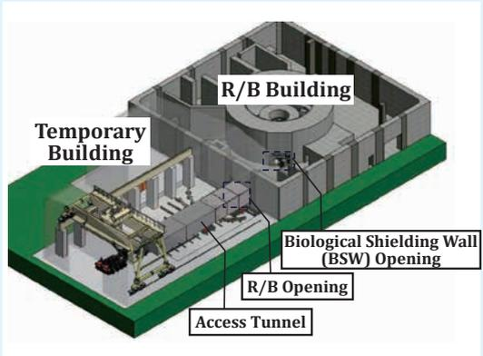
Fig. 2: Access Tunnel Installation Method
