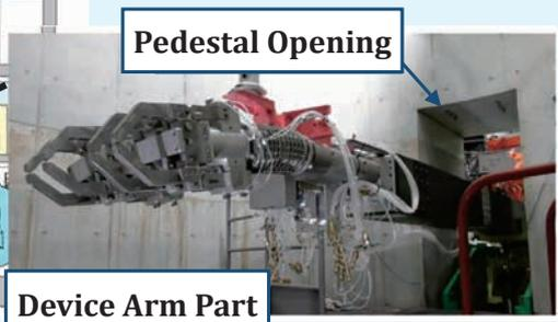
Fig. 4: Partial Submersion Side Access Process Method: Element Test of Interfering Object Removal
