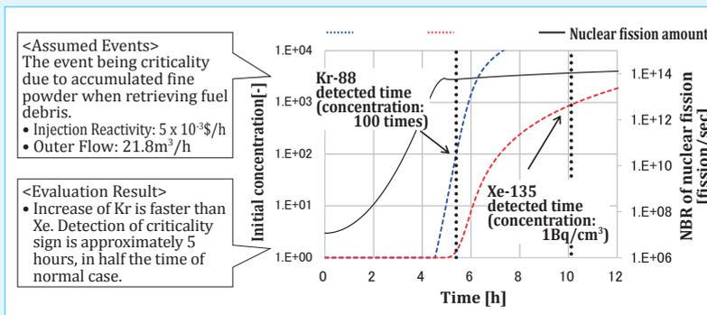
**Fig. 3: Evaluation Result of Criticality Detection Performance in case of Criticality Event (Example of Minor Criticality due to Fine Powder Accumulation)**
