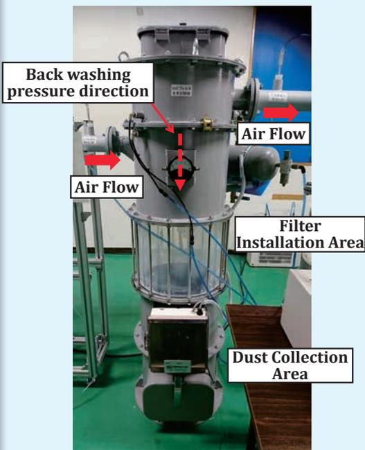
Fig. 4: Example of Collection and Removal Test Back washing Filter Testing Device
