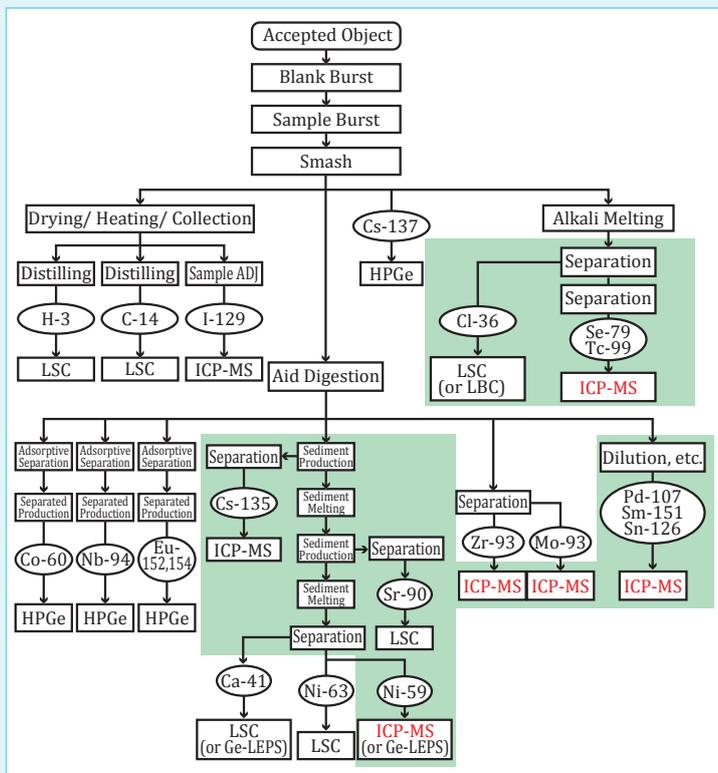
**Fig. 6: Developed Analysis Process**
