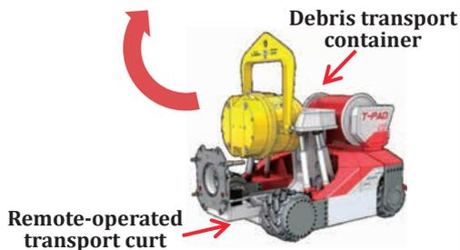
**Fig. 3: Debris Remote Transportation System**
