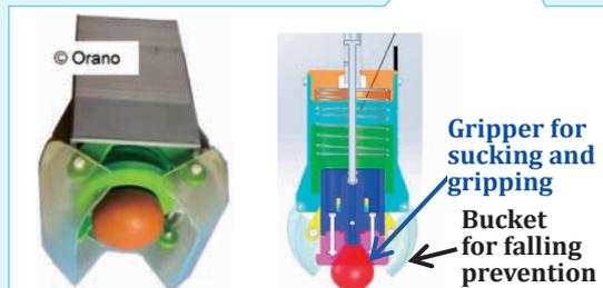
**Fig. 4: Concept of Pebble-like and Sand Shape Debris Collection Device**
