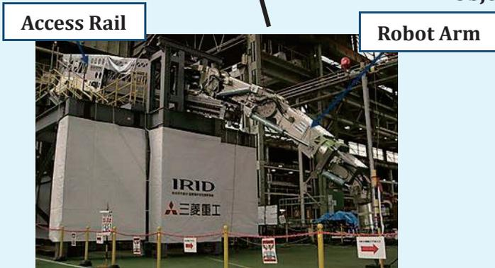
Fig. 5: Partial Submersion Side Access Method: Element Test for Combination of Robot Arm and Access Rail
