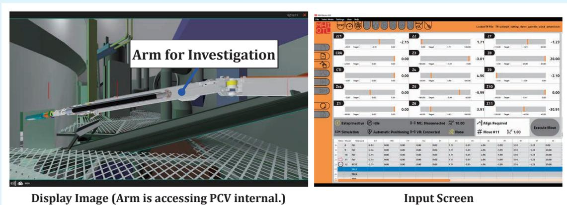
**Fig. 1: VR System for Access and Investigation Device**
