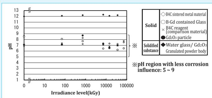
**Fig. 5: Test Result for Water Quality Impact Evaluation by Long-term Irradiation of Insoluble Absorbing Materials**
