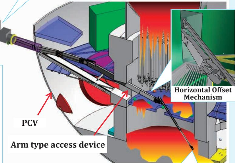
**Fig. 1: Concept of Fuel Debris Sampling in PCV**
