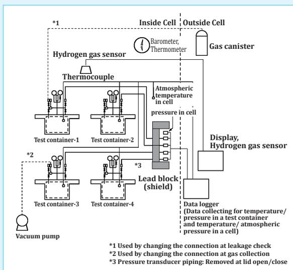
**Fig. 4: Test Device Configuration**
