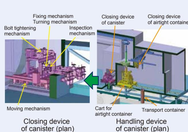
Fig. 7: Handling device of fuel debris canister (Image)
