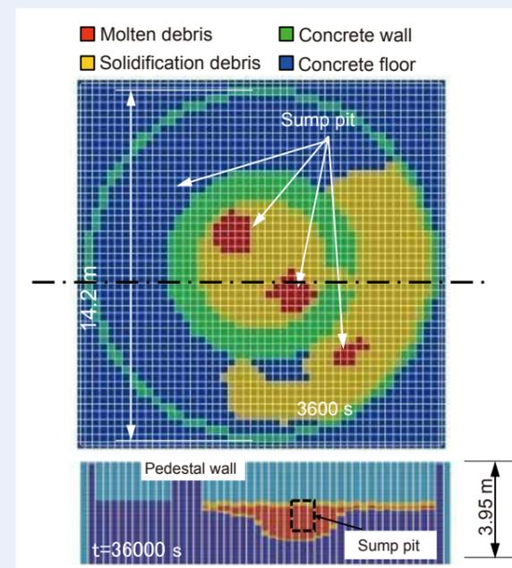
Fig. 3: Example of Fuel debris behavior evaluation in PCV (Unit 1)
