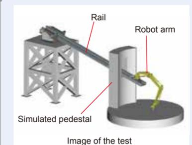
Fig. 5: Mock-up test facility for the access device inside the pedestal and test condition (Image)
