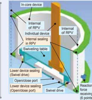
Fig. 2: Conceptual diagram of the access device inside RPV (In-core device)
