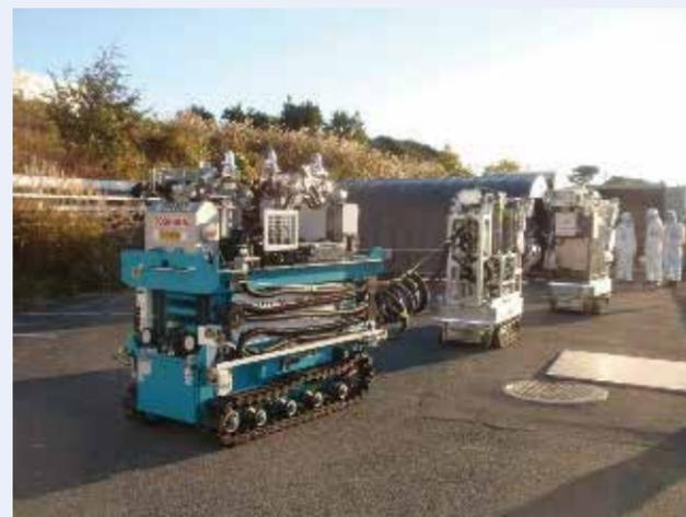
Photo 1: Scene of a combination test for the decontamination equipment for high places and low places
