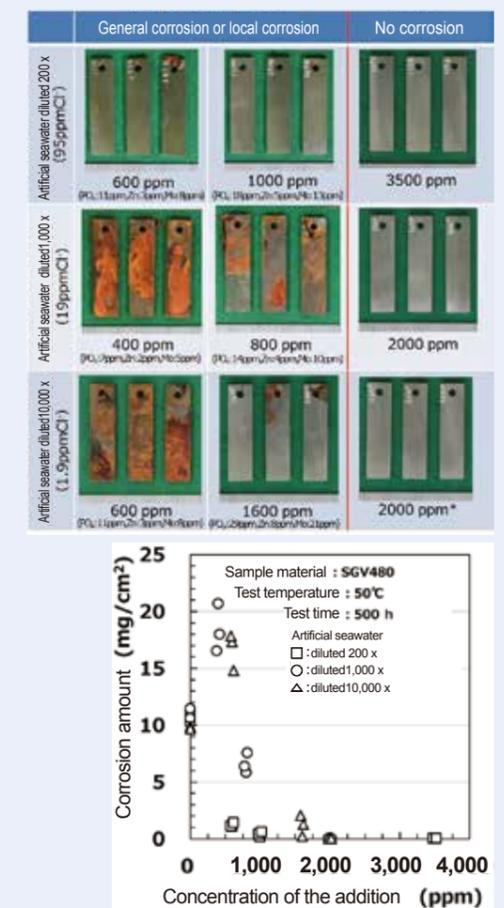
Fig. 2 Example of validation test for anti-corrosion effects of rust-preventive agents (Test result of adding zinc / sodium molybdate mixing phosphate)
