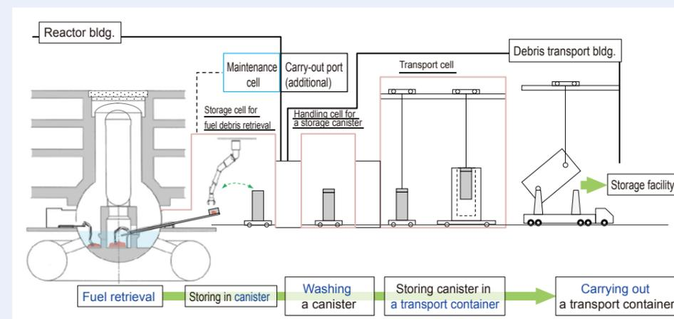
Fig. 5: Flow chart for the collection, transfer and storage for a storage canister (Fig. shows non-submerged from side method from the side of the reactor.)
