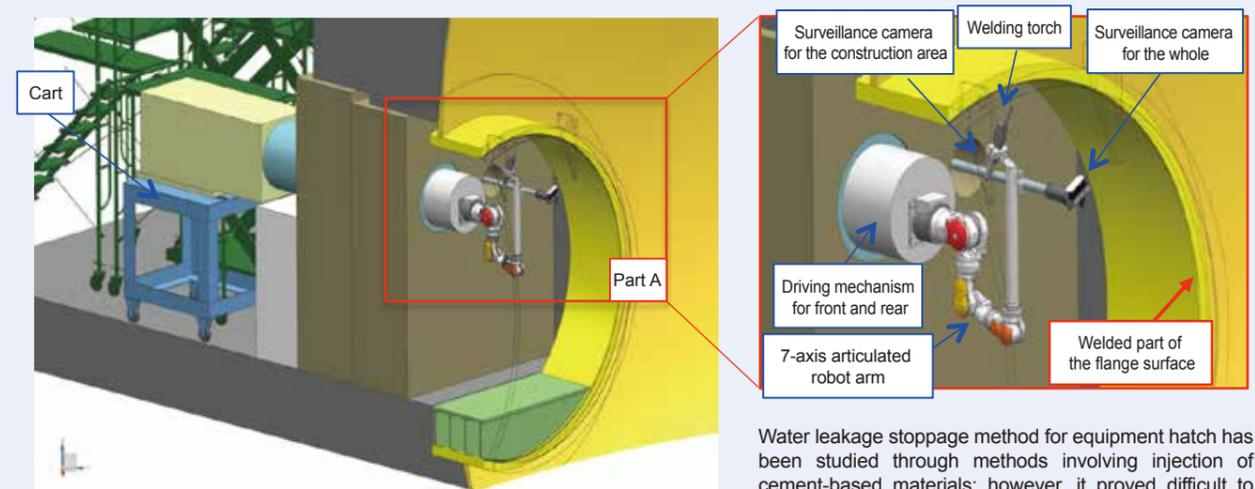
Fig. 5: Water leakage stoppage technology for the sealing parts (water stoppage for the equipment hatch)
