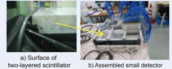
Fig. 2: Overview of a small detector for the transmission method
