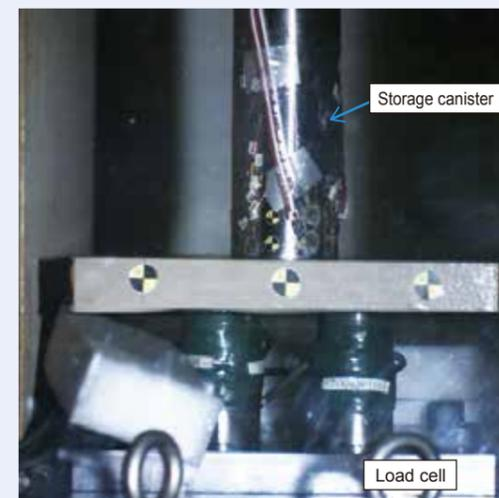
Fig. 3: Example of a storage canister drop test in the vertical direction
