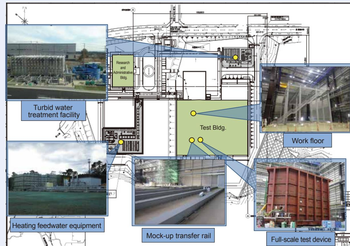
Fig. 1: Preparation of a test device facility
