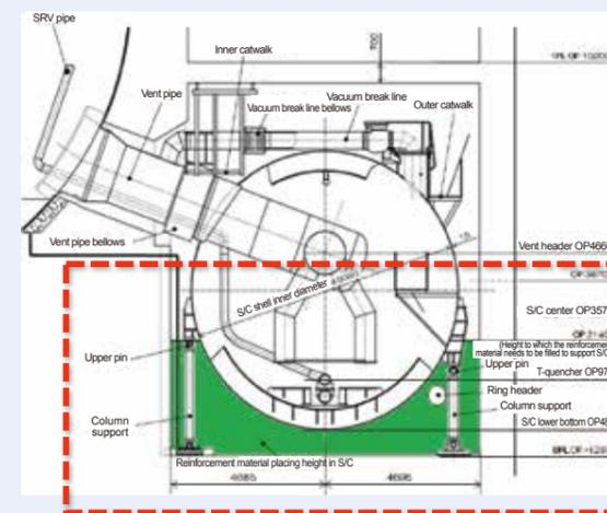
Fig. 1: Reinforcement material placing height in S/C (green area)
