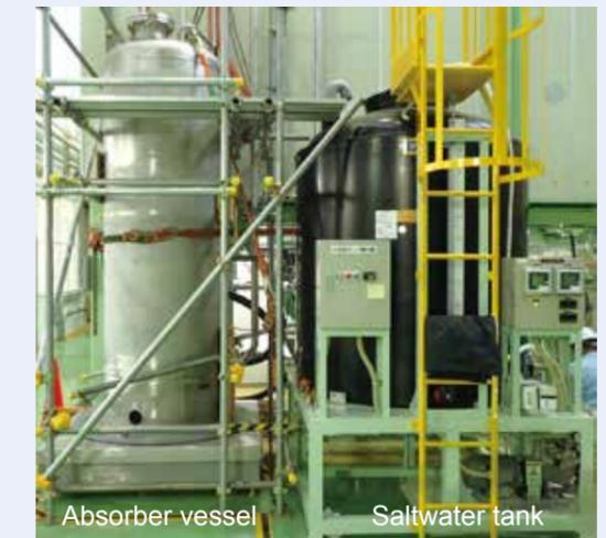
Fig. 3: Appearance of a full-scale absorber vessel to be used for various tests for absorbing, etc.
