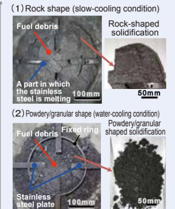
Fig. 4: Production of metal ceramics melt-solidification using UO<sub>2</sub> in the NNC, Kazakhstan.
