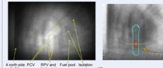
Fig. 4: Image of observation data (left fig.) and distribution of transmissivity (right fig.)
