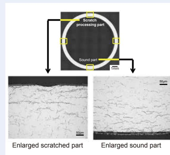
Fig. 1: Example of a verification test result for hydride precipitation behavior (Irradiated 9x9 fuel cladding, 300°C, cooling velocity 0.3°C/h, stress in a circumferential direction 70MPa, with scratches)
