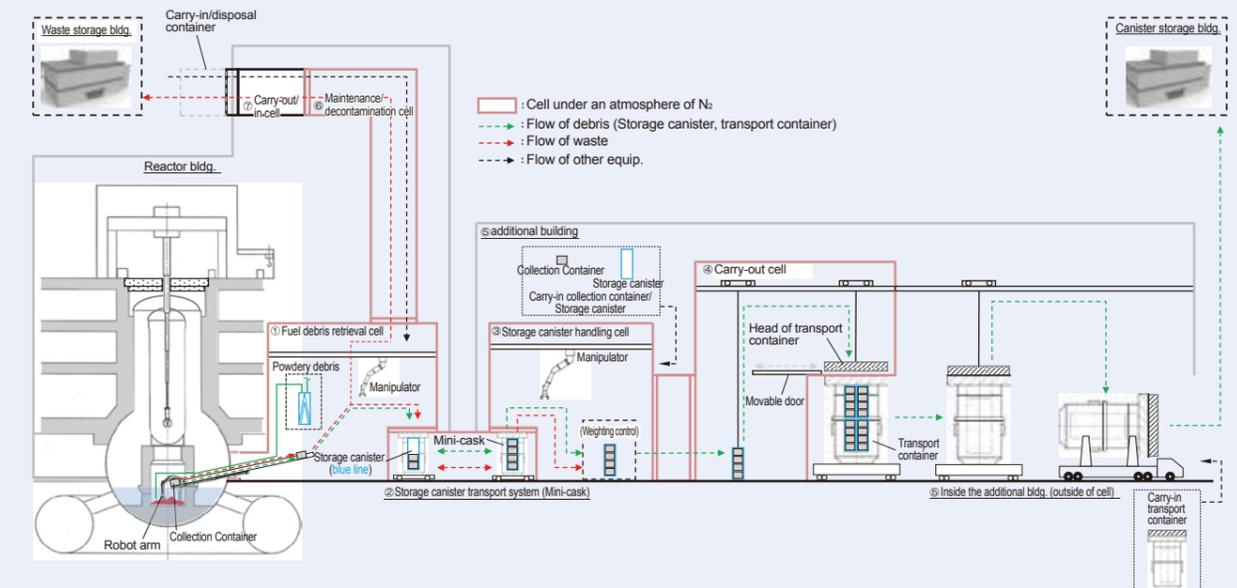
Fig. 2: Flow chart of fuel debris retrieval by Partial submersion-side entry method (Image)
