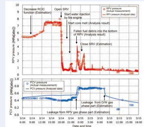
Fig. 2: Example of MAAP code accident progression analysis (Unit 2)
