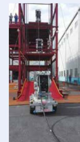
Fig. 4: Upper floor decontamination equipment (Elevating)
