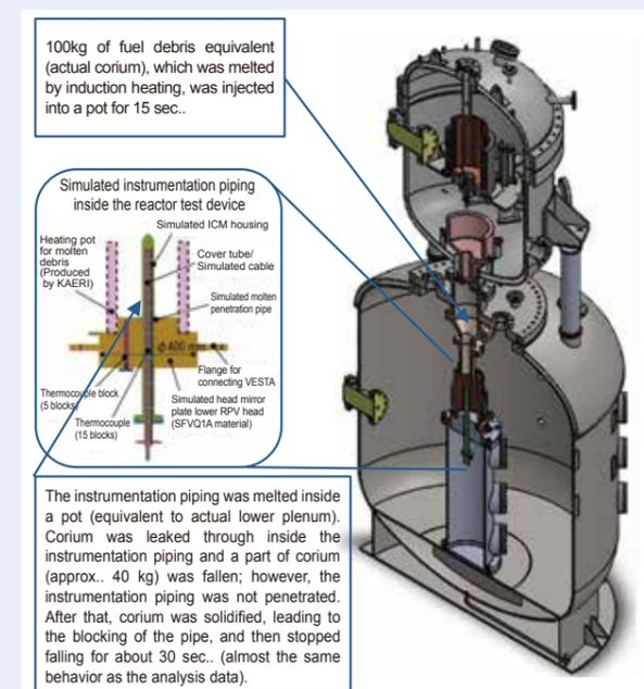
Fig. 4: PCV penetration pipe molten failure test (Simulated instrumentation piping inside the reactor test)
