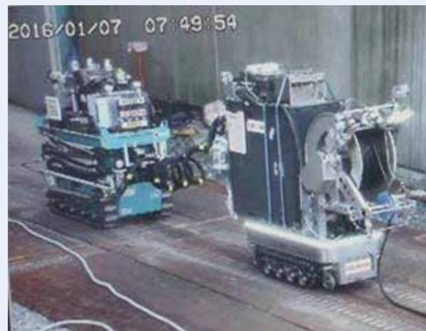
Photo 2: Scene of radiation dose rate measurement for high places (The decontamination equipment comprises two of the equipment for high places (left) and the equipment for low places (right)).
