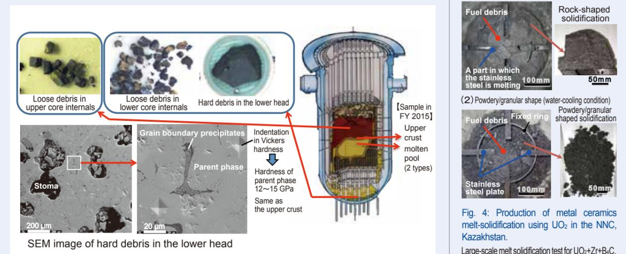
Fig. 3: SEM observation results of TMI-2 debris appearance/ cross-section
