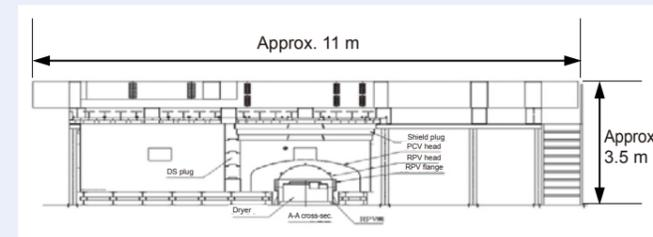
Fig. 1: Conceptual diagram of a plan for the scale model testing facility
