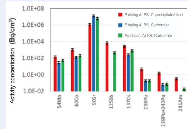
Fig. 1: Analysis data of radioactive waste (slurry) generated by ALPS operation
