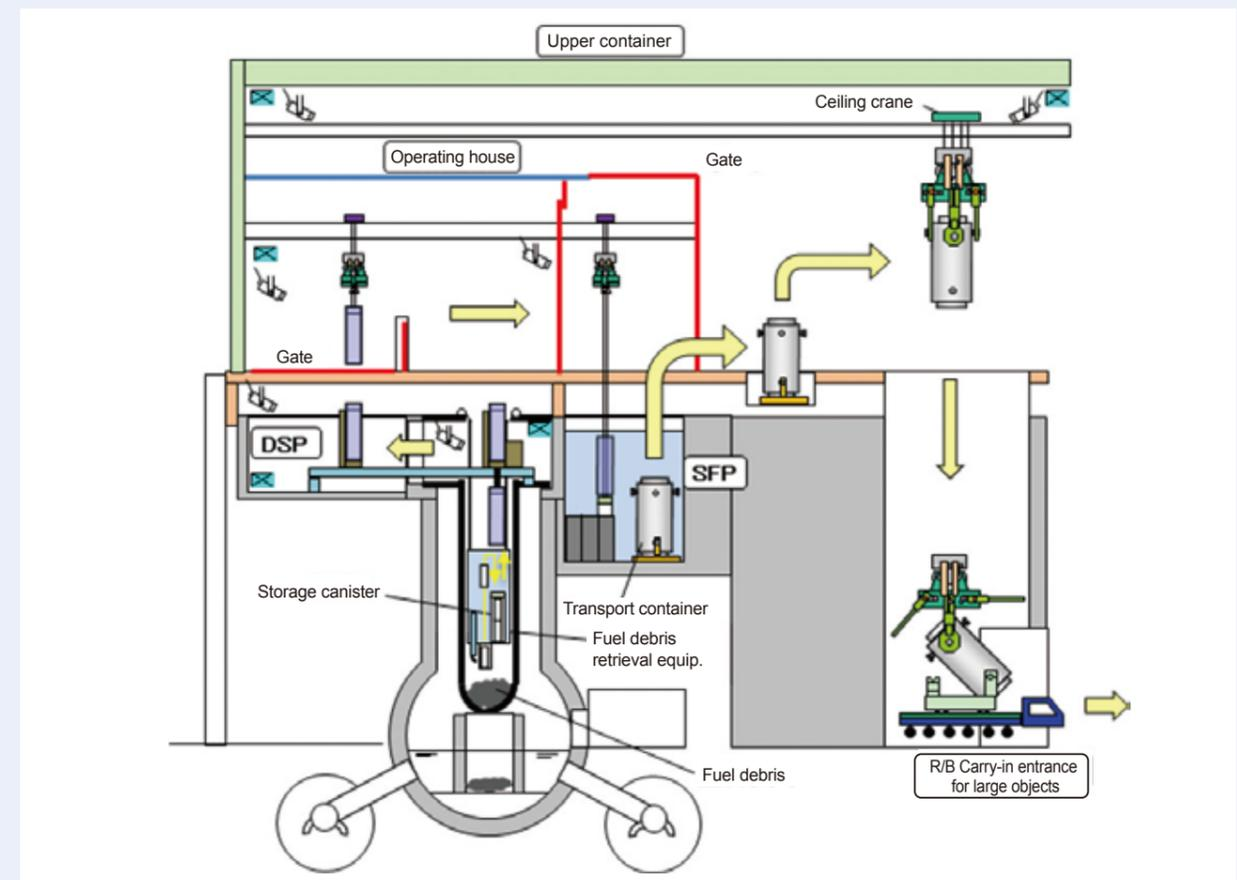
Fig. 1: Flow chart of fuel debris retrieval by Partial submersion-top entry method (Image)
