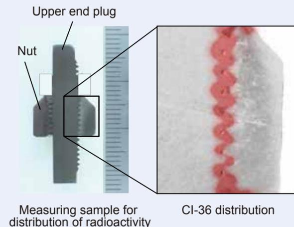
Fig. 3: Distribution of Cl-36 in upper end plug crevice structure (80°C, 2x dilution of artificial seawater after 50 hrs. of immersion)
