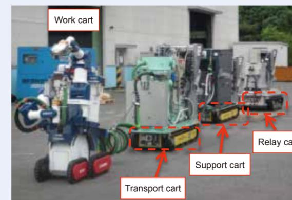
Fig. 3: Upper floor decontamination equipment (Showing mounted suction/blast equipment)
