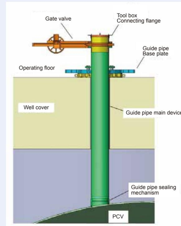
Fig. 1: Image of boundary function maintaining device
