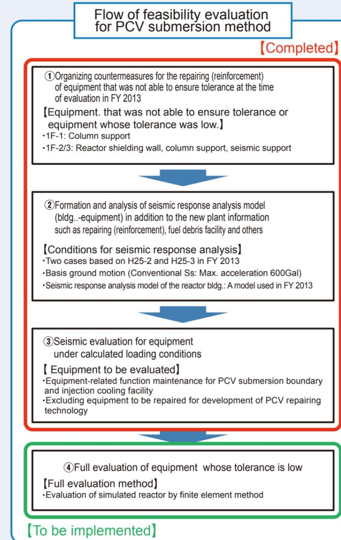
Fig. 1: Flow of PCV submersion method feasibility evaluation
