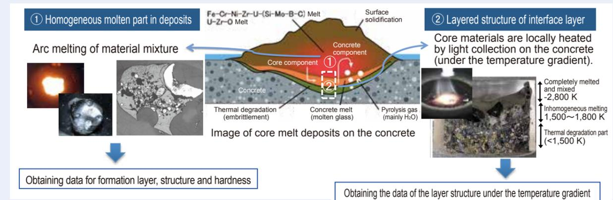
Fig. 2: Production method for two kinds of simulated MCCI products according to the test purpose
