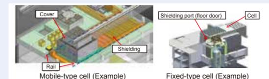
Fig. 8: Mobile-type/fixed-type cell (Image)
