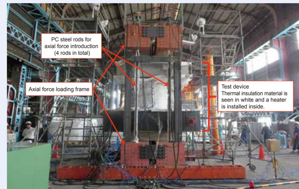
Fig. 3: Proof stress evaluation test of the RPV pedestal (Installation loading frame)
