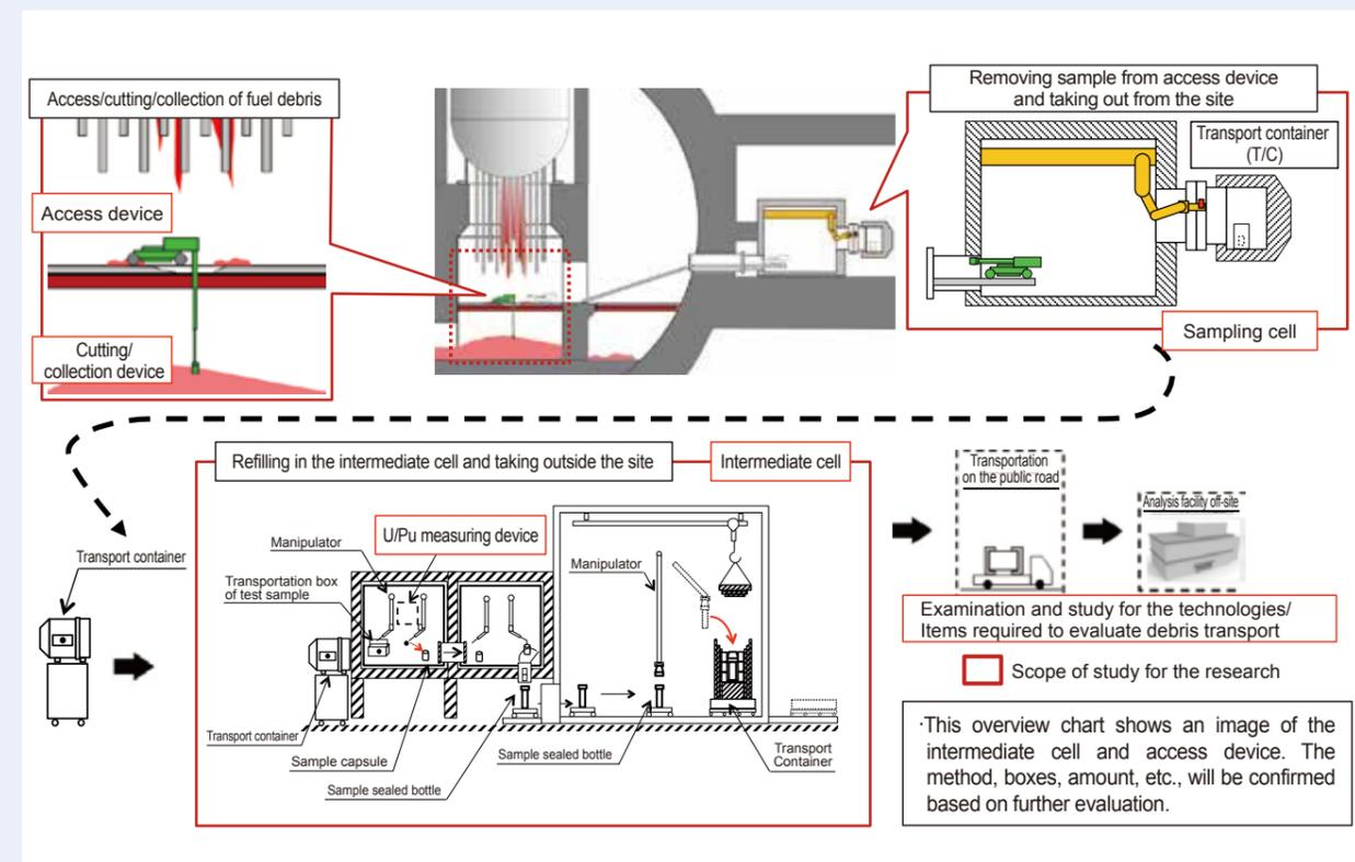
Fig. 3: Flow chart of the whole process from fuel debris sampling to analysis (Image)
