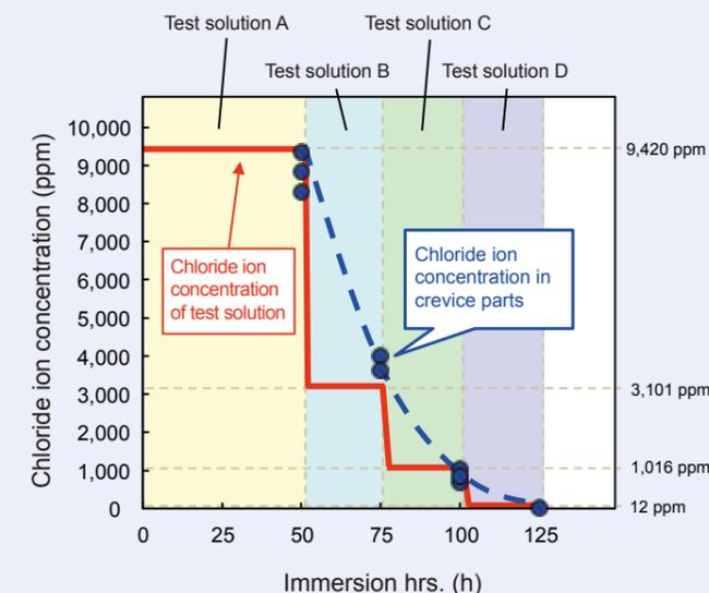
Fig. 4: Evaluation result of chloride ion concentration in the upper end plug crevice structure
