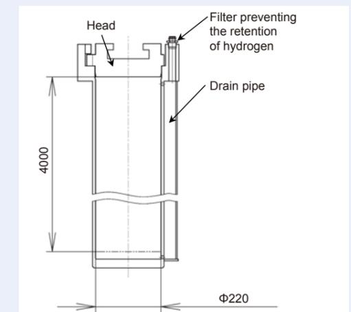
Fig. 4: Basic design of a storage canister (Example)
