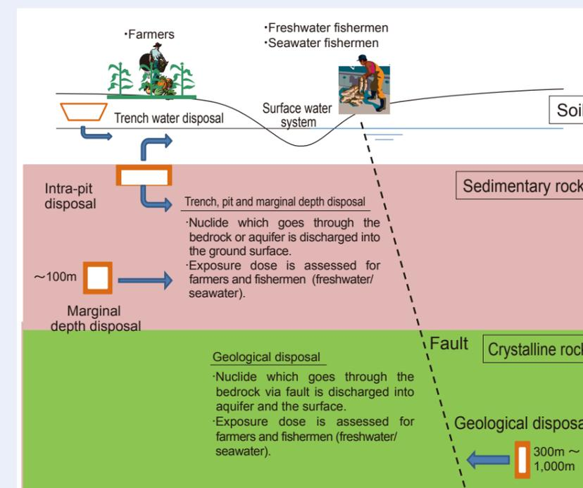
Fig. 4: Conceptual model for a transition of the groundwater
