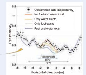
Fig. 5: Comparison with simulated transmissivity measurement
