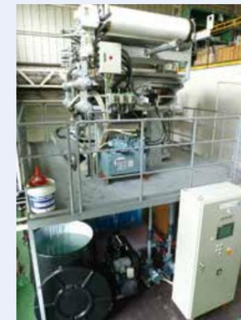
Fig. 2: Pressure filtering test device to examine the dehydration treatment for the slurry from ALPS
