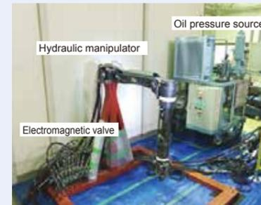
Fig. 3: Photo of test device for hydraulic manipulator
