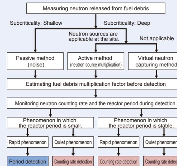
Fig. 2: Detection process of criticality approach detection system inside the reactor core
