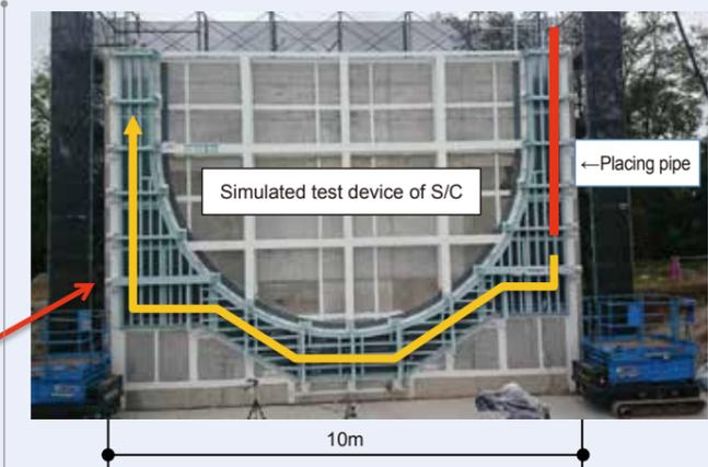
Fig. 2: Verification test for evenly balanced flow behavior of strengthening S/C support column (1/1 scale: simulated Unit 2,3)
