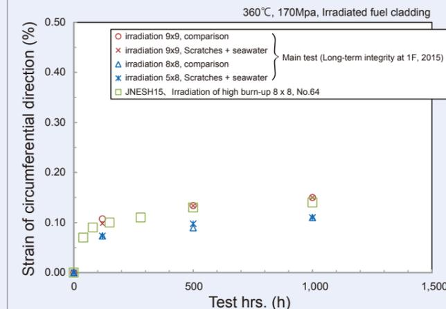
Fig. 2: Example of a study result (attached scratches + seawater) that can affect the creep speed
