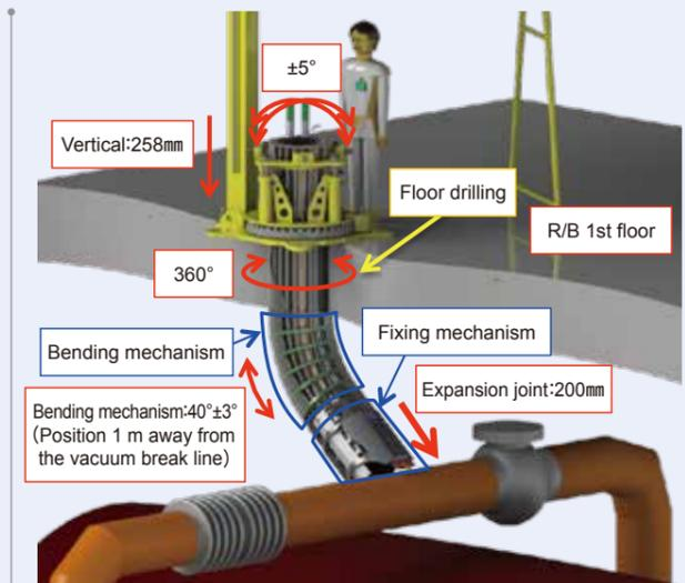
Fig. 4: Flexible guide pipe overview
