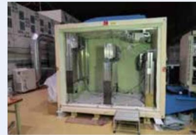
Fig. 1: Detection system for the transmission method used for measurement in Unit 1
