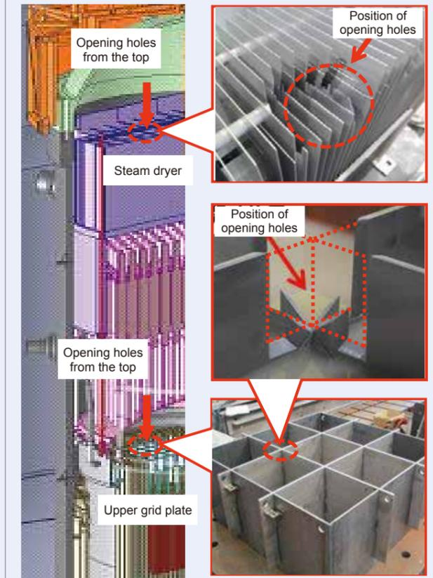
Fig. 2: Elemental analysis for opening holes using partial simulated test device of the reactor internals
