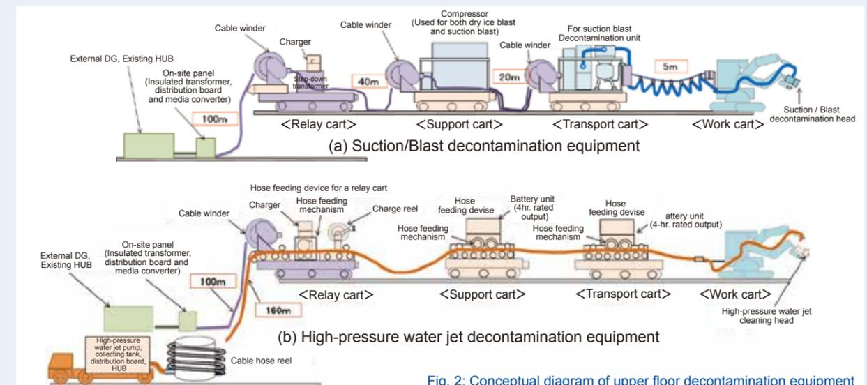
Fig. 2: Conceptual diagram of upper floor decontamination equipment
