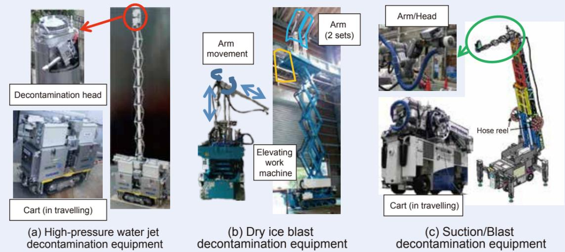
Fig. 1: Decontamination equipment for high places
