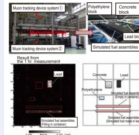
Fig. 6: Measurement results of the transmission method by the developed system
