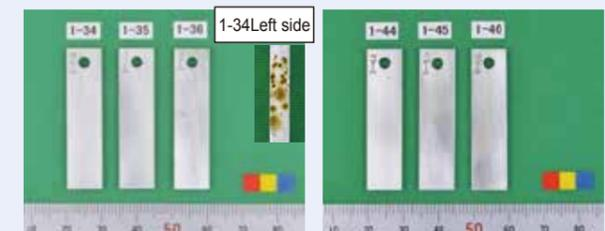
Fig. 3: Soluble neutron absorption material low concentration corrosion test result (example)
