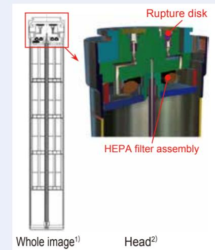
Fig. 2: Storage canister used at Hanford Site in U.S. (Ref.)
