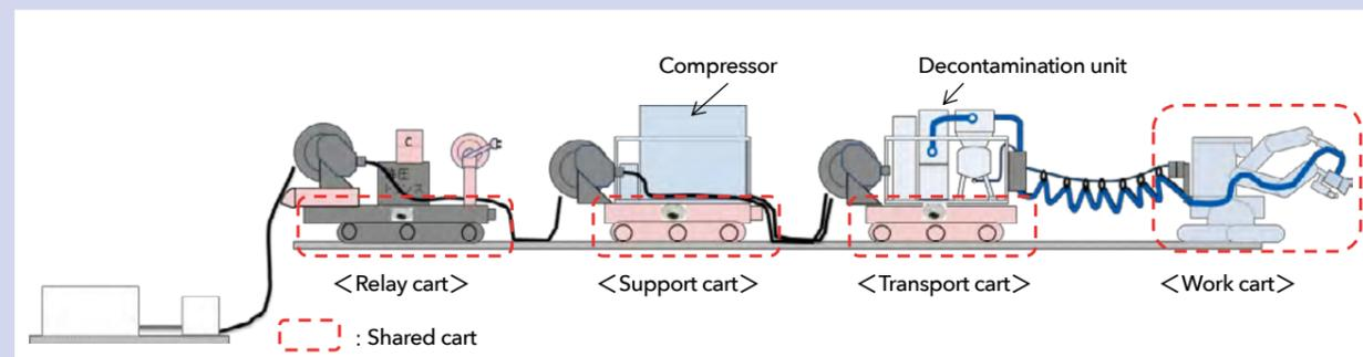
Figure 4 Conceptual diagram of upper floor decontamination equipment (shows mounted blast equipment as an example).
