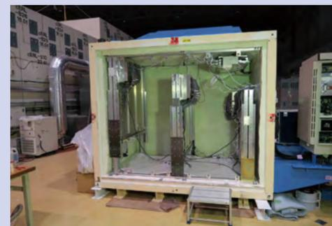
Figure 1 Muon detector which uses transmission method to be installed at the Fukushima Daiichi NPS Unit 1
