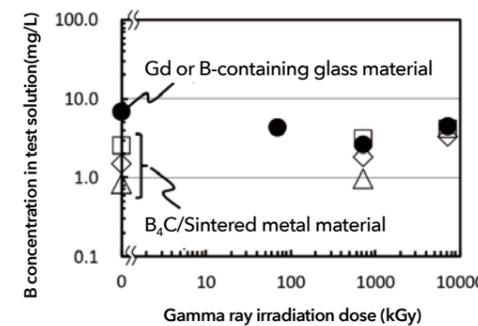
Figure 2 Non-soluble neutron absorption material dissolution test result (example)
