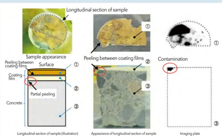
Figure 1 Imaging plate measurement results of contamination sample (Unit 2 operation floor: Floor of upper part of well)
