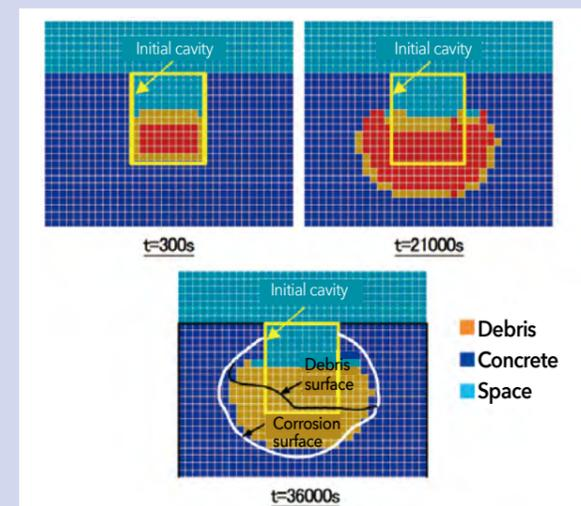
Figure 3 Pit erosion behavior evaluation example
