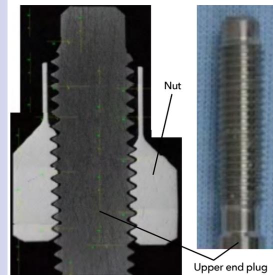
Figure 1 Results of cross-sectional (left) and external (right) observation of fuel assembly upper section test specimen (The test specimen was immersed for 1,000 hours at a temperature 90°C and a chloride ion concentration of 2,500ppm. After that, it was further immersed for 7,409 hours at a temperature 60°C and chloride ion concentration of 100ppm.)
