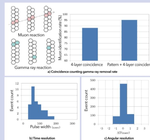
Figure 5 Results of circuit system performance evaluation
