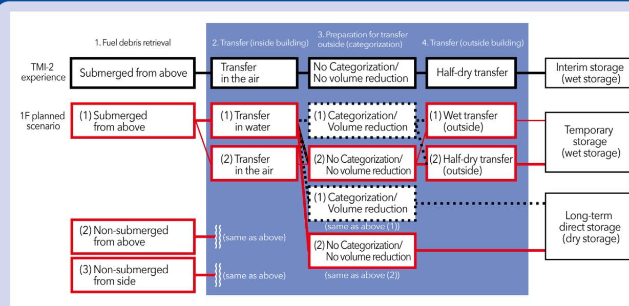
Figure 1 Scenario for collection, transfer, and storage of retrieved fuel debris (partial)
