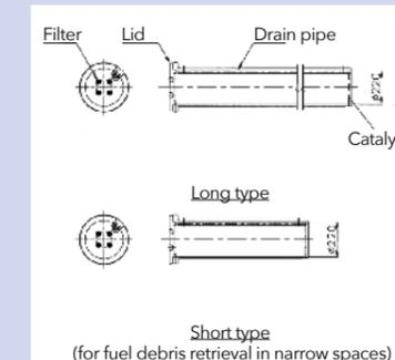
Figure 2 Storage canister basic concept (example)
