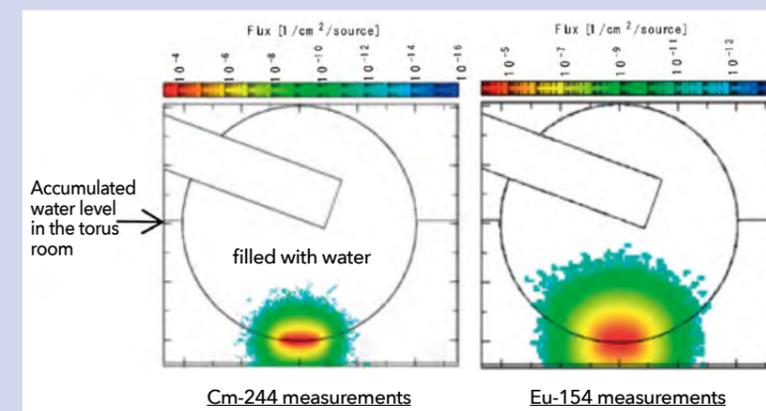
Figure 2 Distribution of radiation originating from fuel in the vicinity of the S/C (Unit 1)
