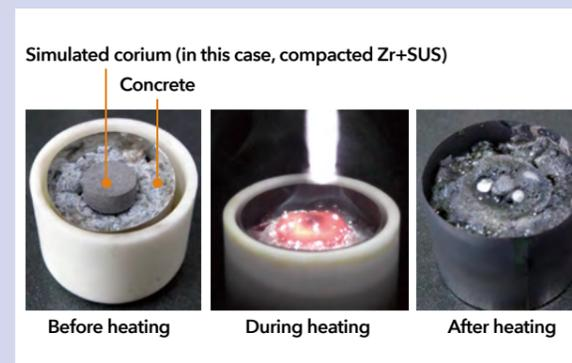
Figure 1 State of simulated MCCI products manufactured through light condensing and heating
