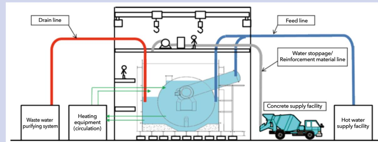
Figure 1 Conceptual design of the full-scale test facility
