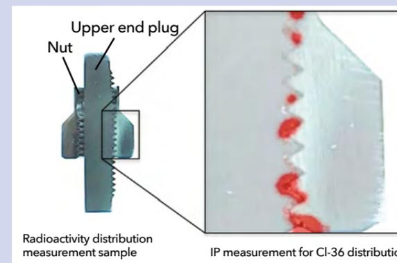
Figure 3 Distribution of Cl-36 in upper end plug screw structure (80°C, two-fold dilution of artificial seawater, after 50 hours immersion)
