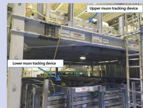
Figure 4 Muon tracking device system performance test platform
