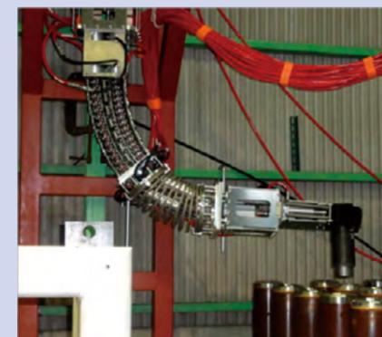
Figure 3 Handling test on remotely operated working arm (artificial muscle robot)
