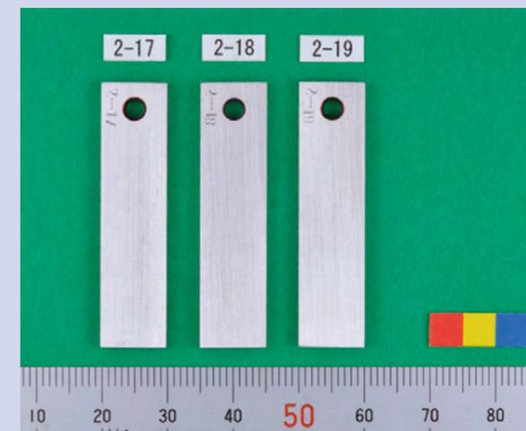
Figure 3 Soluble neutron absorption material corrosion test result (example)
