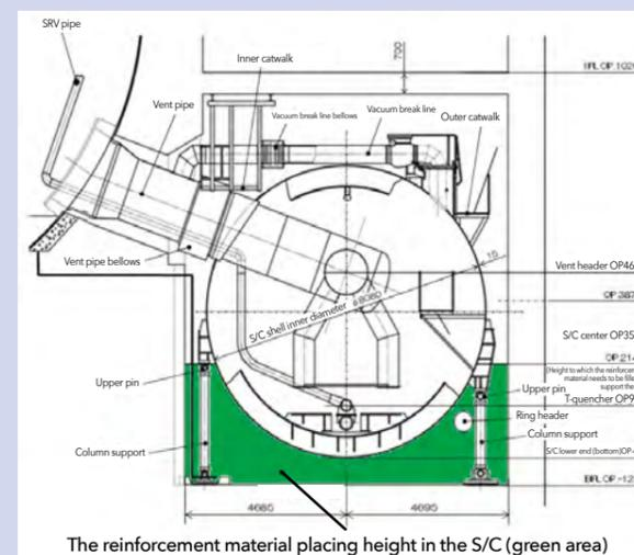
Figure 1 The studied reinforcement material placing height in the suppression chamber (S/C)
