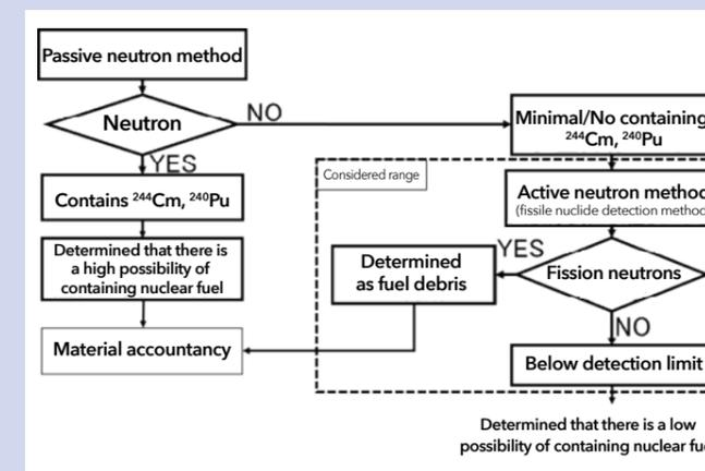
Figure 5 Proposed sorting method related to the presence or absence of nuclear material
