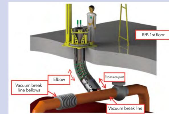
Figure 4 Flexible guide pipe overview
