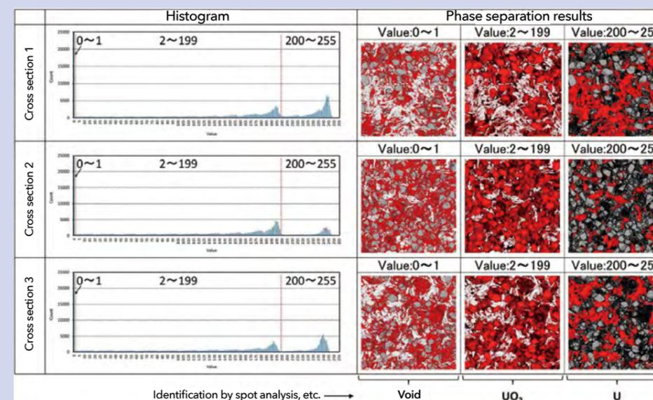
Figure 3 Results of phase analysis using backscattered electron images and gradation distribution taken by SEM/WDX
