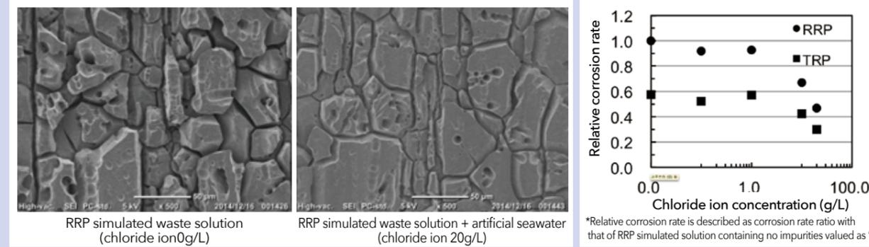
(1) Surface observations of immersion test piece
