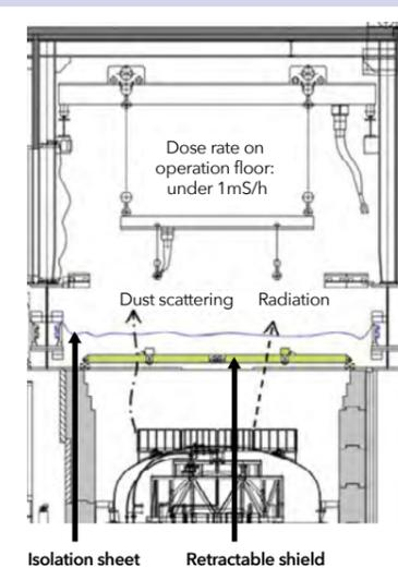
Figure 2 Use of isolation sheet for preventing the spread of contamination
