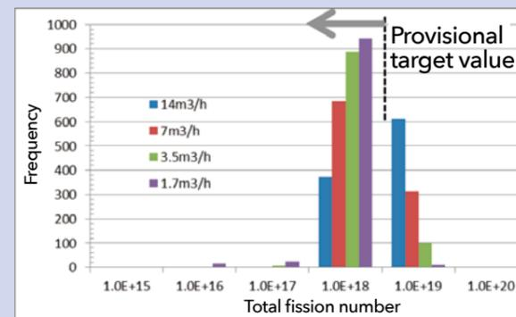
Figure 1 Evaluation of total fission number on the assumption of a criticality accident occurring at the time of PCV submersion
