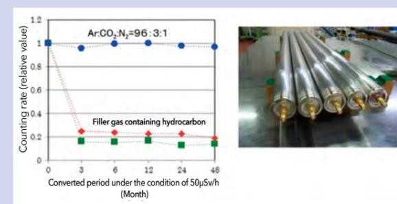
Figure 3 Production of highly radiation-resistant drift tube detectors.
