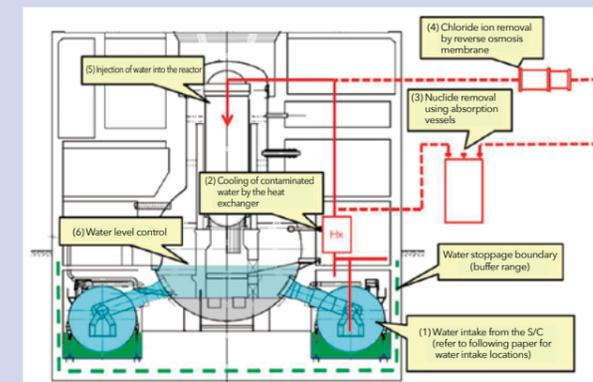
Figure 2 Concept of the PCV circulation cooling system
