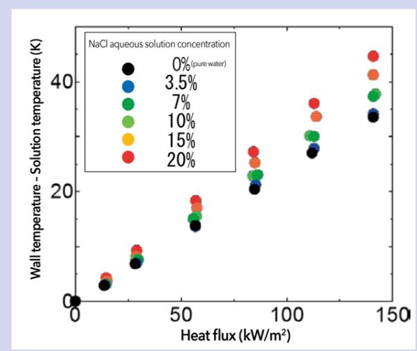
Figure 4 Example of test results using sodium chloride solution (Temperature difference between wall and solution)
