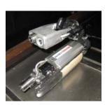
Robot for Measurement of S/C Water Level
