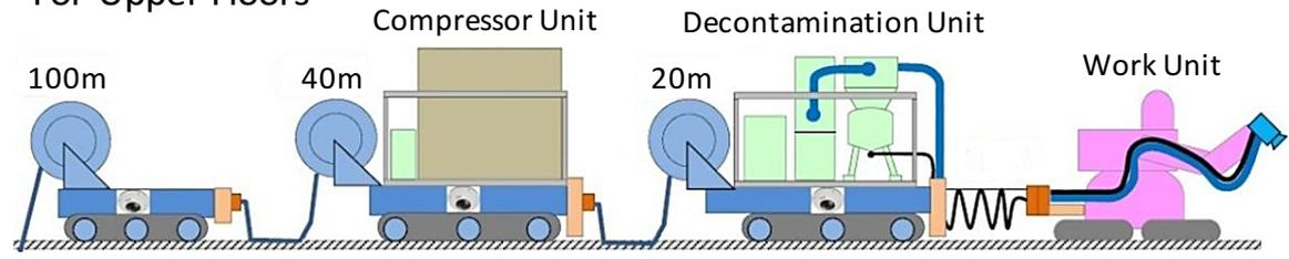
Each unit is lifted up to the upper floor with the Lifter in continuity
