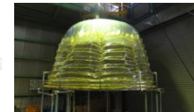
Sealing a PCV head (1:4 scale) with Radioactive material diffusion preventing film
