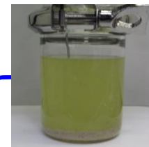
【Nitric acid solution of seawater and concrete】
