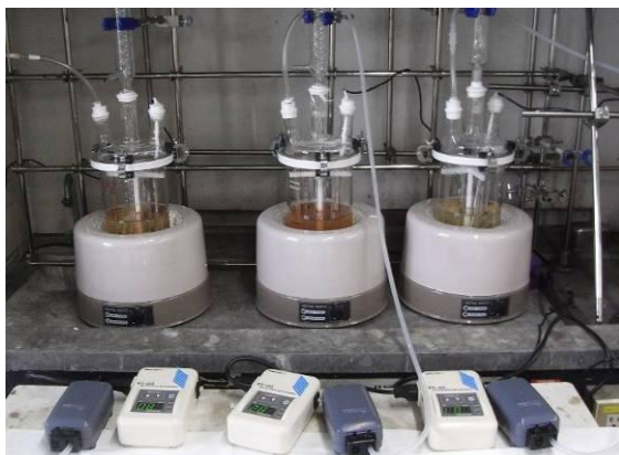
Corrosion testing status and example of the results (carbon steel / low alloy steel)
